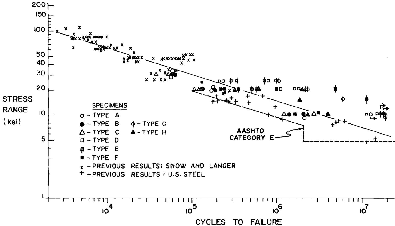
Fig. 18 Comparison of Axial Loaded Single Nut Fatigue Data With Category E Fatigue Stress Level
