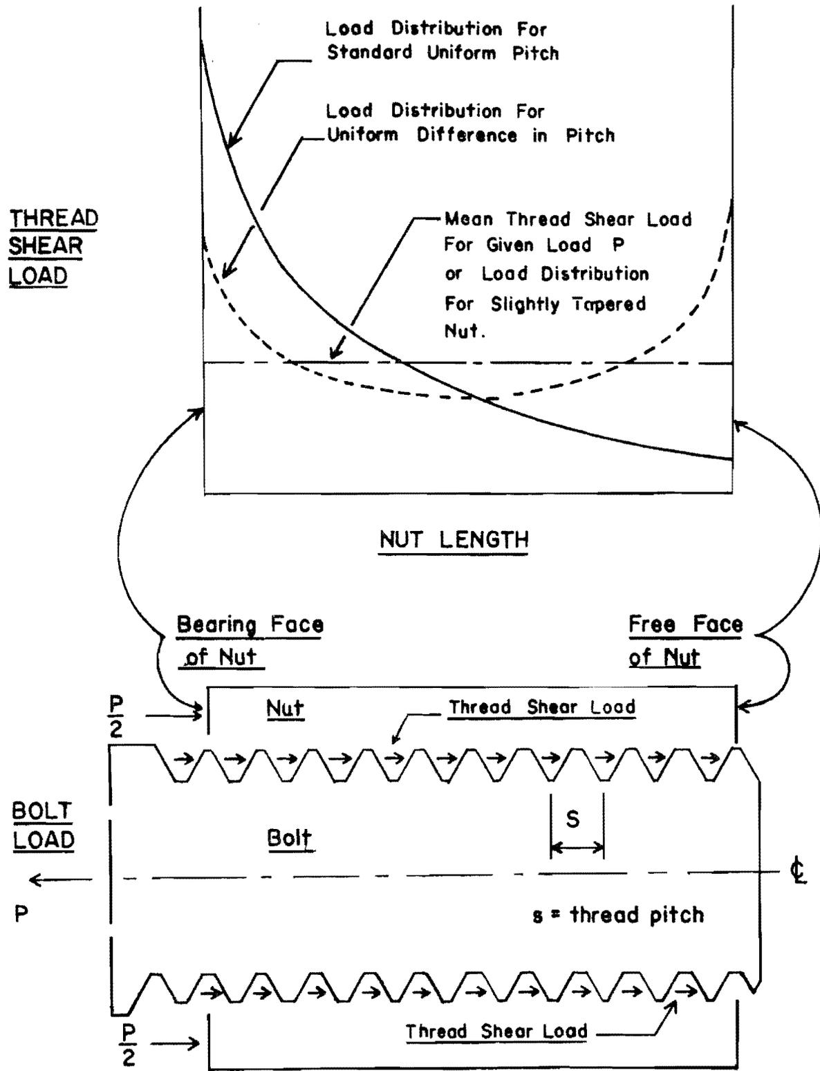
Fig. 11 Thread Shear Load Distribution in Single Nut Connection
