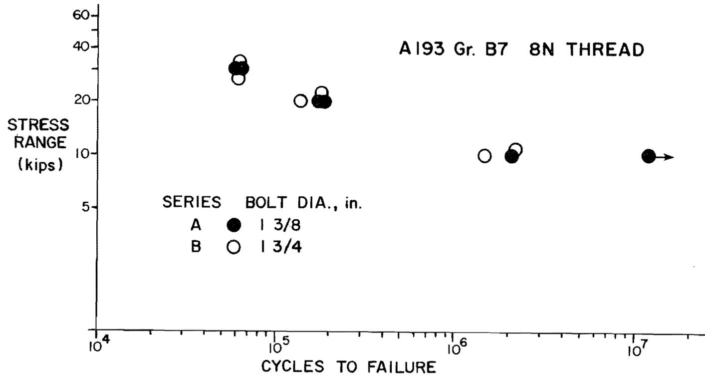
Fig. 14 Effect of Bolt Diameter on Axial Fatigue Strength
