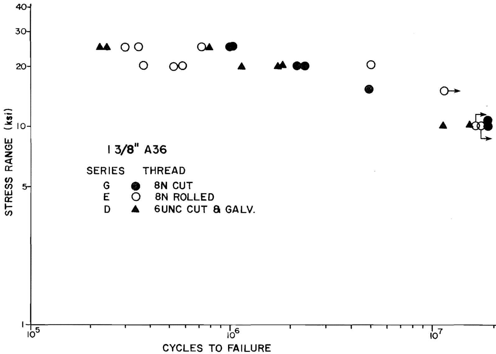
Fig. 15 Effect of Thread Forming on Axial Fatigue Strength
