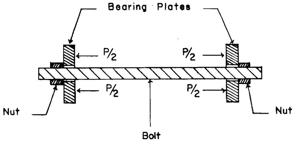
Fig. 2. Specimen Loading Geometry.
