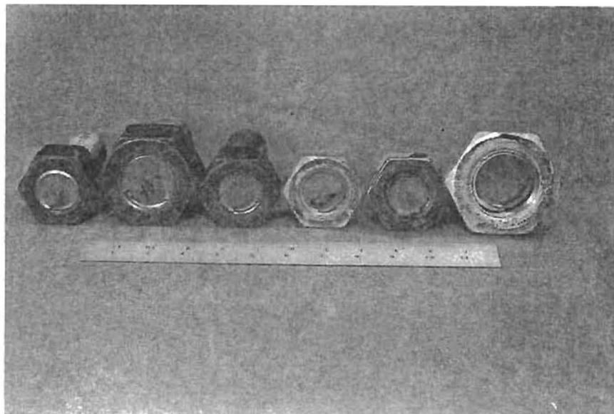
Fig. 10 Characteristic Failure Surfaces (Left to Right: Series A, B, C, D, E, and F)
