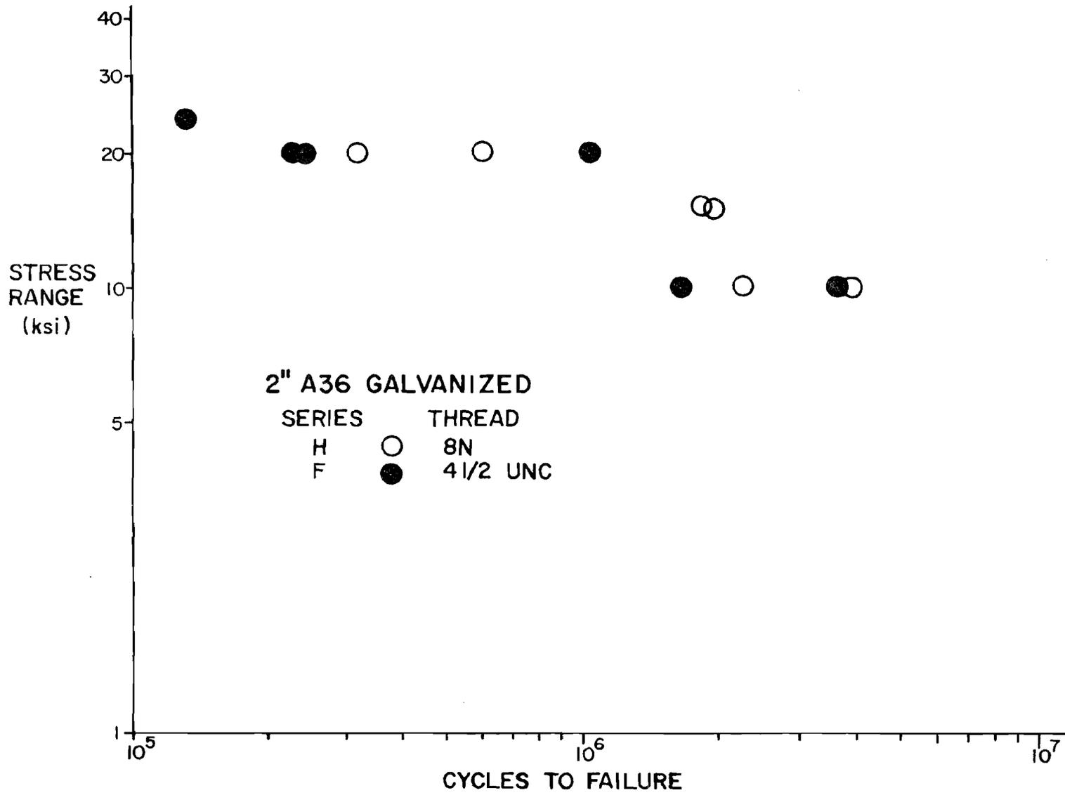
Fig. 13 Effect of Thread Pitch on Axial Fatigue Strength
