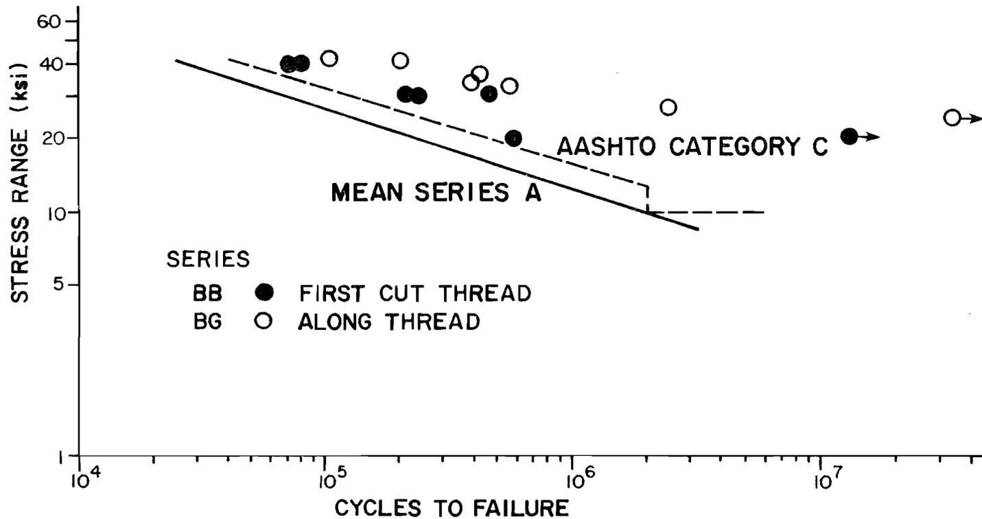
Fig. 17 Bending Fatigue Data
