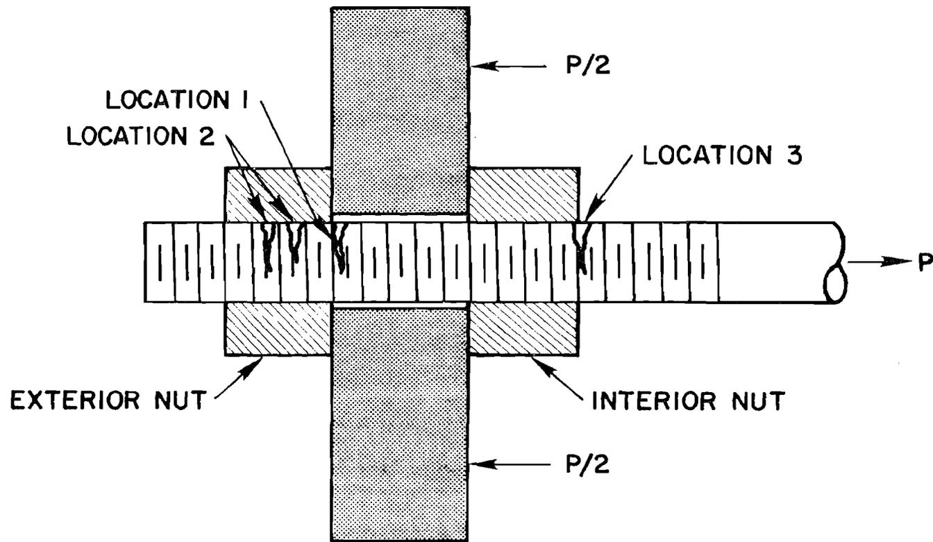
Fig. 8 Fatigue Failure Locations
