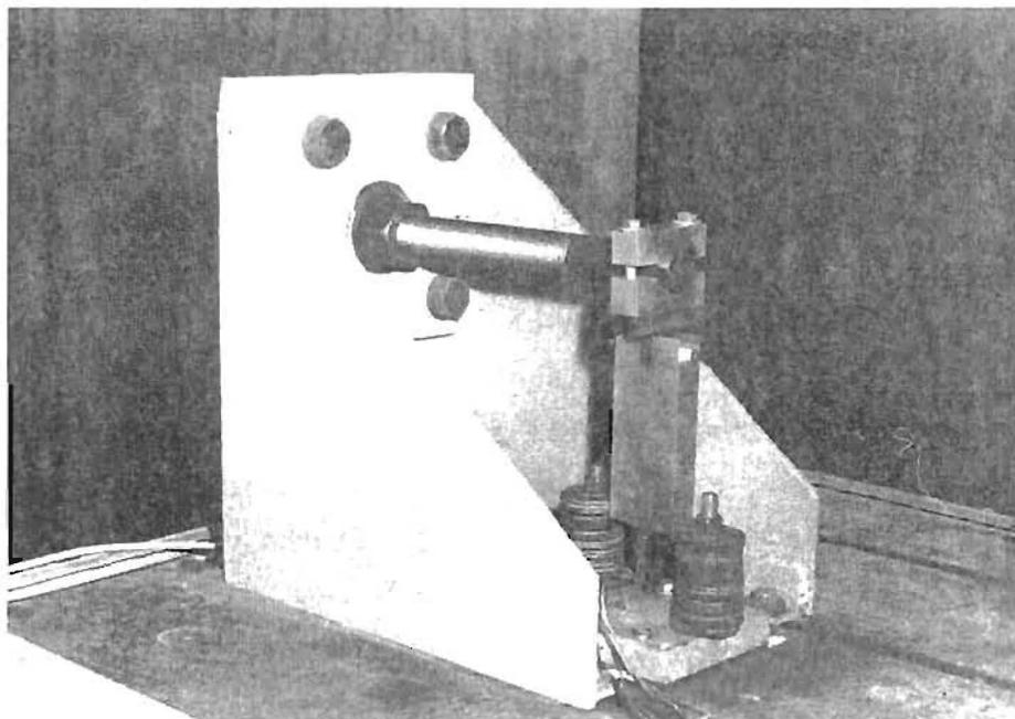
Fig. 5 Bending Fatigue Test Setup
