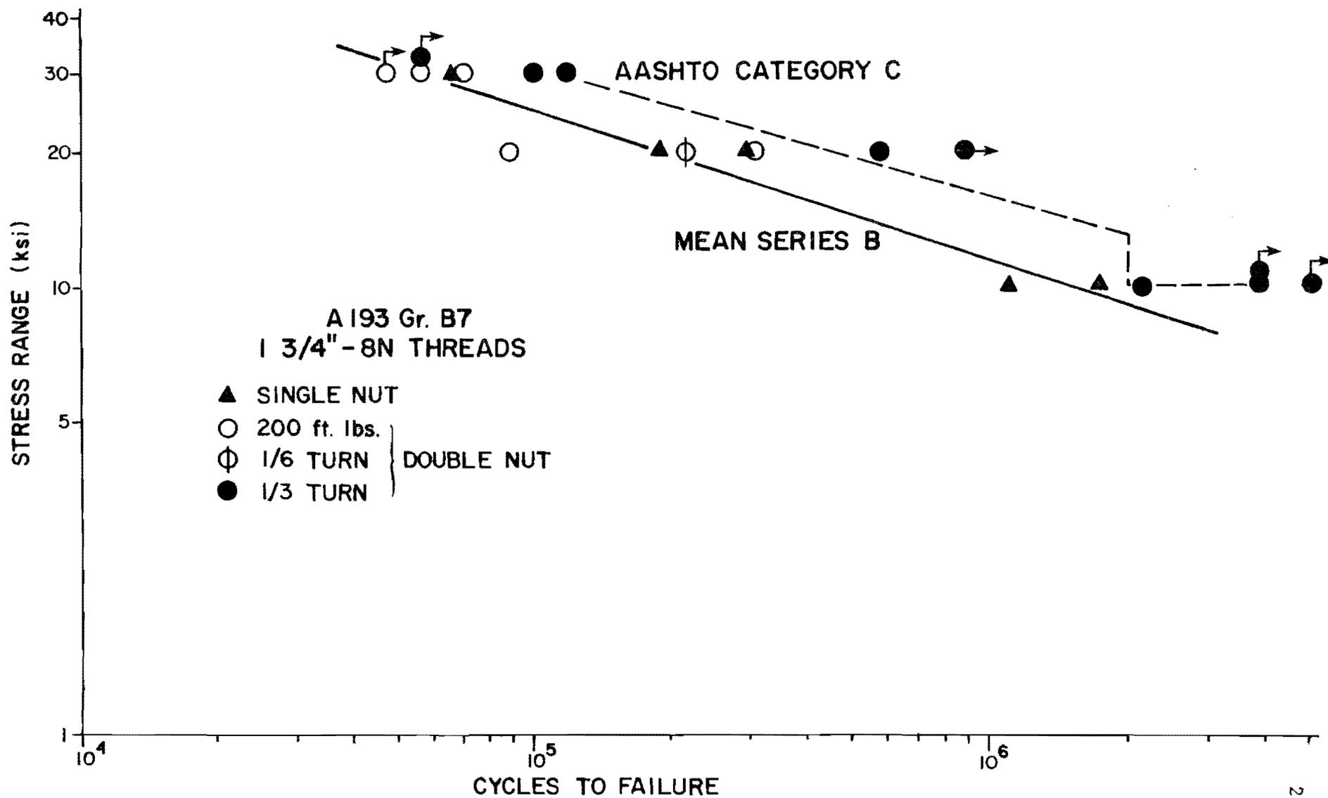
Fig. 16 Double Nut Axial Fatigue Data
