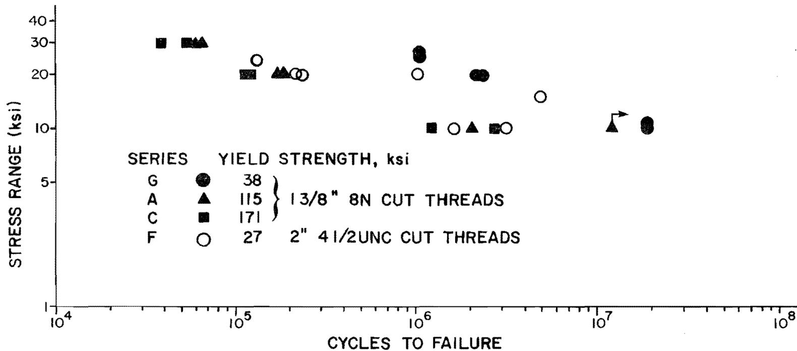
Fig. 12 Effect of Steel Strength on Axial Fatigue Strength
