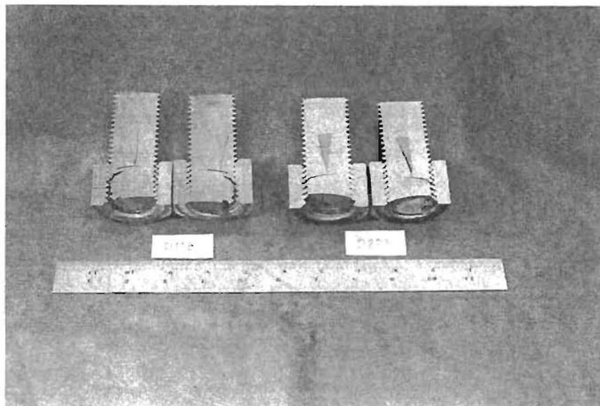
Fig. 9 Cross Section Showing Multiple Cracking
