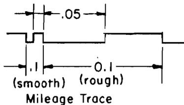
(1) **Distance** (top trace), is controlled by a special odometer, zigs for 0.05 and zags for 0.05 miles; one complete cycle = 0.10 miles. The distance the vehicle traveled is recorded independently of chart feed.
