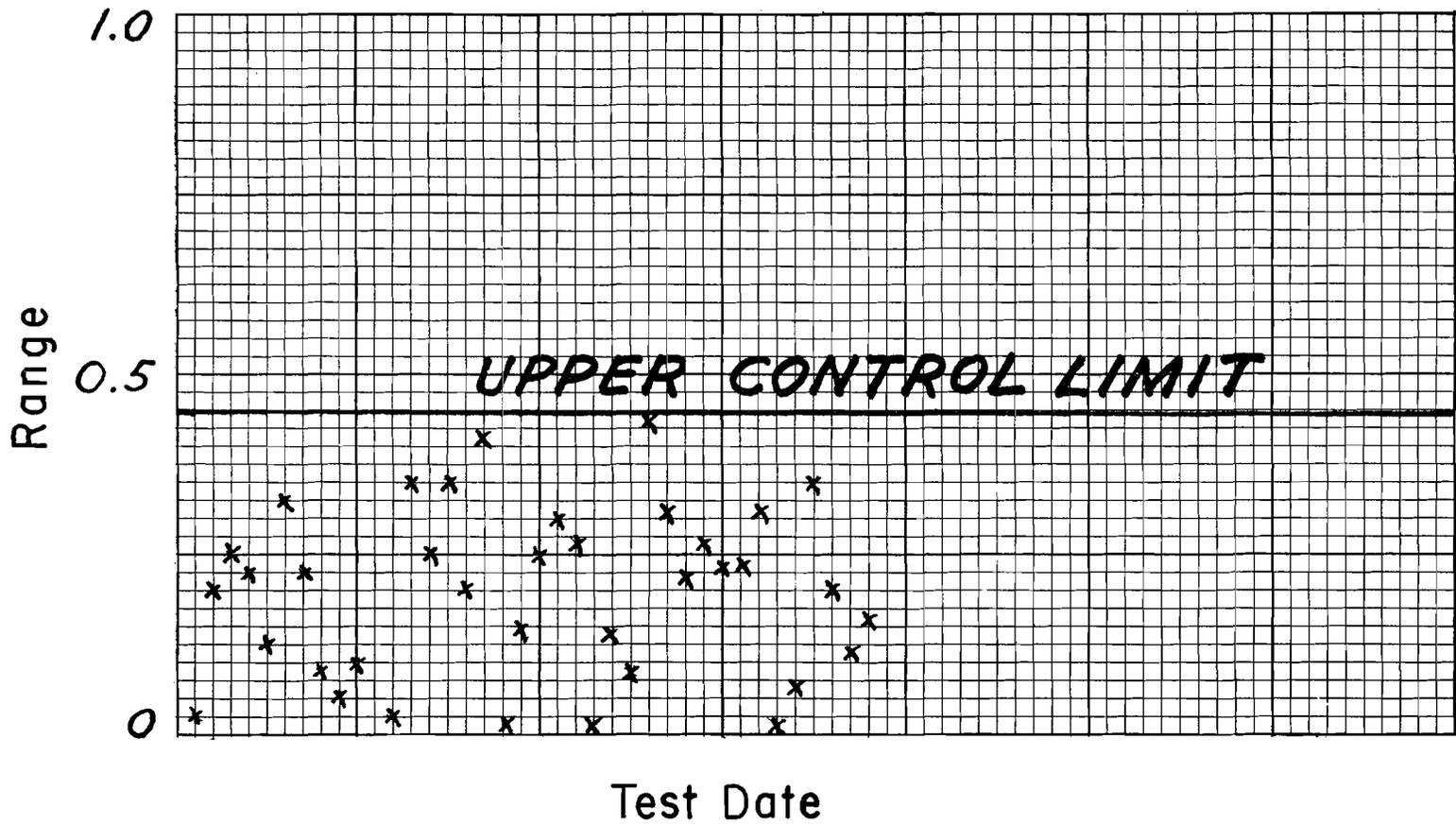
Fig D. Typical MRM control chart for range.
