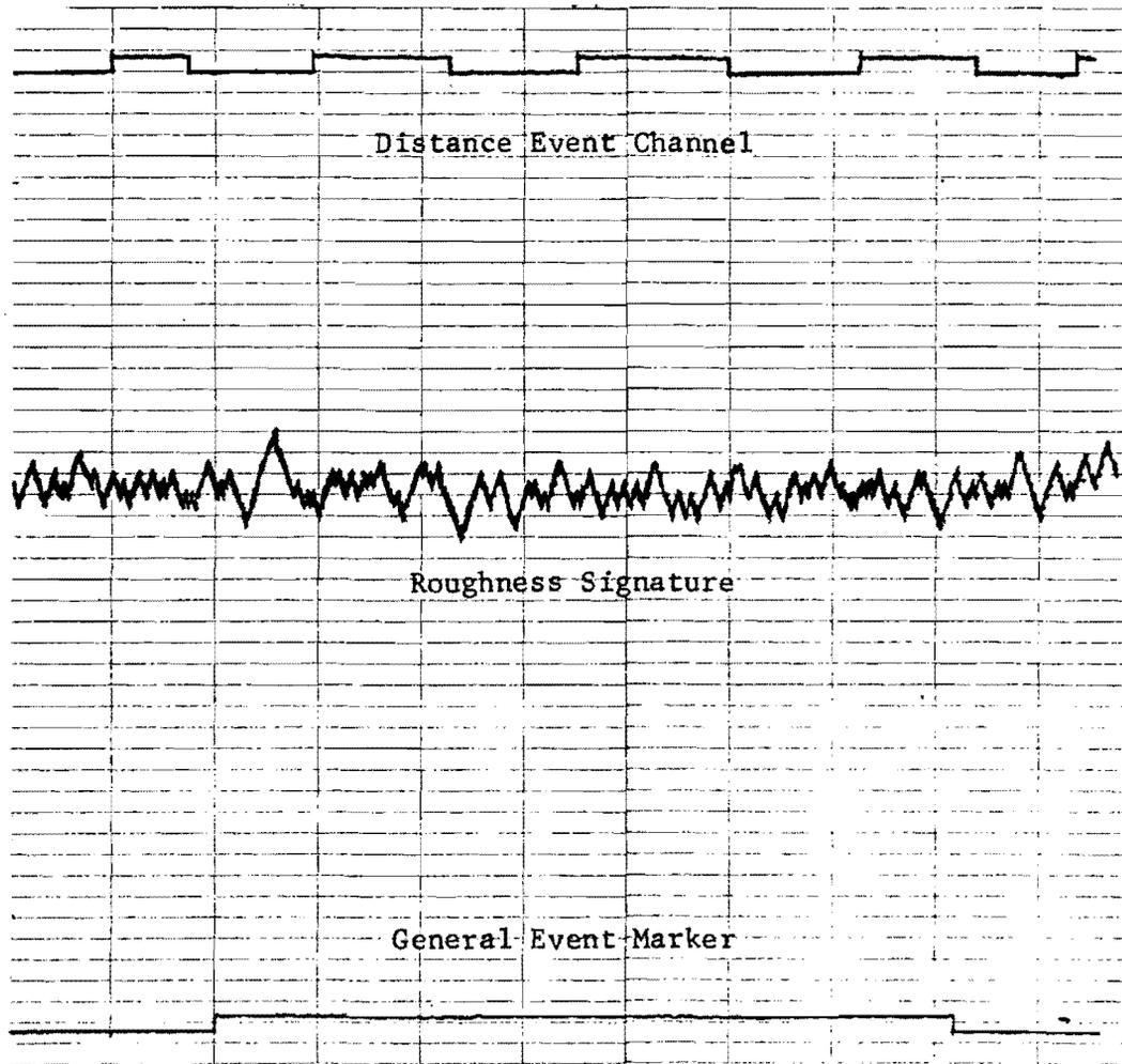
Fig 2.1. Typical Rainhart MRM measurement record.
