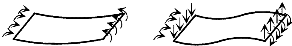
Figure 2.2. Out-of-Plane Deformations of Plates
