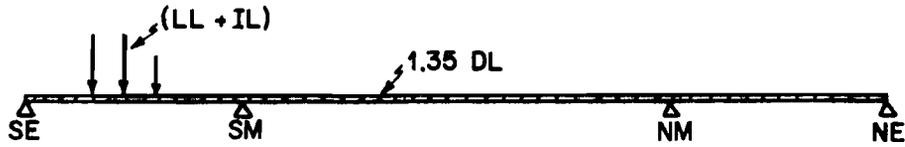
(C) ULTIMATE LOADING CONFIGURATION FOR MAXIMUM SHEAR ADJACENT TO NM IN THE MAIN SPAN.
