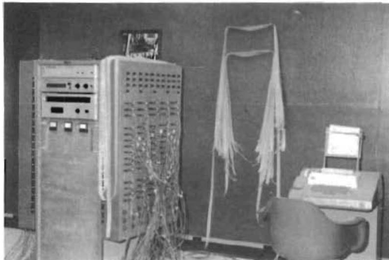
Fig. 5.2. VIDAR system and teletype
