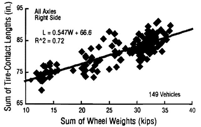
**Fig 6.14. Sum of tire-contact lengths versus sum of weights for all axles.**
