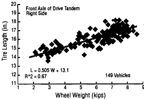
Fig 6.8. Tire-contact length versus weight for front axle of drive tandem.
