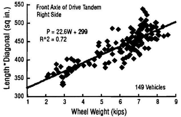
Fig 6.10. Product of tire-contact length and projected diagonal dimension versus weight for front axle of drive tandem.
