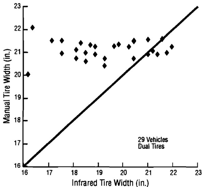
Fig 6.3. Comparison of tire-contact widths.
