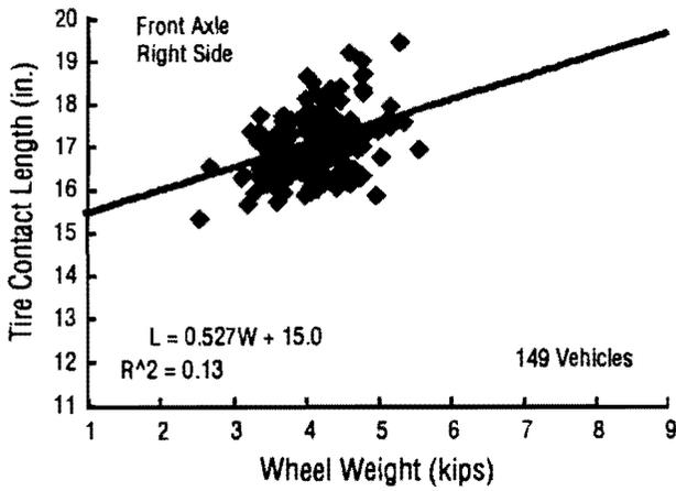
Fig 6.6. Tire-contact length versus weight for front axle.
