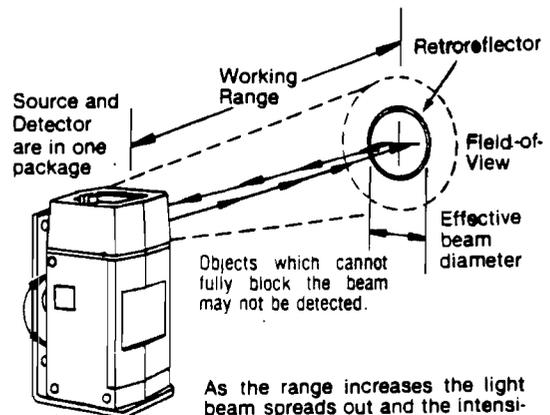
As the range increases the light beam spreads out and the intensity per unit area is reduced because the same amount of light must cover a much greater area.
