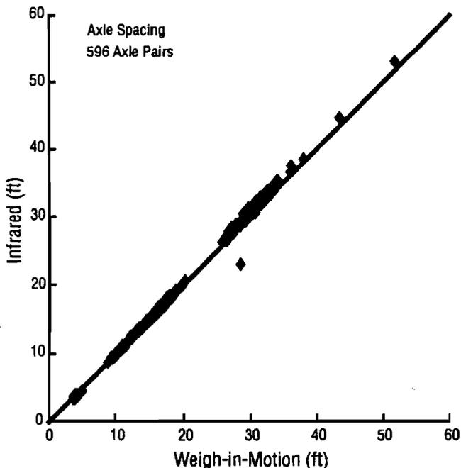
Fig 6.5. Comparison of axle spacing.
