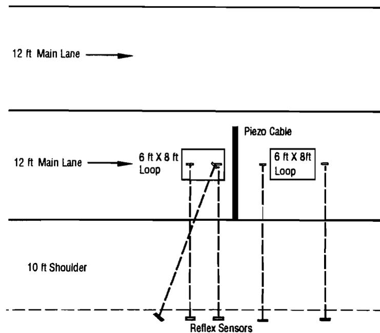
Fig 6.16. Sensor arrangement at Jarrell.
