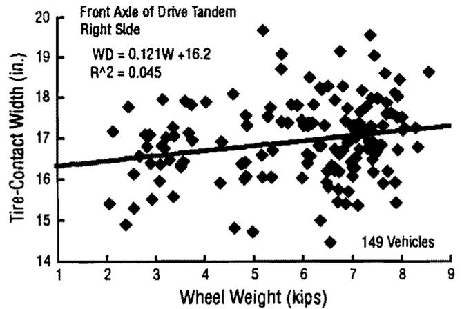
Fig 6.11. Tire-contact width versus weight for front axle of drive tandem.
