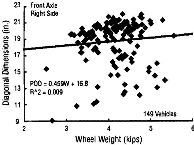
Fig 6.7. Projected diagonal dimension of tire-contact areas versus weight for front axle.
