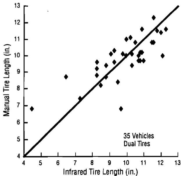
Fig 6.2. Comparison of tire-contact lengths.
