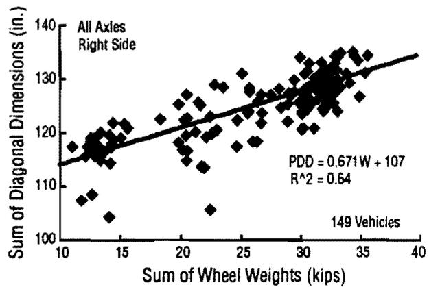
**Fig 6.15. Sum of projected diagonal dimensions of tire-contact areas versus sum of weights for all axles.**
