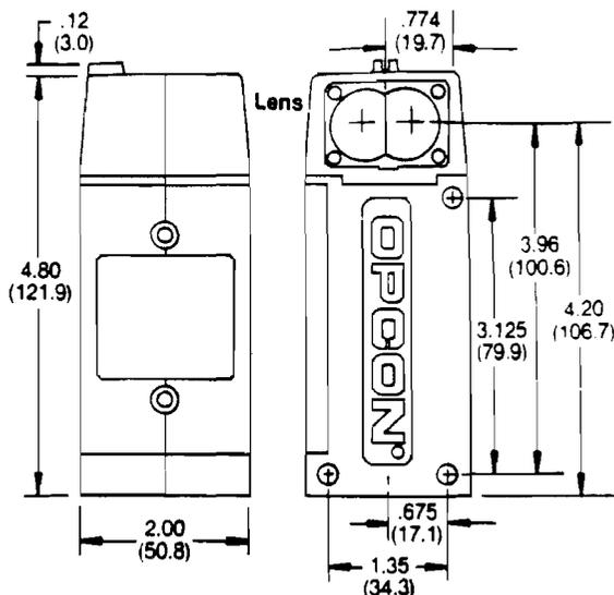
Reference Dimensions for Center of Lens.
