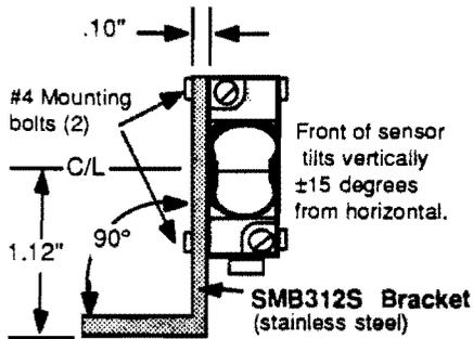
Bracket rotates horizontally ±10 degrees from position shown.
