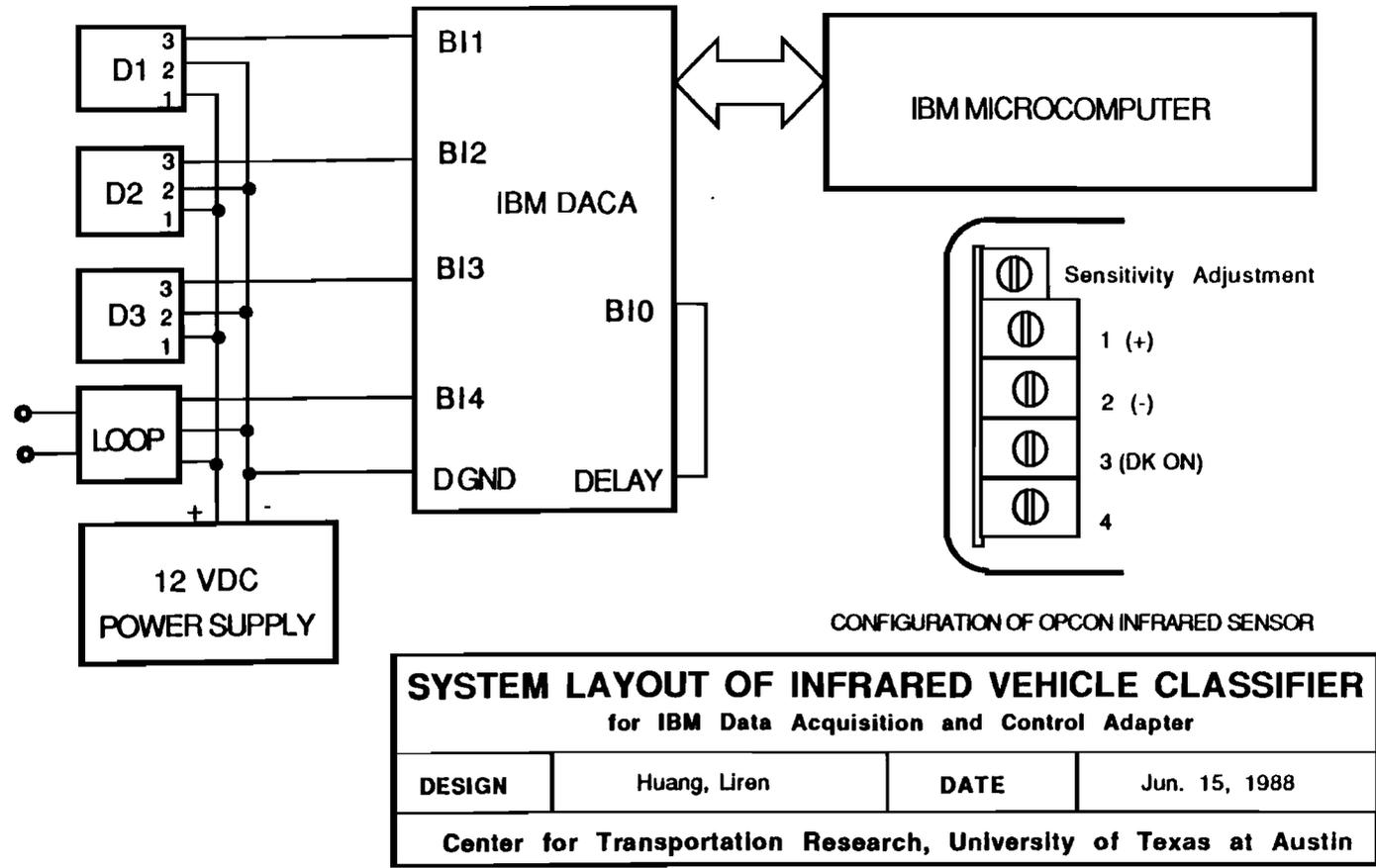
Fig A.8. System layout for three-sensor vehicle classification system.
