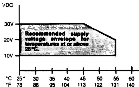
Note: Operation outside the recommended supply voltage envelope will result in erratic performance at high temperature.
