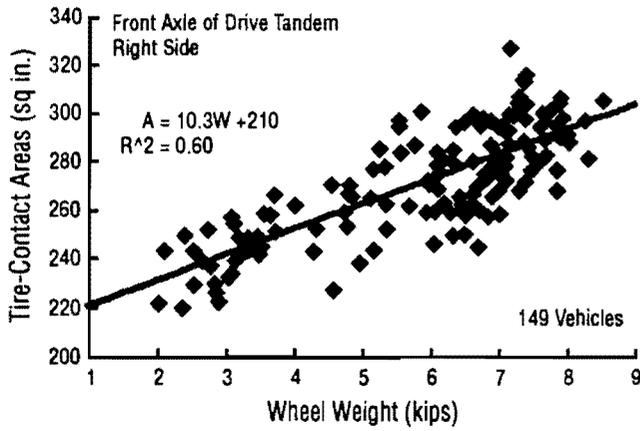
**Fig 6.12. Tire-contact area versus weight for front axle of drive tandem.**
