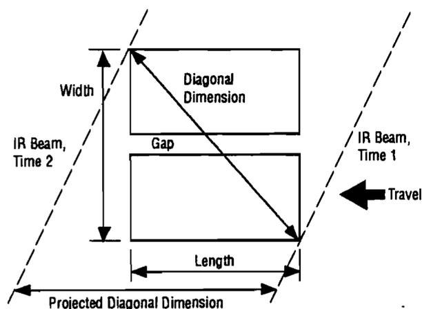
Fig 6.1. Tire-contact-area dimensions.
