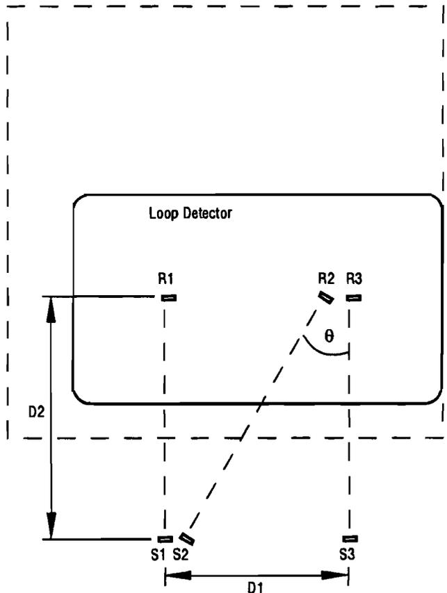
Fig 4.2. Pavement-level sensors.
