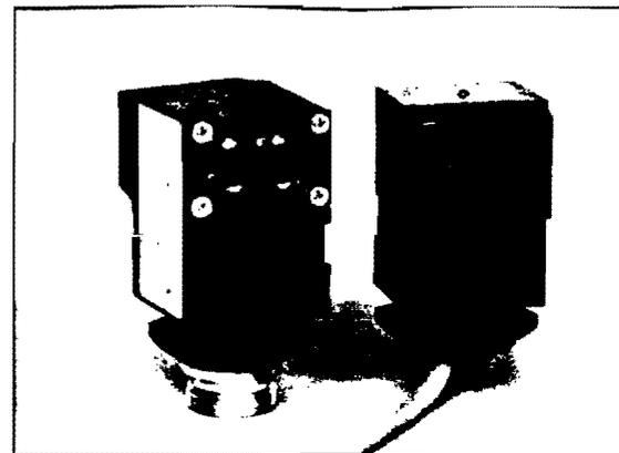
**CONSTRUCTION:** reinforced black Valox™ housing, totally encapsulated circuitry, molded o-ring sealed lenses or fiber fittings, stainless steel hardware. Meets NEMA standards 1, 2, 3, 3S, 4, 4X, 12, and 13.
