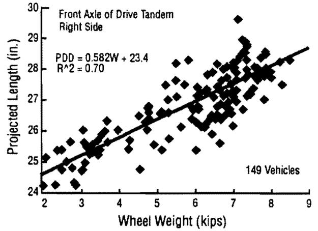
Fig 6.9. Projected diagonal dimension of tire-contact areas versus weight for front axle of drive tandem.
