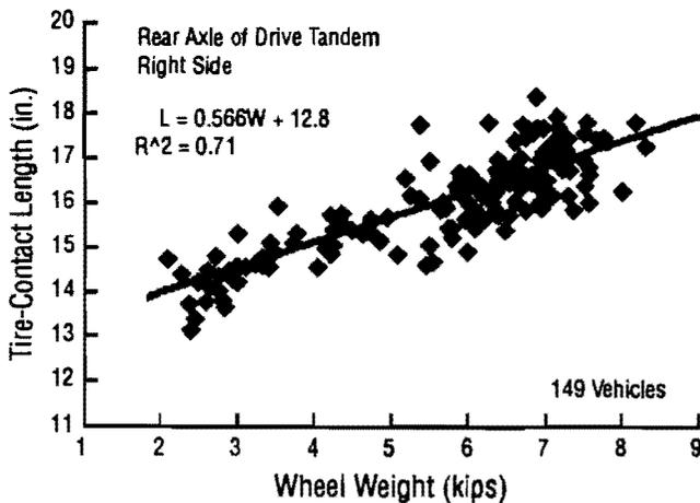
**Fig 6.13. Tire-contact length versus weight for both axles of drive tandem.**
