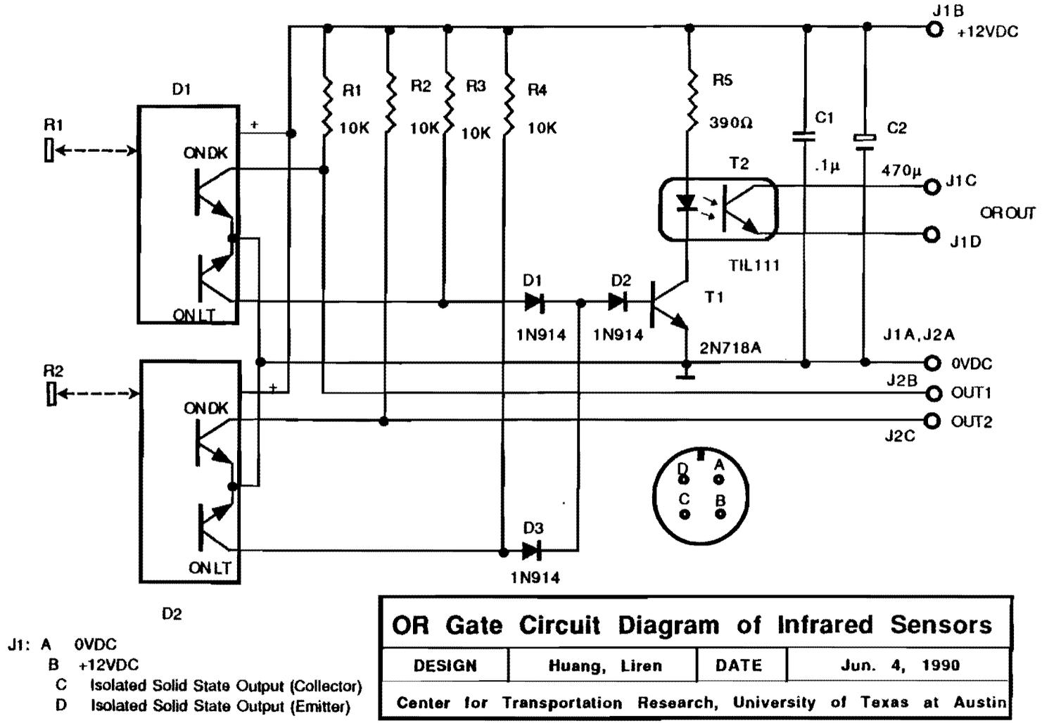
Fig A.7. Circuit diagram for HOV lane in Houston.
