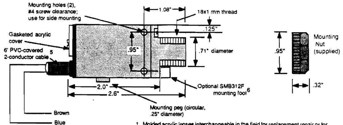
1. Molded acrylic lenses interchangeable in the field for replacement repair or for different sensing ranges.
