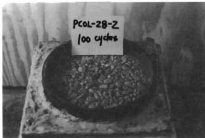
Fig. 4.5. PCOL-28 at Zero and 100 Cycles of Freeze-Thaw Testing.
