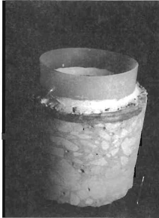
Fig. 5.31. Open Cylinder Sealed to Top Surface Used in 72-Hour Phenolphthalein Soak Test. (Ref 28)
