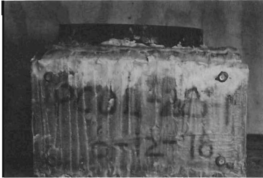
Fig. 3.4. Freeze-Thaw Specimen with Reference Tabs for Strain Measurement.
