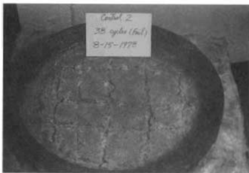
Fig. 4.2. Control Specimen at Zero and 38 Cycles of Freeze-Thaw Testing.
