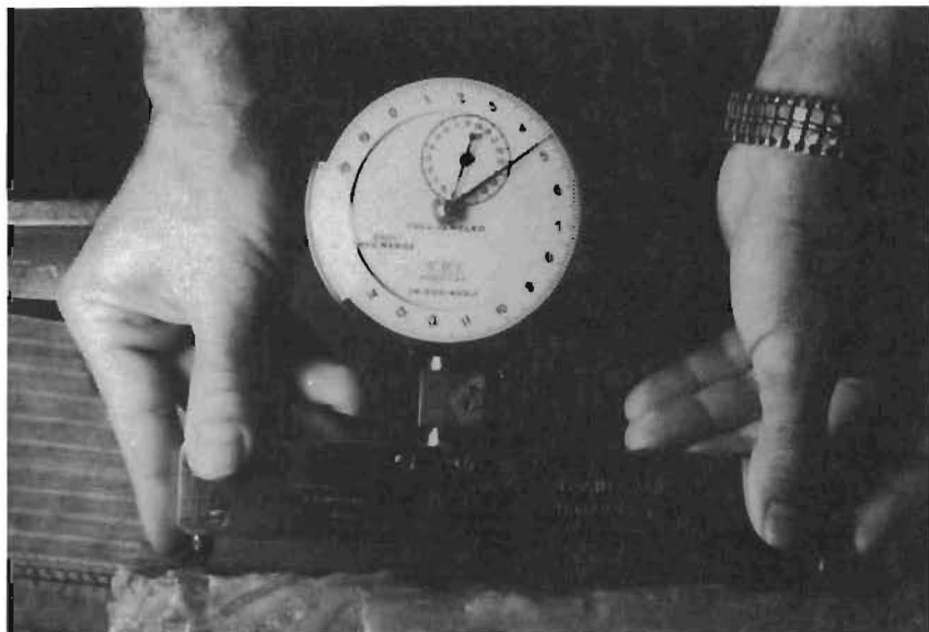
Fig. 3.5. Measurement of Horizontal Strain of Freeze-Thaw Specimen by Use of Berry Gage.
