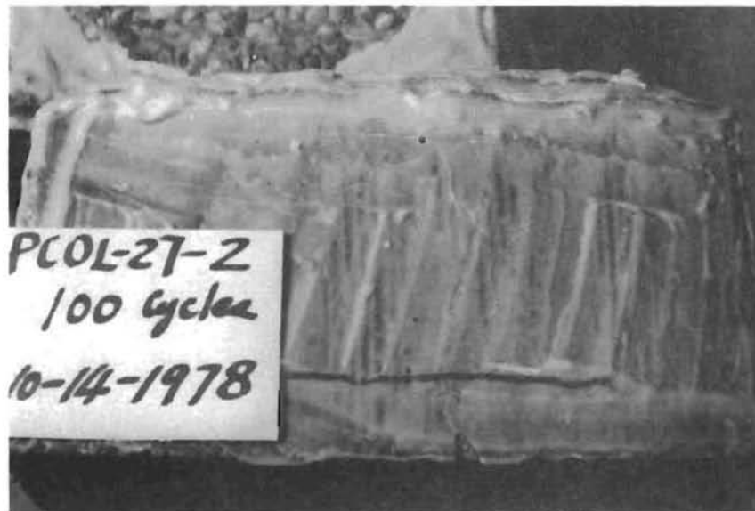
Fig. 4.4. Fine Cracks on the Sides of PC Overlay-27 Specimens.
