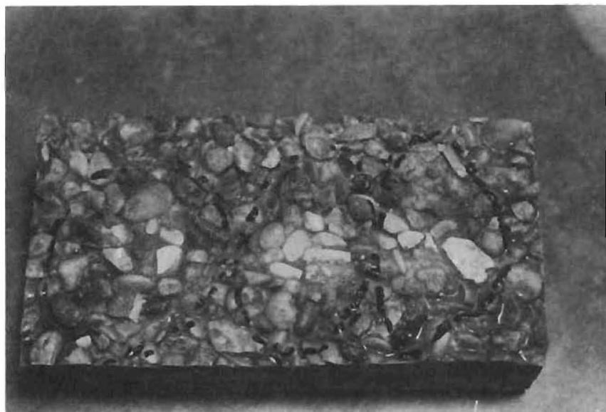
Fig. 4.11. Sandblast Abrasion Specimen of PC Overlay-27 After 100 Cycles of Freezing and Thawing.
