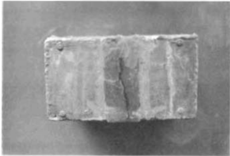
a) Cracking at Interface (Side View)
