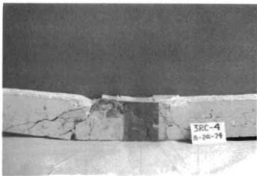
FIG. 4.14 FAILURE MODE OF REPAIRED BEAM 3RC-4
