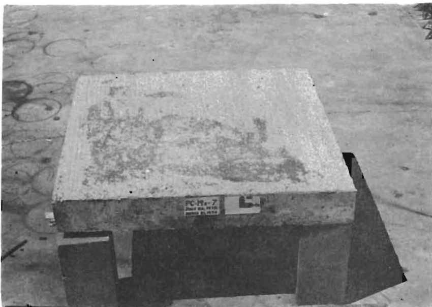
Fig 2.4. Impregnated slab (No. 7) after salt water spray exposure.
