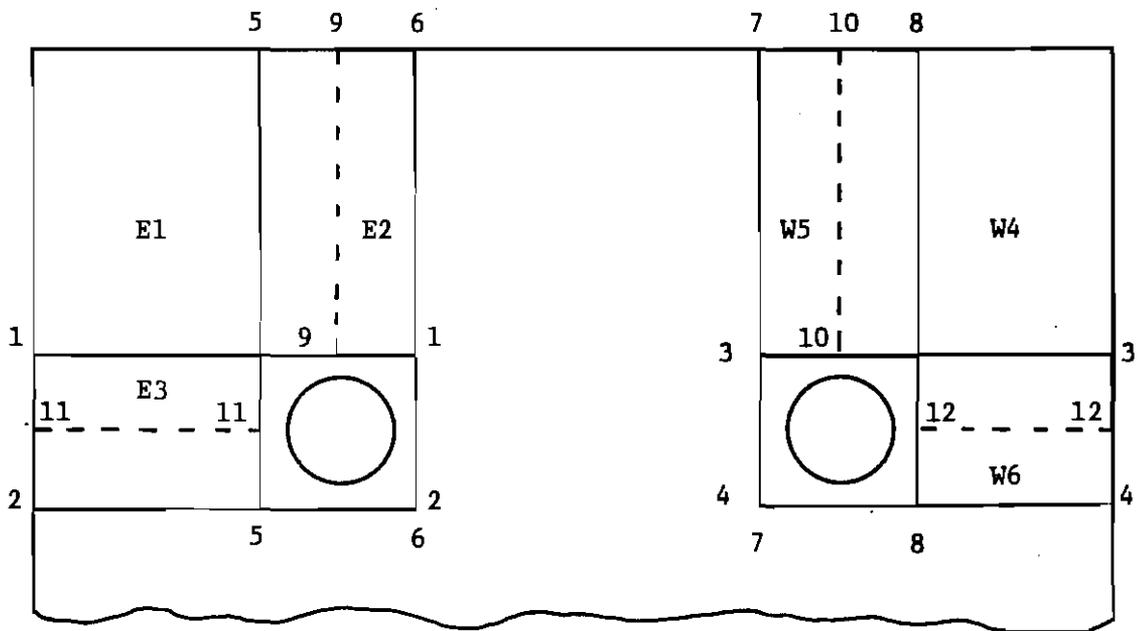
Fig. 4. Primary pattern of saw cuts. The cuts along the dotted lines were made later.
