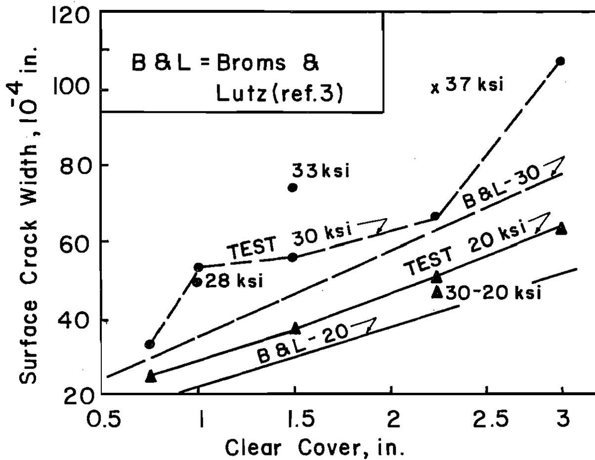
Fig.-14. Average crack width at tension face of beam (all cracks).
