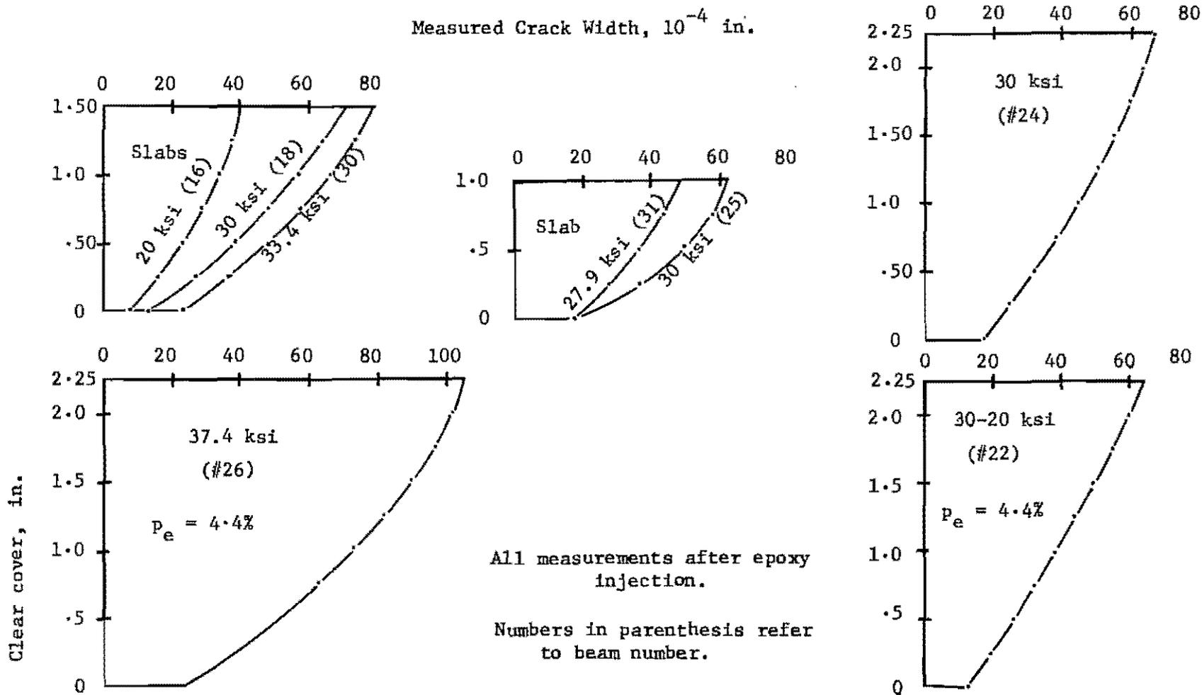
Fig. 19. Best fit curves for crack profiles.
