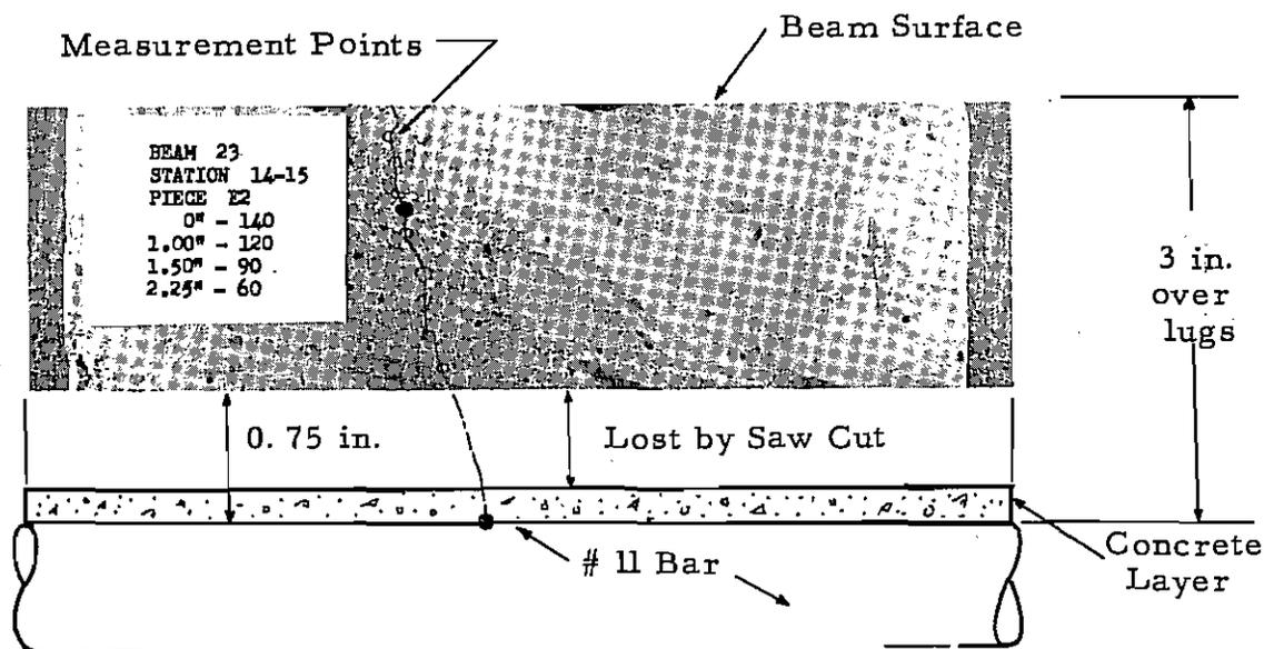
Fig. 8a. Typical variation in crack width.
