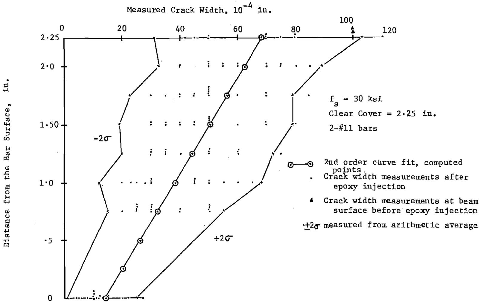
Fig. 17. Best fit crack shape for 30 ksi beam (21-24-11)
