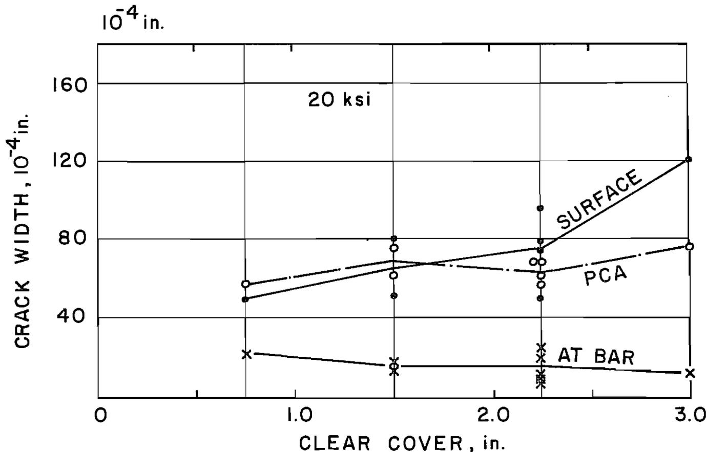
Fig. 12. Maximum crack widths at 30 ksi and 20 ksi steel stress, unless noted.
