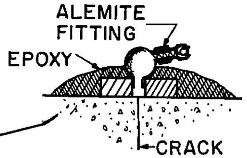
Fig. 3. Injection of colored epoxy. Note epoxy seal over upper part of crack and Alemite fittings for injection. The black streaks are overflow from vent holes.
