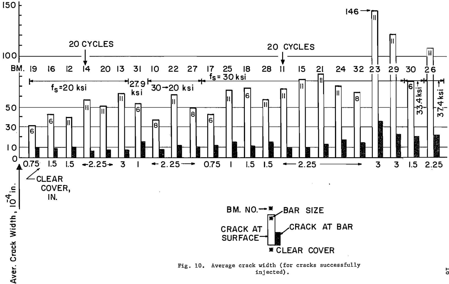
Fig. 10. Average crack width (for cracks successfully injected).
