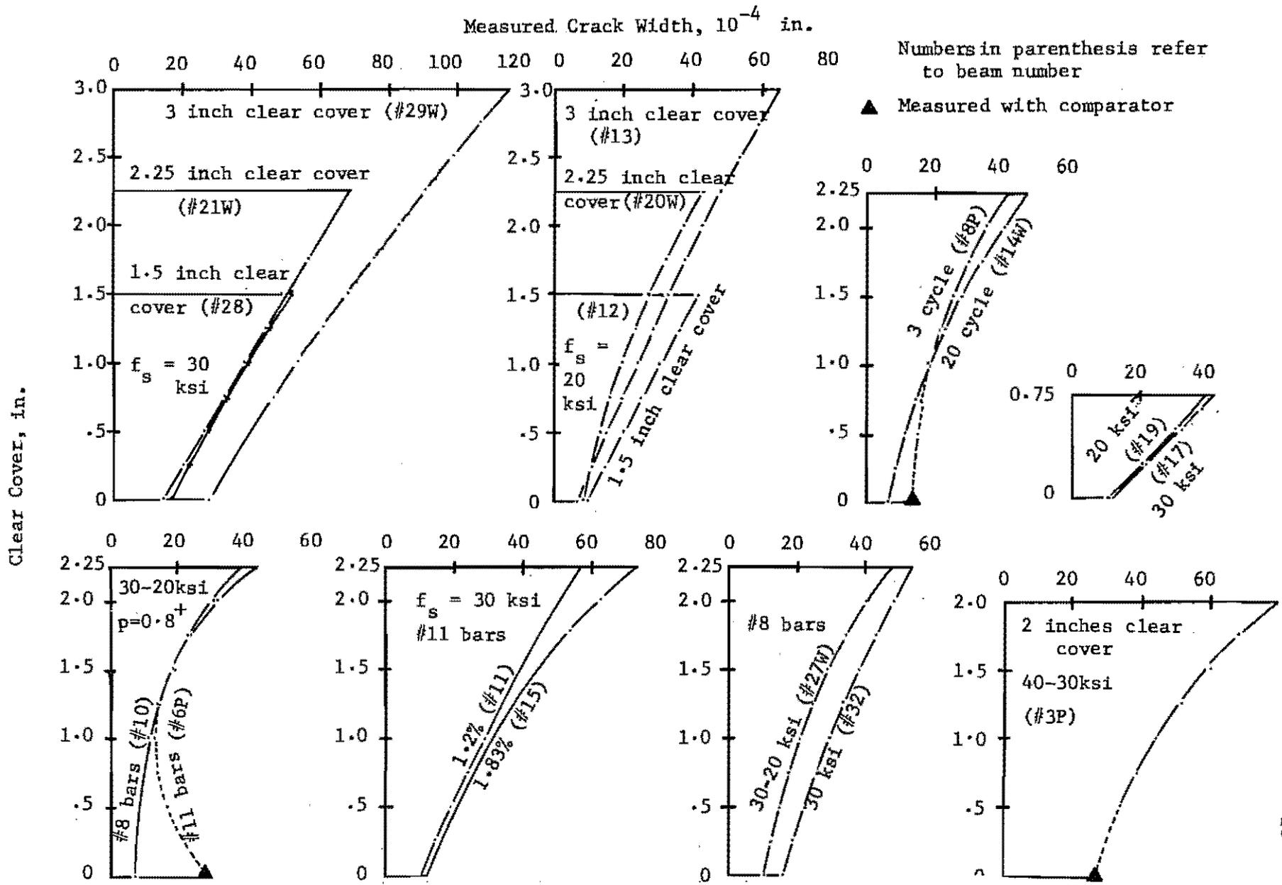
Fig. 18. Best fit curves for crack profiles.
