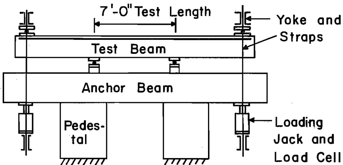
Fig. 1. Arrangement of loading rig.
