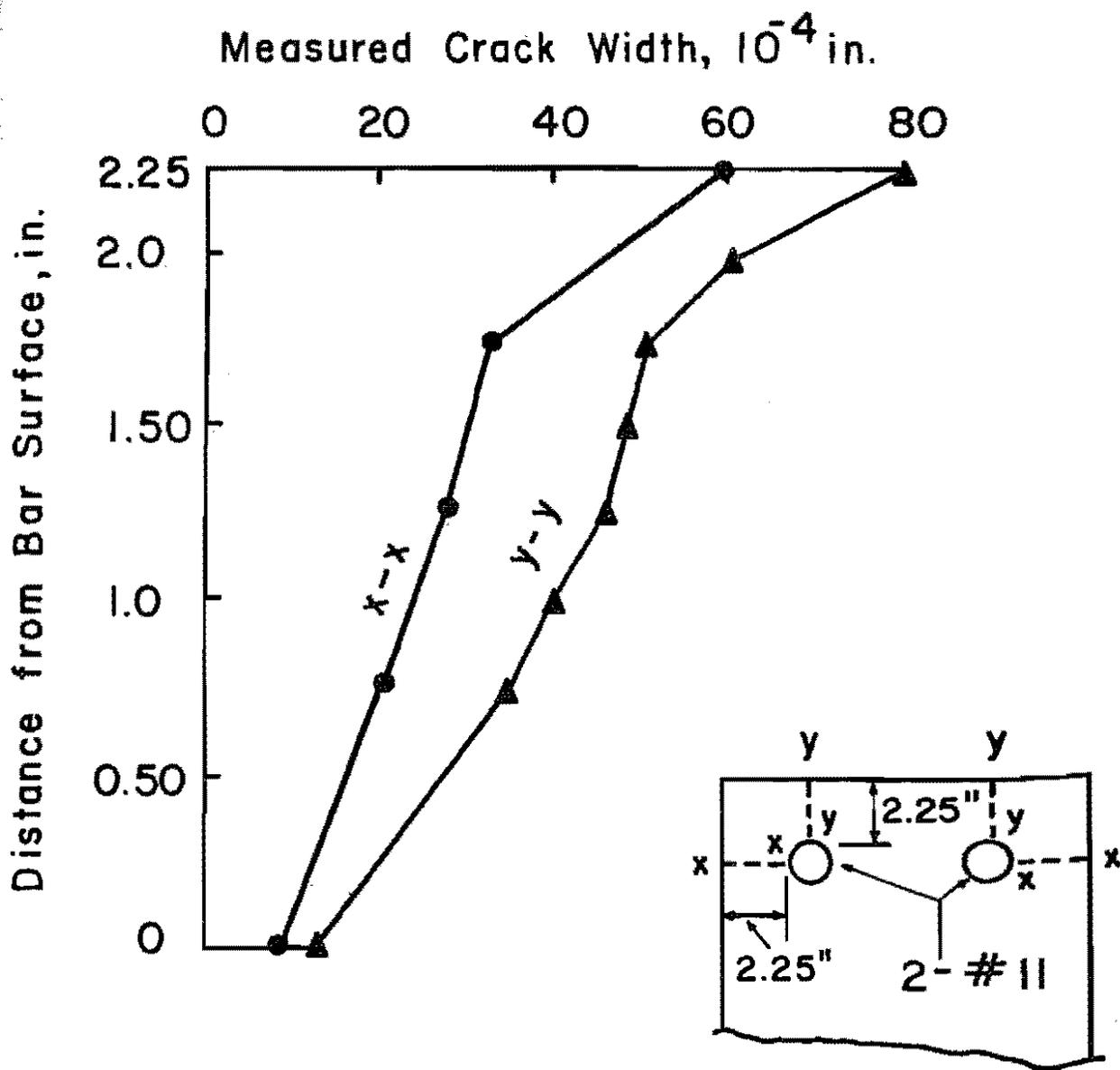
Fig. 20. Average crack width on lateral and vertical planes, at  $f_s = 30$  ksi (#21-24-11).
