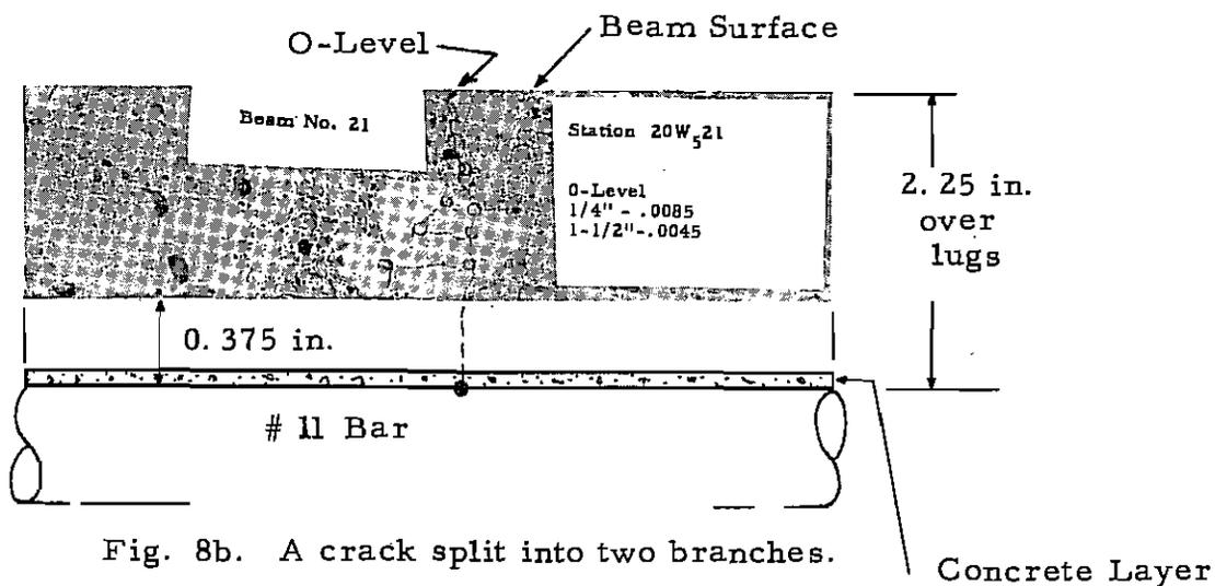
Fig. 8b. A crack split into two branches.
