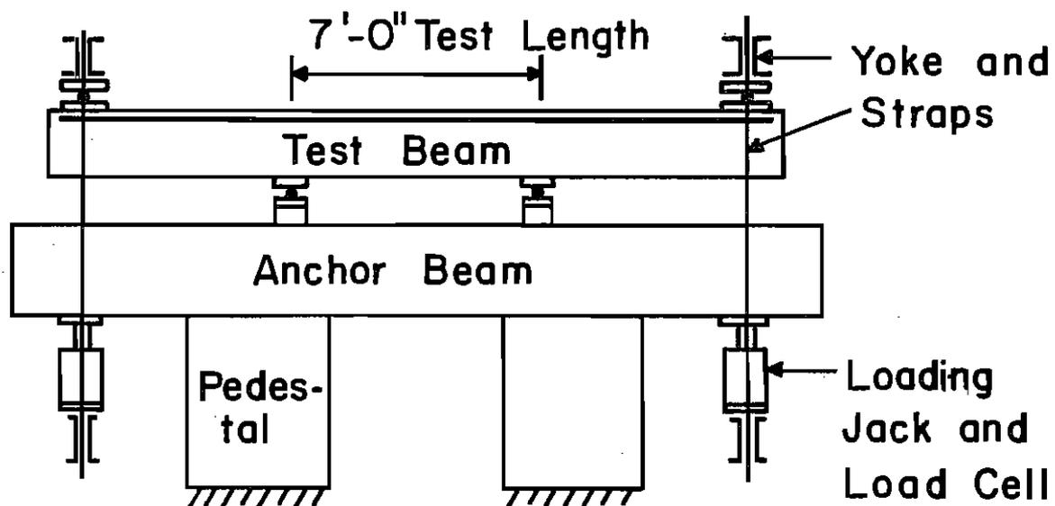
Fig. 1. Arrangement of loading rig.
