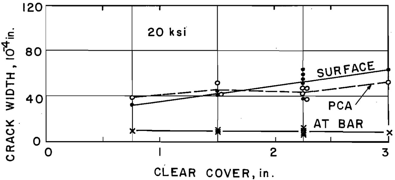
Fig. 11. Average crack widths at 30 ksi and 20 ksi steel stress.
