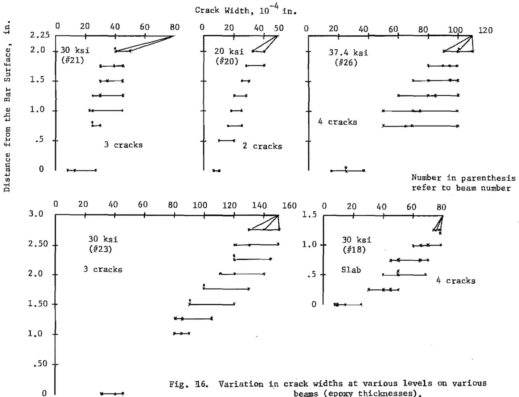
Fig. 16. Variation in crack widths at various levels on various beams (epoxy thicknesses).
