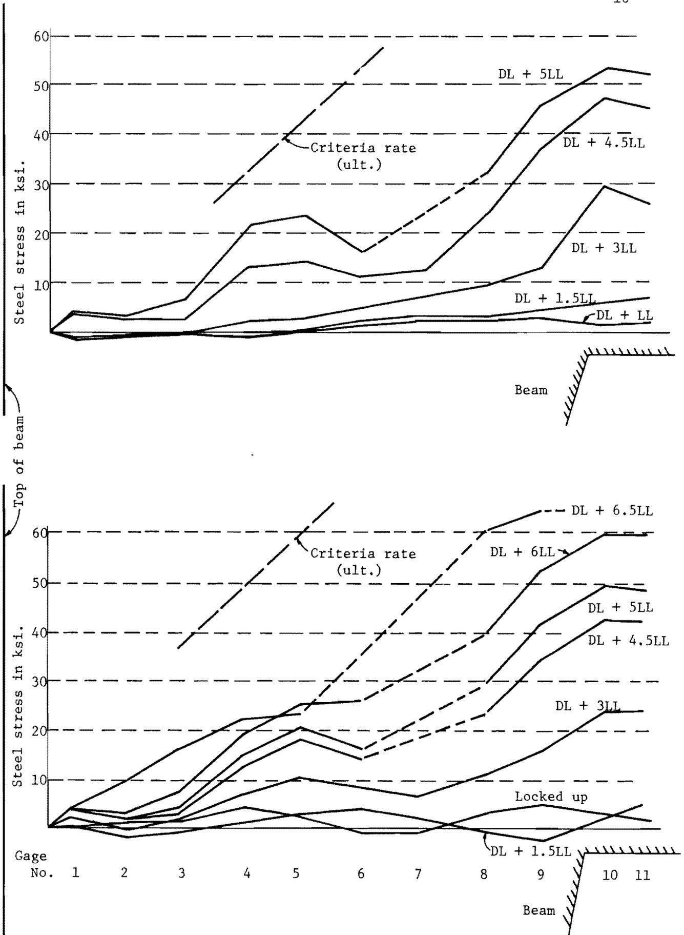
Fig. 11. Steel stress distribution in outer (bottom) bar.
