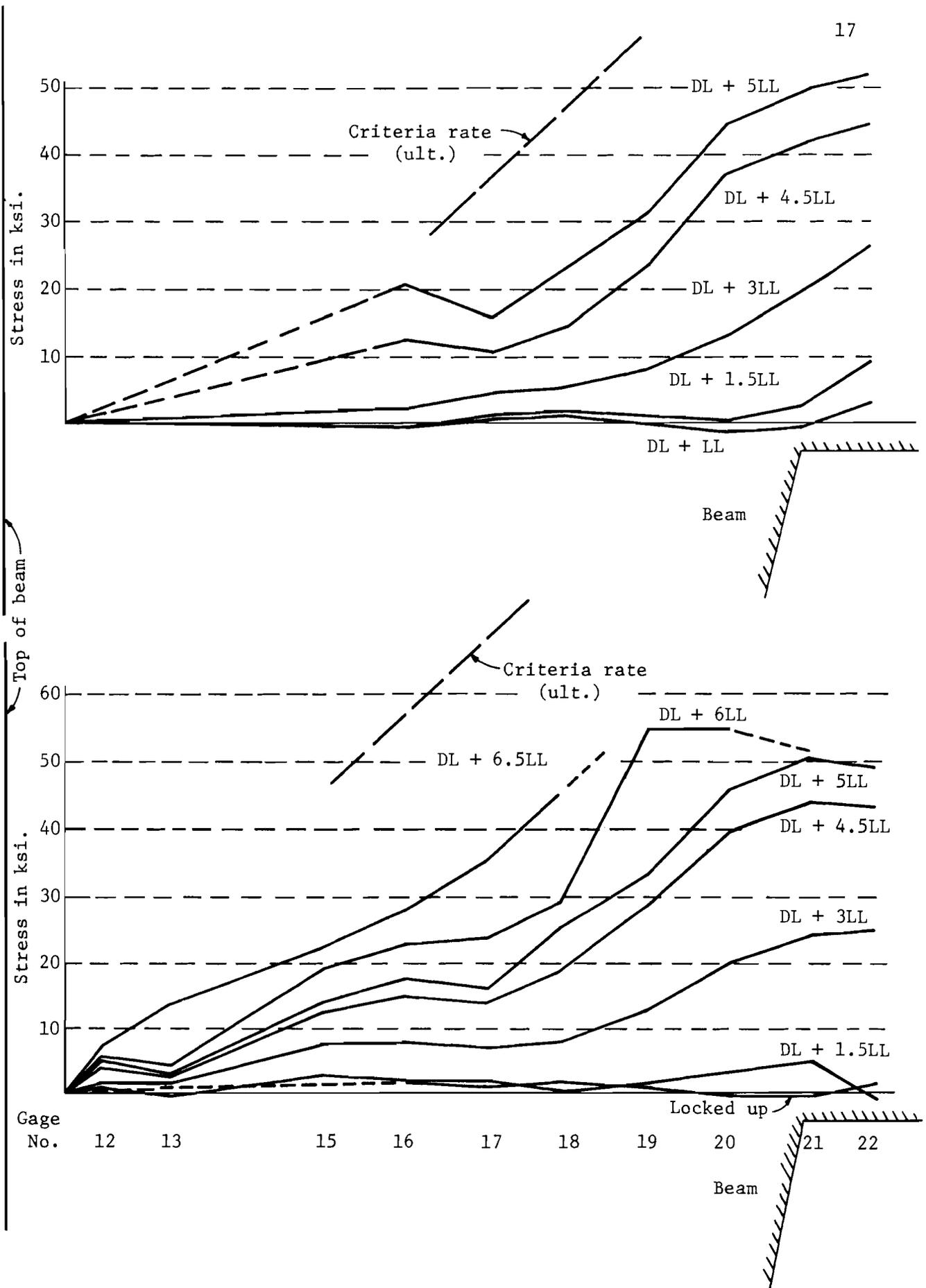
Fig. 12. Steel stress distribution in outer (top) bar.
