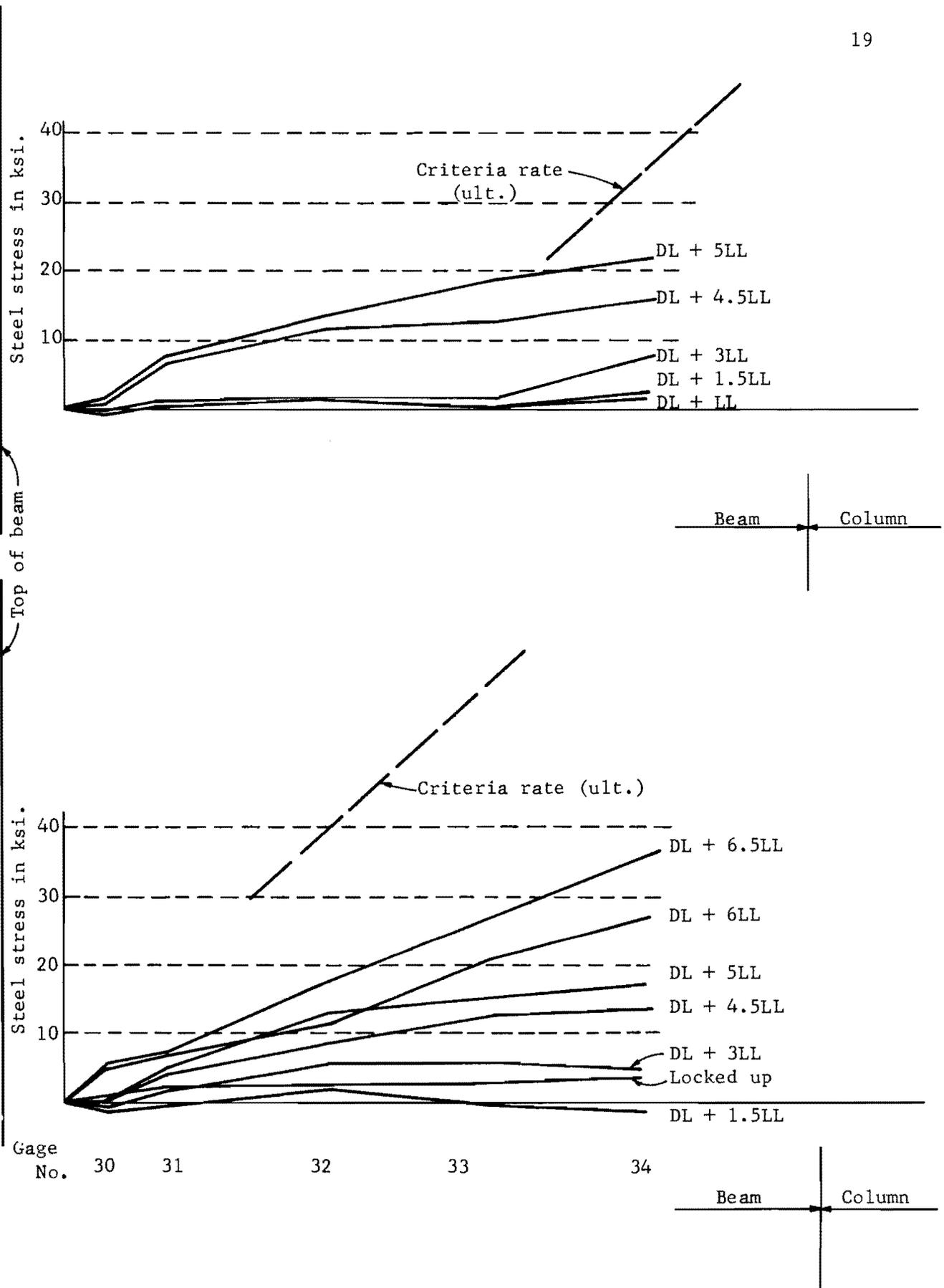
Fig. 14. Steel stress distribution in inner (bottom) bar.
