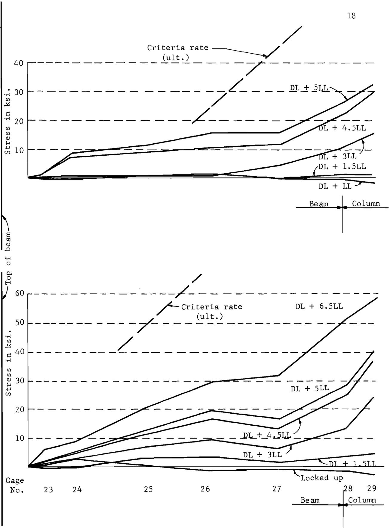
Fig. 13. Steel stress distribution in inner (top) bar.
