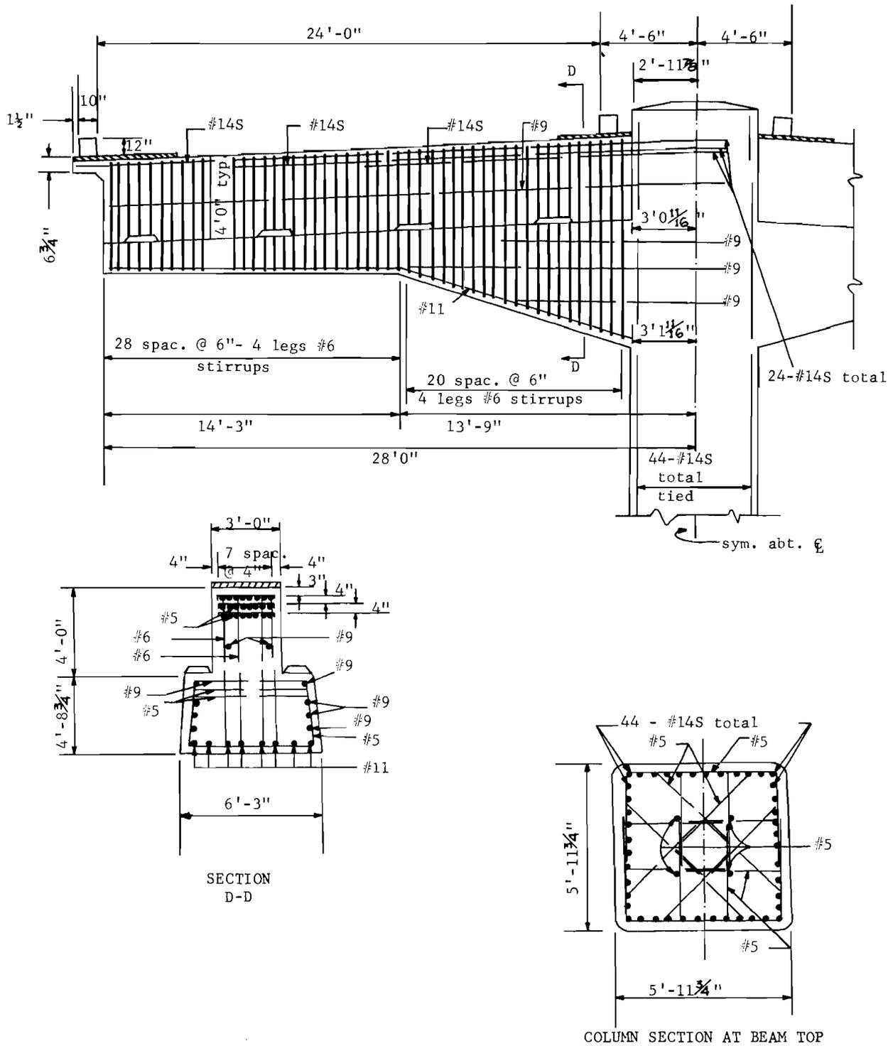
Fig. 1. Details of pylon (prototype).
