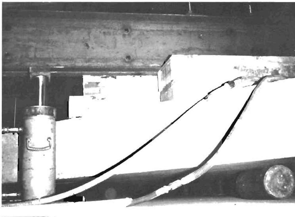
Fig. 5. Lifting of the specimen and placing on rollers.
