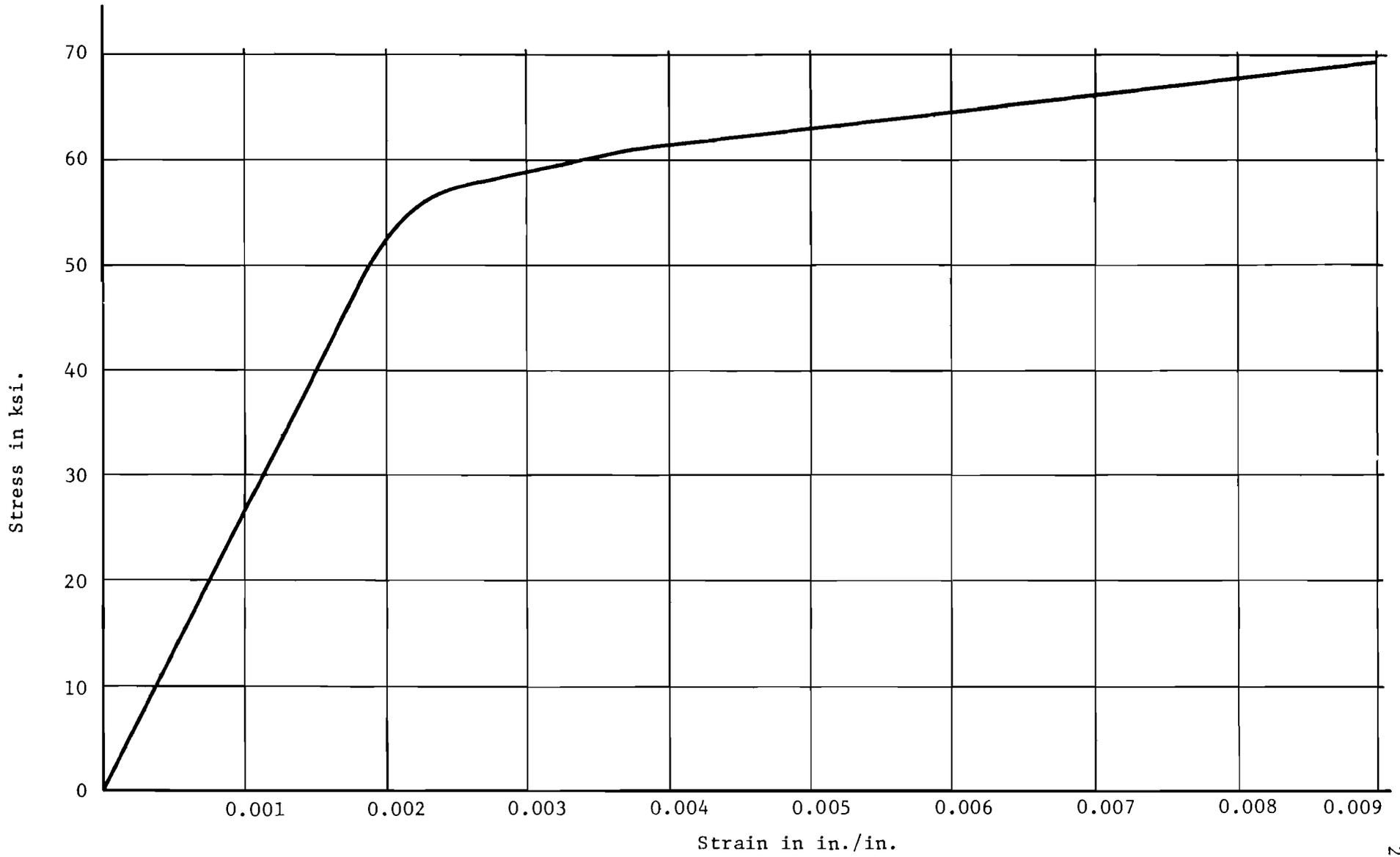
Fig. 15. Steel stress-strain curve for #14S bar.
