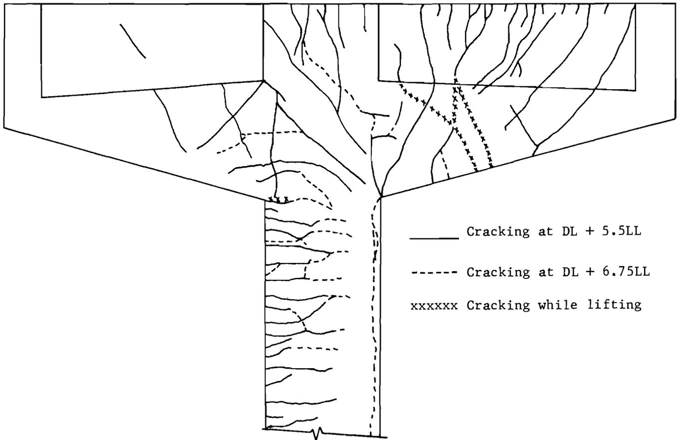
Fig. 9. Crack pattern of the specimen.
