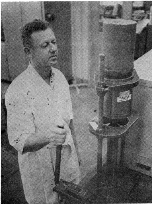
Figure 9. Extruding the LFA specimen from the 6 inch by 8 inch compaction mold.
