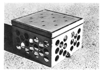
Load Cell for Measuring Dynamic Driving Forces on the Top of Concrete Piles
