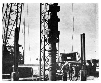
View of Link-Belt Speeder 520 diesel hammer, load cell, and 16-inch diameter steel pipe pile at Port Arthur field test location. Reaction piles for static load test are shown on left and right.
