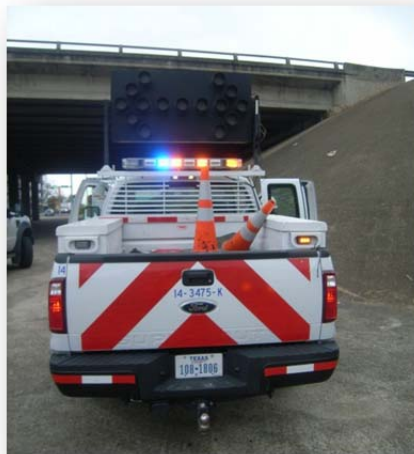
Figure 9: Minimum Truck Requirements for VSDO
