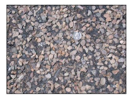
TxDOT standard specification Item 302 defines Grade 4 rock as having a nominal size of 1/4 inch. The particle size is generally smaller than 3/8 inch, but larger than 0.19 inch (number 4 sieve).
