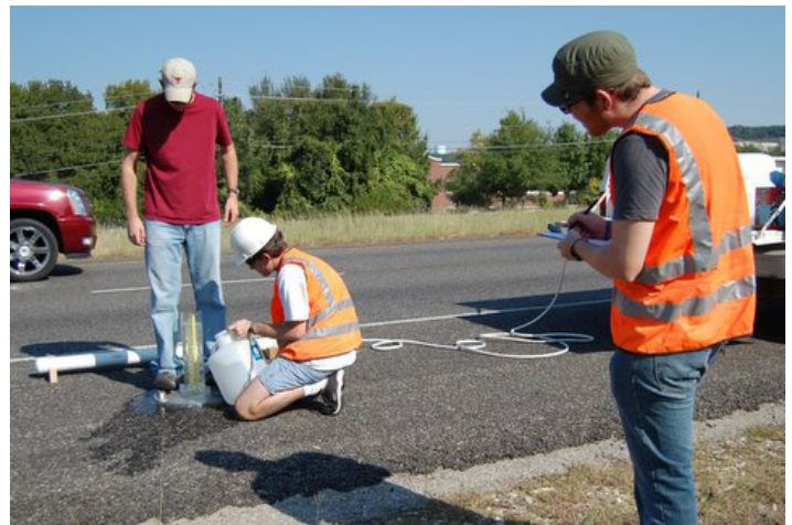
Above and left: Ph.D. students Brandon Klenzendorf and Brad Eck perform a field test of PFC permeability using a testing device developed by the project team. MS student Patrick Frazier records test results.
