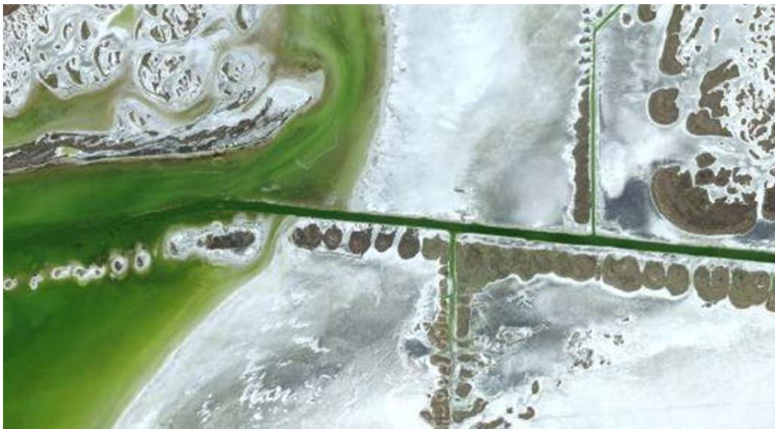
Figure F23: An aerial photograph of the GIWW connecting to the Laguna Madre near Port Mansfield. Dredged silt is dumped in piles along the waterway.
