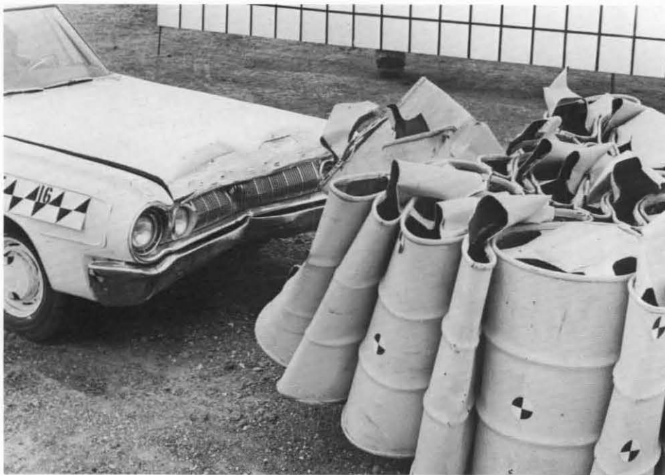
Figure F-8. View of minor vehicle damage. Only one of four headlights was broken. Bumper and grill deformed approximately 4 in.
