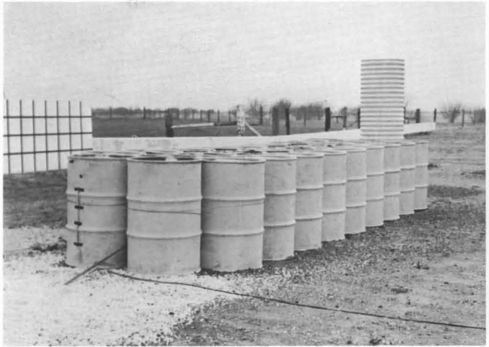
Figure F-5. Barrel protective barrier installed in front of 30 in. diam. simulated bridge pier
