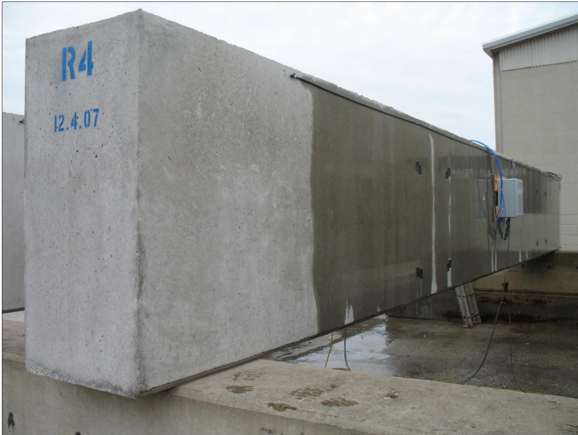
Figure 4-5: Demonstration of Watering System
