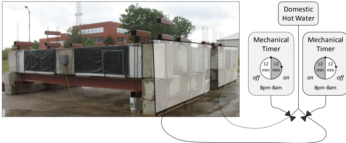
Figure 4-6: Alternating Two-Zone Watering System
