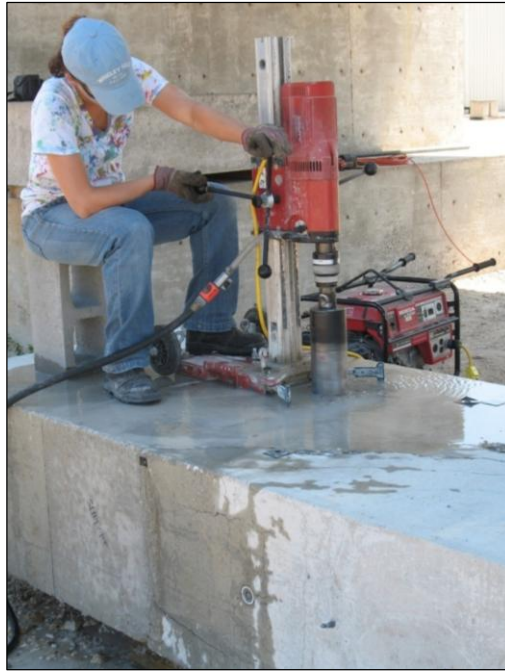
Figure 4-30: First Series Specimens - Extraction of Cores
