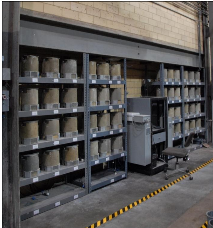
Figure 3-22: FSEL Sure Cure System – Controller and Molds
