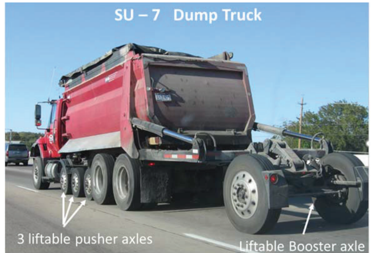
Figure 1. SU-7 dump truck with three liftable pushers and one liftable booster axle
