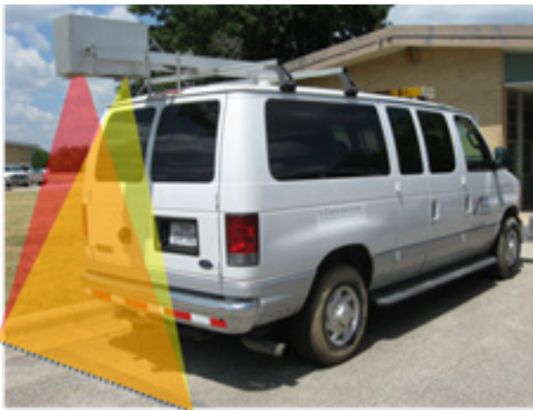
Figure 1: TxDOT 3D automated system
