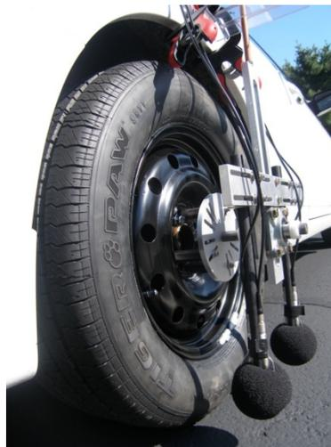
*Figure 3.5: OBSI device microphones*
