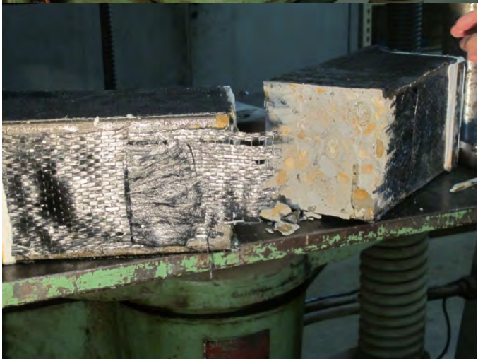
Figure C2: Successful test with CFRP sheet fracture
