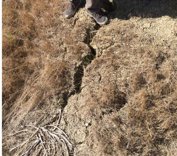
*Figure 4.18: Cracking of Heiden Clay near La Frontera Blvd*
