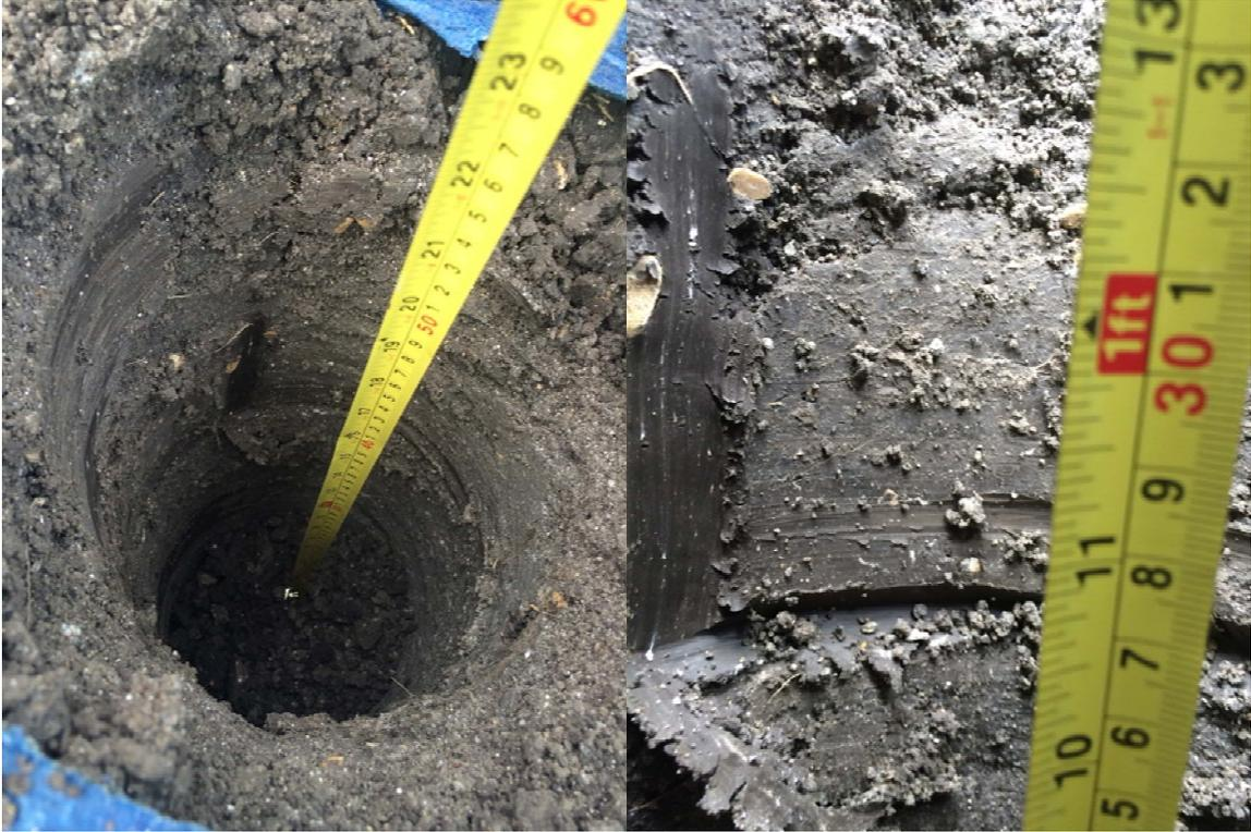
*Figure 4.22: Augured Hole and Soil Samples from FM 971*
