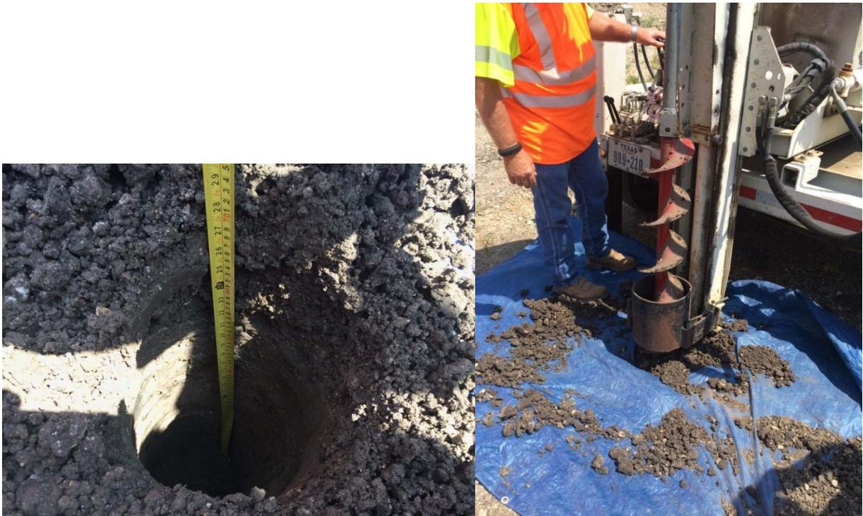
*Figure 4.34: Augured Hole and Soil Samples from Taylor Maintenance Office*
