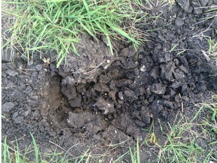
*Figure 4.5: Sample of Tinn Clay from Field Sampling*
