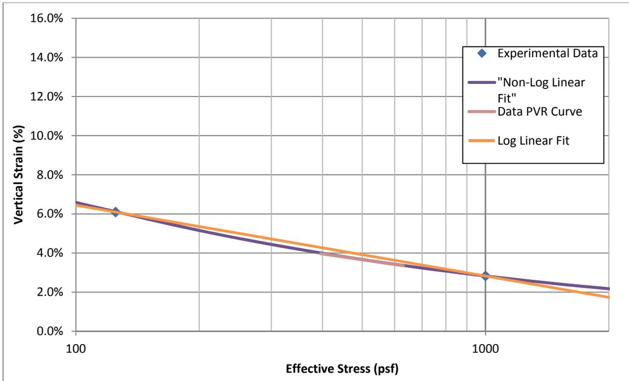
Figure 5.25: Swell-Stress Curves for Turnersville Road Bulk Samples
