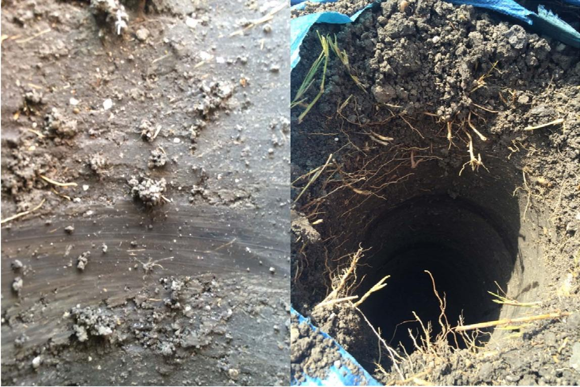
*Figure 4.30: Augured Hole and Soil Samples from SH 95*
