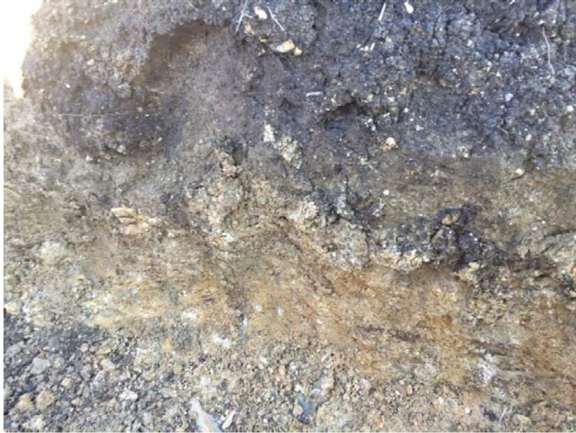
*Figure 5.43: Soil Strata Delineation between Branyon Clay and Krum Soil at FM 685*
