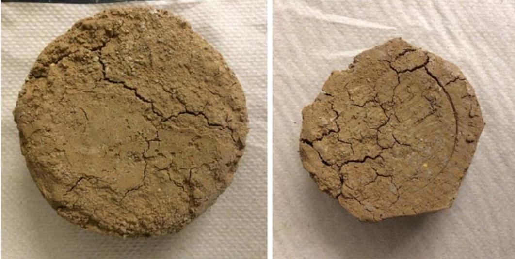
*Figure 2.4: Shrinkage Cracks formed from rapid drying.*
