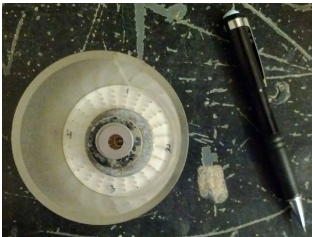
Figure 7: Assembled Permeameter Cup with Overburden Washers and Washers Simulating 51.3 Grams of Overburden from the Ponded Water
