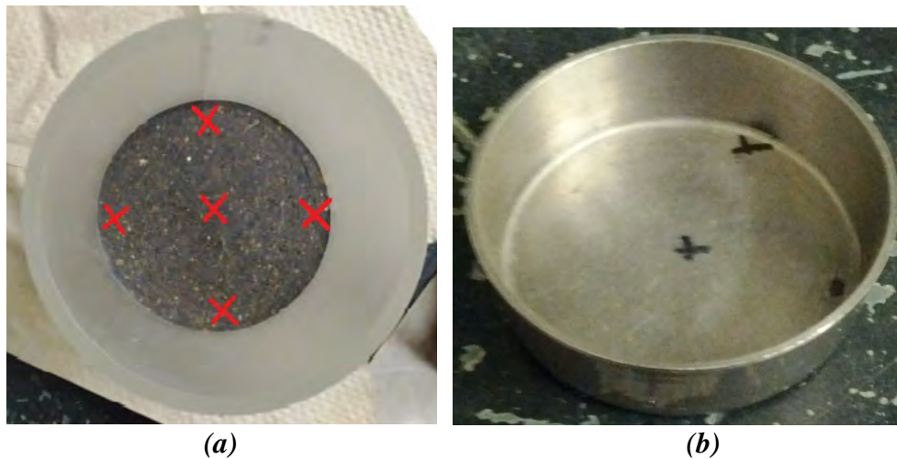
Figure 2: (a) Location of Sample Height Measurements throughout Testing Procedure (b) Metal Plate Used in Determining Sample Height
