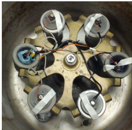
Figure 8: Assembled Testing Setup within the Centrifuge
