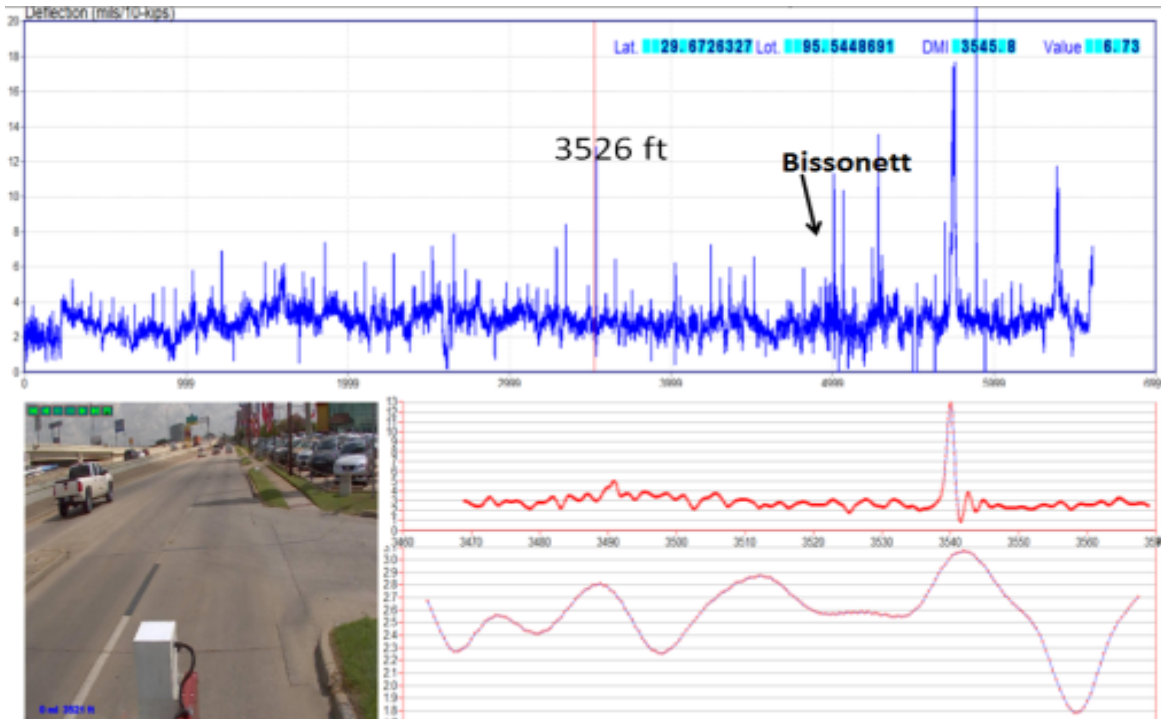
Figure 2.16: Typical Maximum Deflection Pattern on the Section from BW 8 to Bissonett
