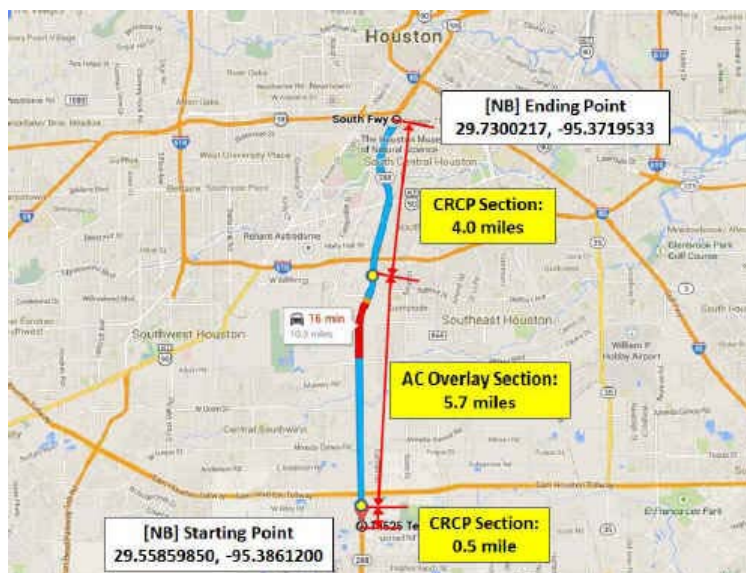
Figure 2.28: TPAD Testing Location and Pavement Types on SH 288 in Houston, TX
