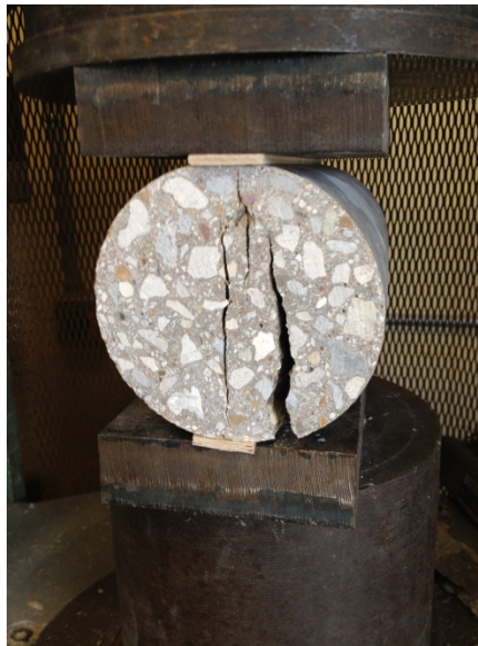
Figure 3.3- Testing for splitting tensile strength.
