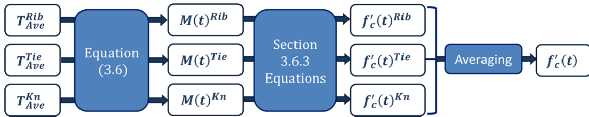
Figure 5.1- Procedure for calculating the maturity-based compressive strength of the arches.
