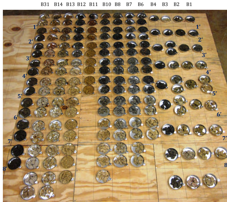
Figure 3.22 Diversity of subsurface soil types in Borings B1 to B31 from the ground surface to the maximum depth of 9 ft.
