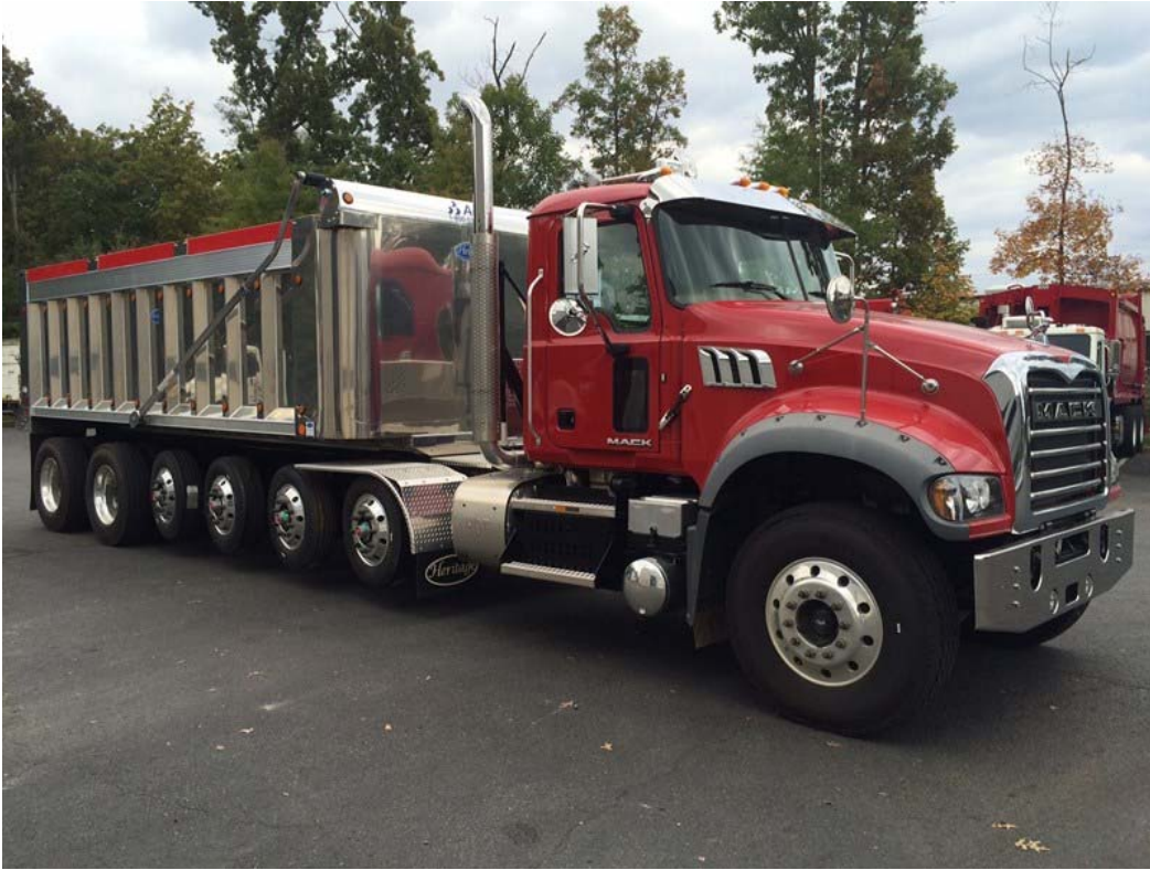
Figure 9.3: SU7 dump with four liftable pusher axles (single tires), no booster axle, with long outer bridge length (uncommon; seen in Texas)
