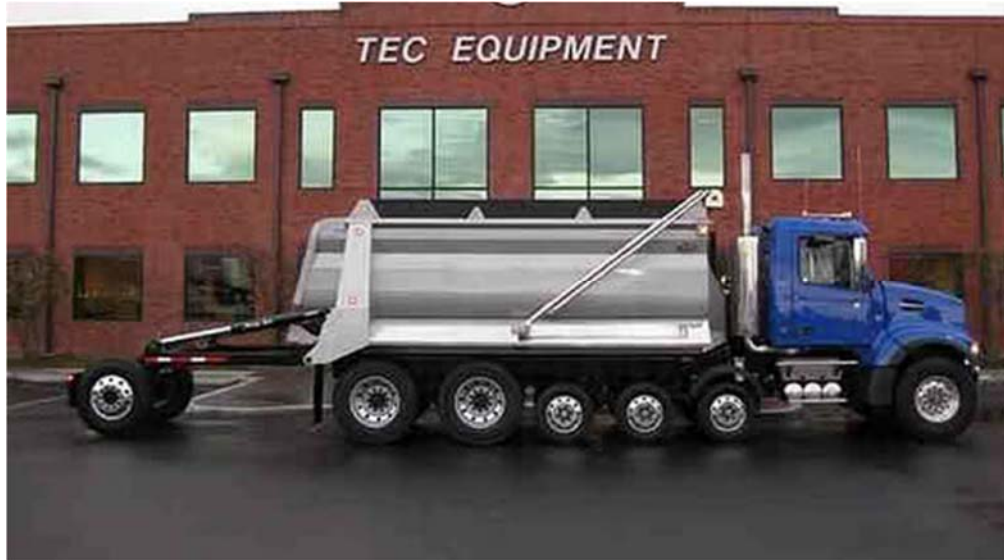
Figure 9.1: SU7 dump with three pusher lift axles with single tires and one booster lift axle (a common configuration; seen in Texas)
