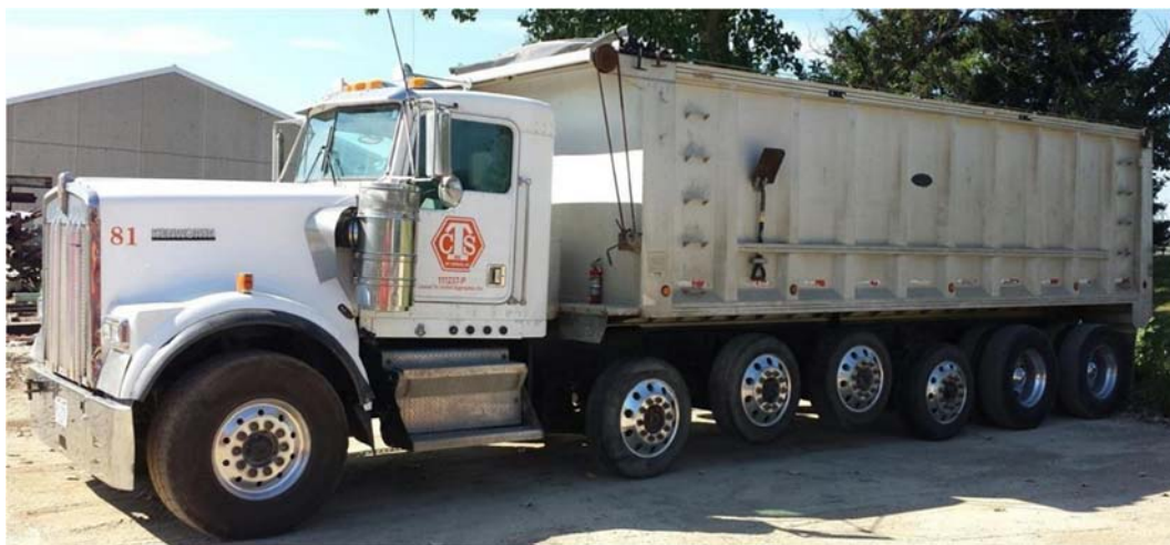
Figure 9.2: SU7 dump with four liftable pusher axles (single tires) but no booster axle (an uncommon configuration; seen in Texas)
