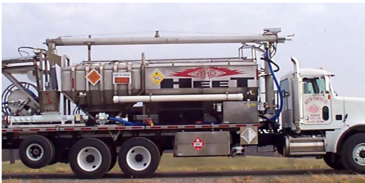
Figure 3.2: Austin Powder quarry explosives transport truck (different design) (SU4 with lifted tag axle)
