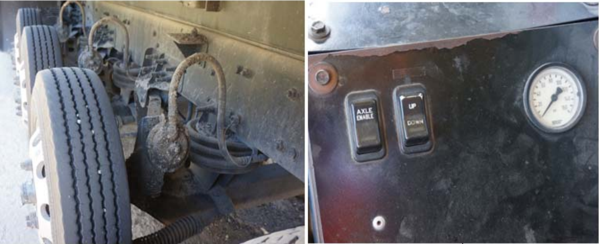
Figure 3.14: Control system of the liftable axles
