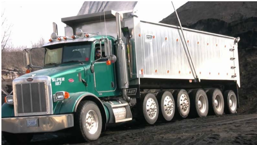
Figure 9.4: SU7 dump with three liftable pusher axles with single tires and one liftable tag axle with dual tires (operates in Kentucky and possibly other states; not observed in Texas during this study)
