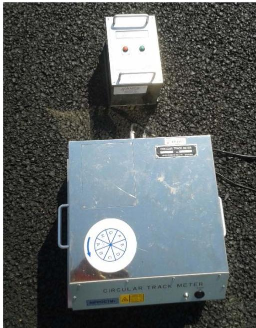
*Figure 4.6: LTS (top) and circular track meter (bottom).*
