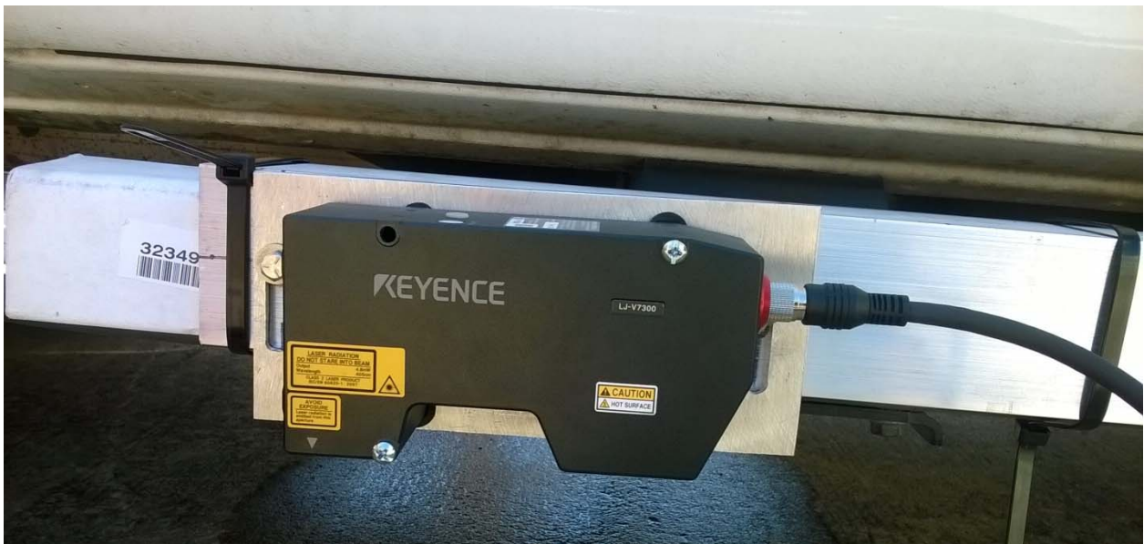
Laser sensor system, as mounted on Ford F150 light truck. The top image shows the system mounted on the truck nerf bar. The bottom image provides a close-up view.
