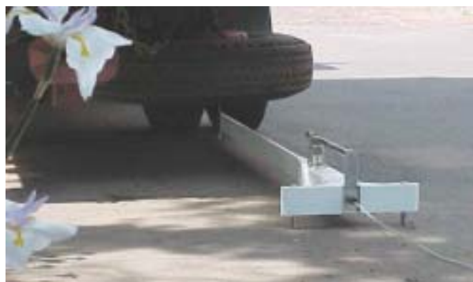
Figure 1.2 RSD during deflection measurements
