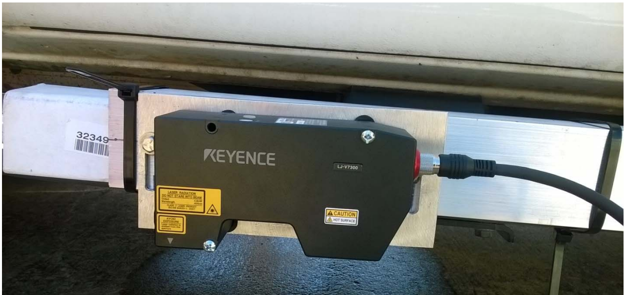
Figure 8.1 Experimental data acquisition setup, as mounted on Ford F150 light truck. The top image shows the devices as mounted on the truck nerf bar. The bottom image shows a close-up view of head B, as mounted on the aluminum profile.
