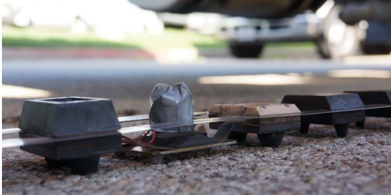
Figure 1.7 Detail of Curviameter’s geophone on the pavement surface
