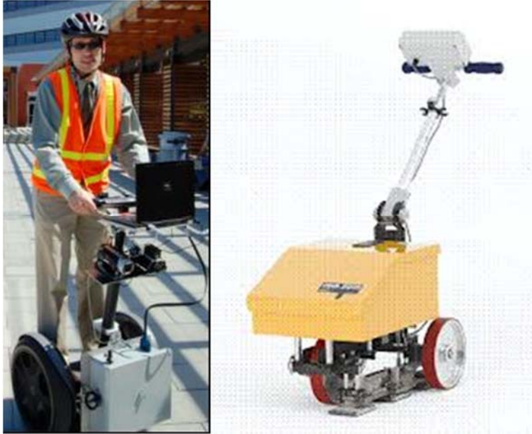
Figure 2.6 Alternative devices: a) ULIP Segway, b) AMSKAN IRIS 2000
