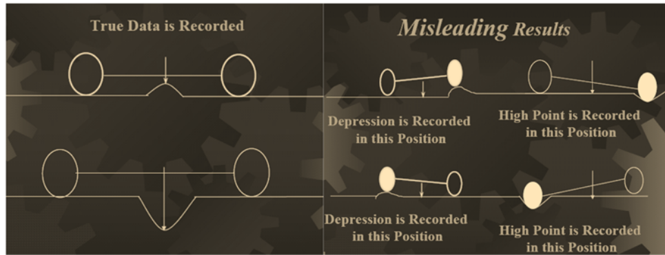
Figure 2.4 An example of accurate and inaccurate results from a rolling straightedge's recording (Vitillo, 2016)
