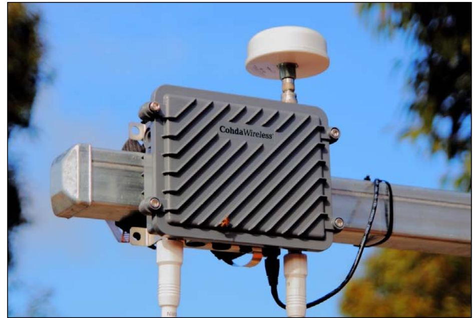
DSRC Beacons (or LTE Small Cells)
