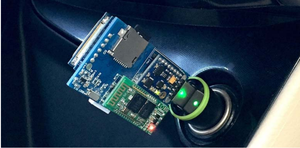
Figure 3.8: IMU Device Installed in a Vehicle, with Power Supplied through a USB Car Charger.
