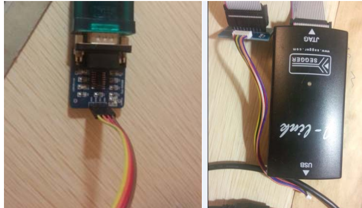
Figure 3.7: JTAG Programming System. Left: RS232 Interface. Right: JLink Programmer
