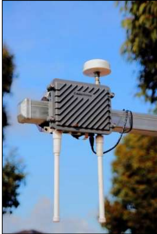
Figure 19.1 An example of an RSU device, a Cohda MK5 RSU
