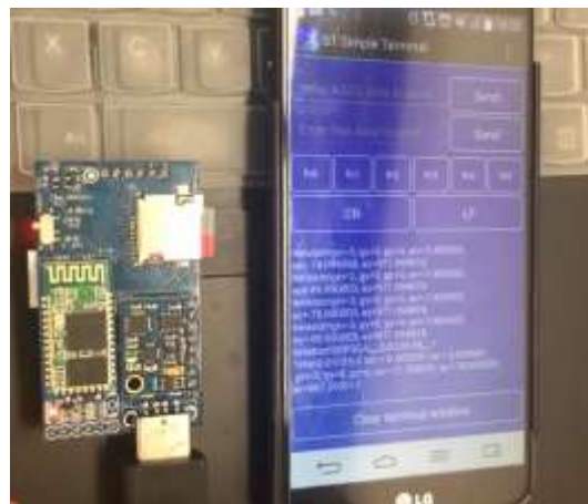
Figure 17.3 Transmission of data to an Android phone via Bluetooth
