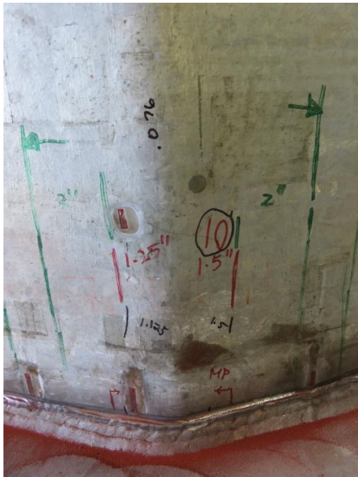
Figure 8.36: Grinding Continued to Remove Magnetic Particle Evidence of the Cracks: Specimen 33-3-12-TX-A3 – Bend 10
