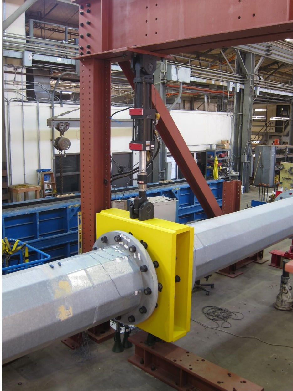
Figure 5.17: MTS 55-kip Hydraulic Actuator and the Stiff Reaction Box (the Load Box)
