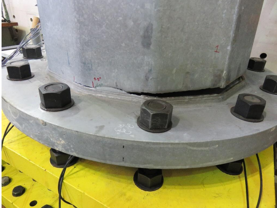
Figure 5.106: Propagation of Cracks in the Damaged Specimen 33-3-12-TX-A1 Following the Ultimate Strength Test
