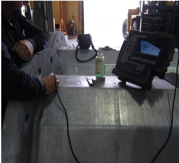
Figure 5.37: Hargang X-32 PAUT Instrument Used in Detecting Cracks in an HMIP Specimen
