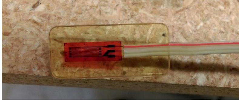
Figure 6.18: Strain Gage to Monitor Wind-Induced Stresses
