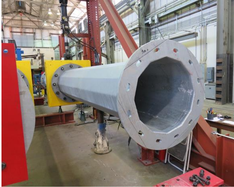
Figure 5.23: A specimen supported on a jack during Final Stages of installation.
