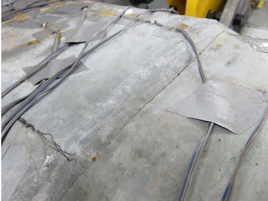
Figure 5.95: Specimen 33-3-12-TXEC-A7 (Bends 10 and 11) following the Fatigue Test 7 at the Combined Stress Ranges of 3 ksi and 5 ksi (Fatigue Cracks after 4.2 Million Cycles)
