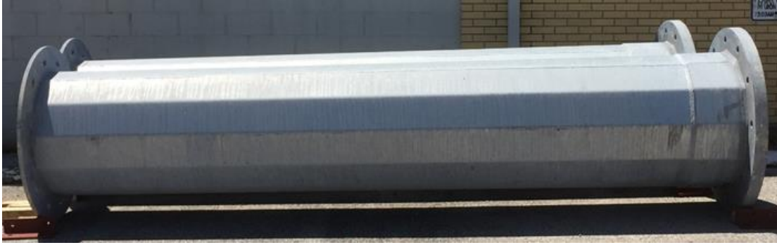
Figure 5.10: HMIP Fatigue Test Specimens of Secondary Interest following Fabrication
