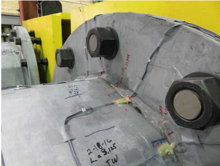
Figure 5.73: Specimen 33-3-12-TX-A4 following the Fatigue Test 3 at the Stress Range of 4 ksi (Fatigue Cracks after 3.8 Million Cycles)
