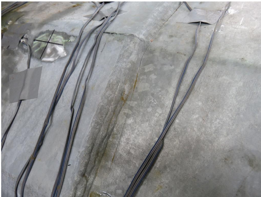
Figure 5.96: Specimen 33-3-12-TXEC-A7 (Bends 10 and 11) following the Fatigue Test 7 at the Combined Stress Ranges of 3 ksi and 5 ksi (Fatigue Cracks after 4.2 Million Cycles)
