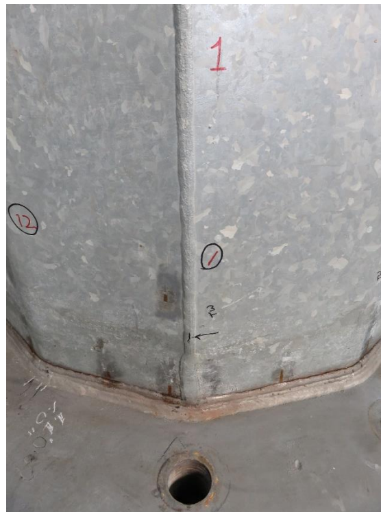
Figure 8.10: State of Cracks: Specimen 33-3-12-TX-A2 – Bend 1
