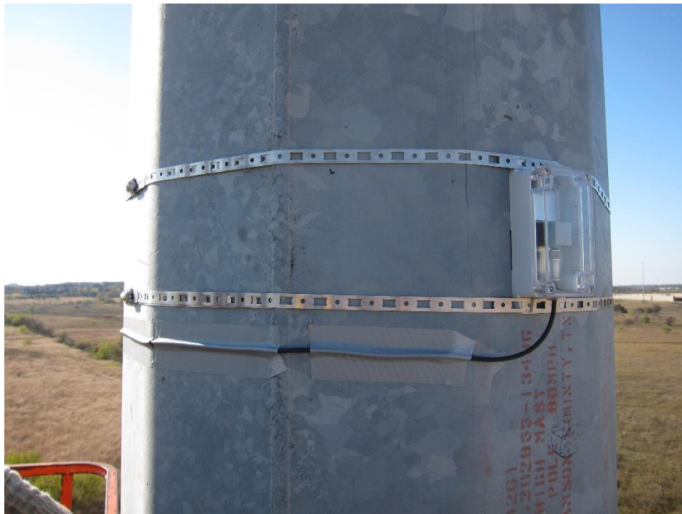
Figure 6.32: Accelerometer Clamped on to the HMIP in Austin
