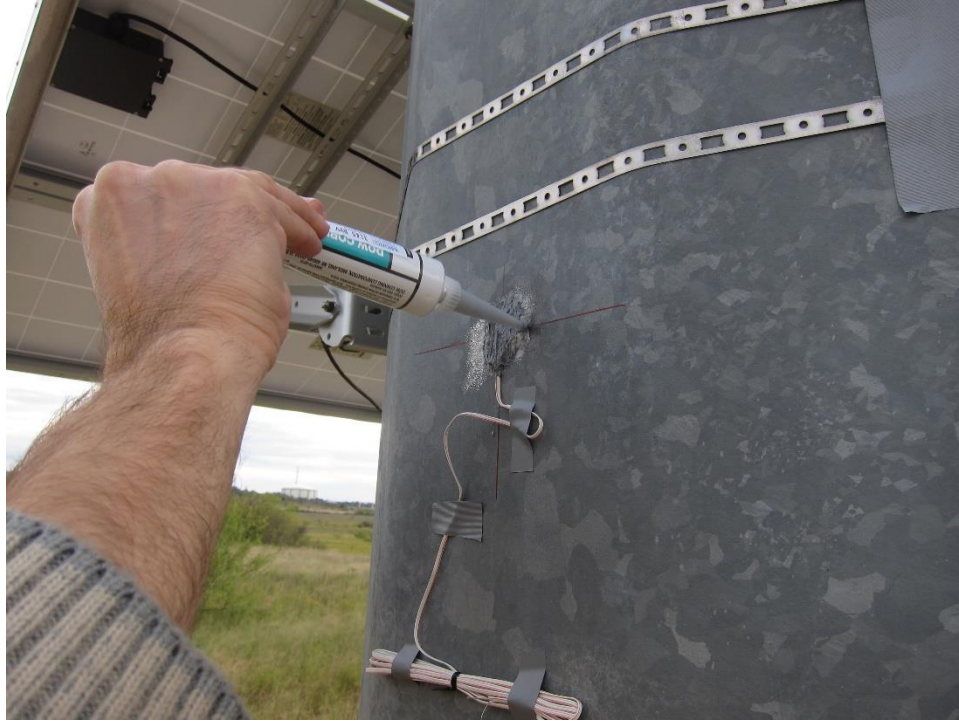
Figure 6.37: Silicon Epoxy to Protect the Strain Gages from Environment
