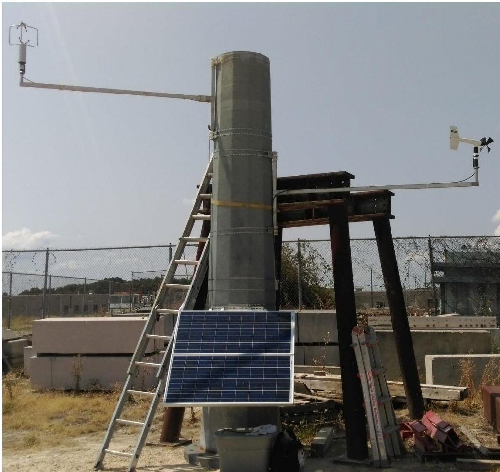
Figure 6.26: Anemometers and Solar Panel Installed on a Mock-up Pole
