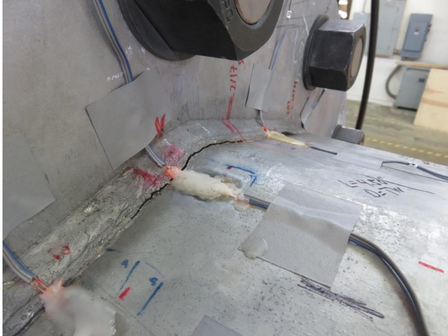
Figure 5.74: Severe Cracking on Bend 4 of the Specimen 33-3-12-TX-A4 following the Fatigue Test 3 at the Stress Range of 4 ksi (Fatigue Cracks after 3.8 Million Cycles)
