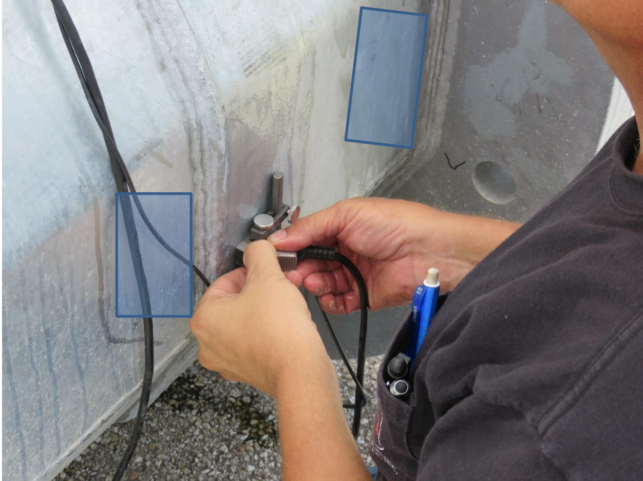
Figure 5.42: Probe Locations in PAUTs Conducted on the Specimens of Secondary Interest
