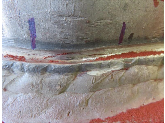
Figure 8.37: Grinding Continued to Remove Magnetic Particle Evidence of the Cracks: Specimen 33-3-12-TX-A3 – Bend 10
