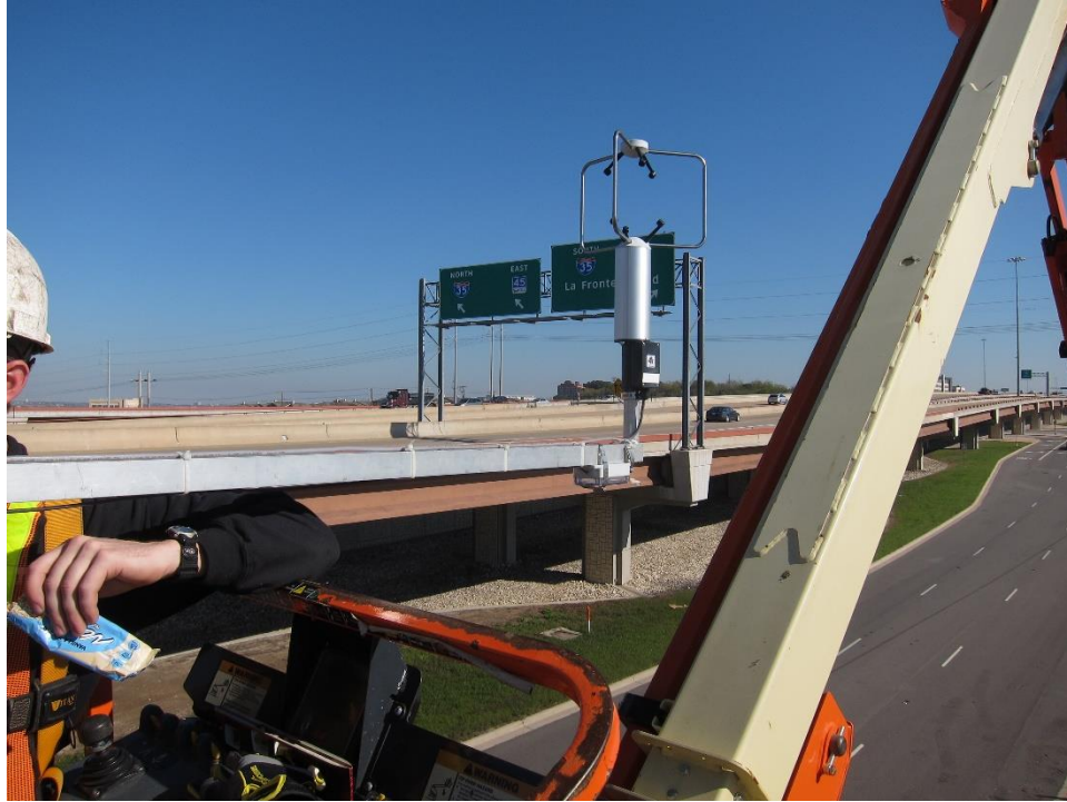
Figure 6.31: Ultra-Sonic Anemometer Installed on the Pole in Austin
