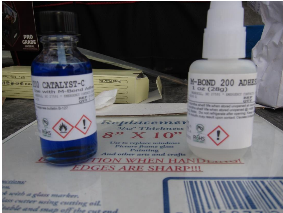
Figure 6.36: The Adhesive and Catalyst for Attaching Strain Gauges
