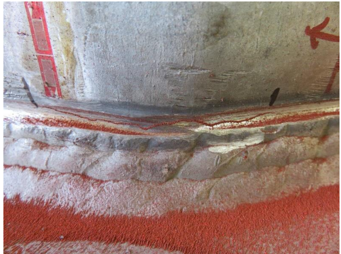
Figure 8.36: Grinding Continued to Remove Magnetic Particle Evidence of the Cracks: Specimen 33-3-12-TX-A3 – Bend 10
