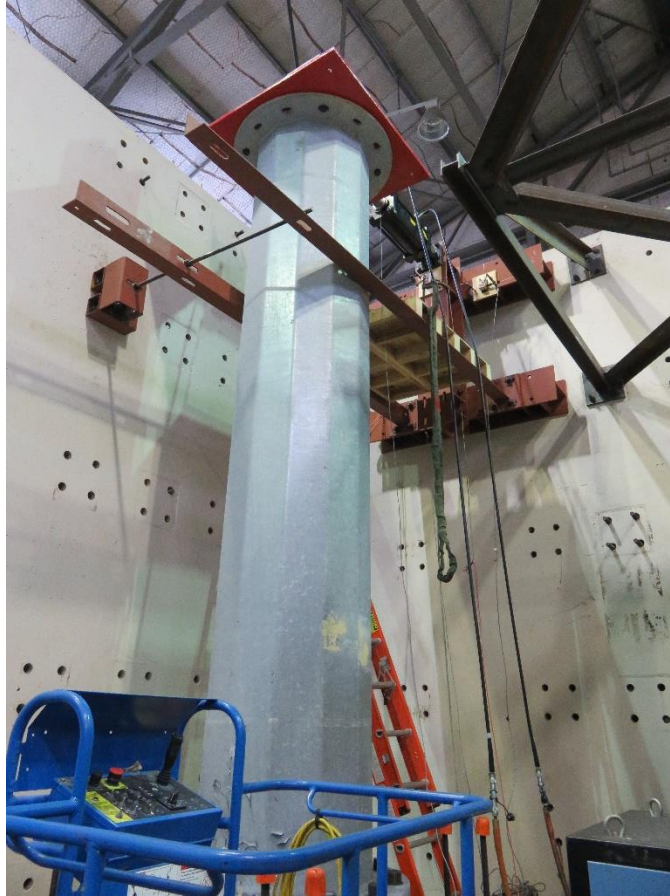
Figure 5.34: Vertical Setup Configured to Perform Ultimate Strength Test on an HMIP Specimen at the Ferguson Structural Engineering Laboratory
