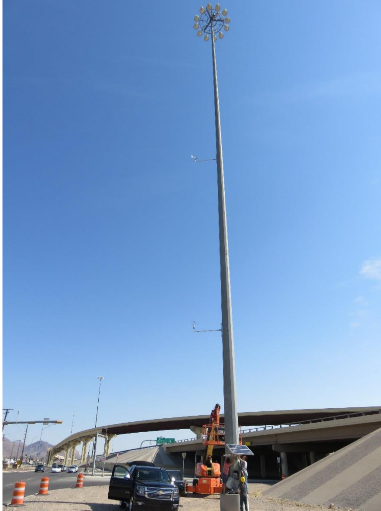
Figure 6.48: Instrumented HMIP in El Paso
