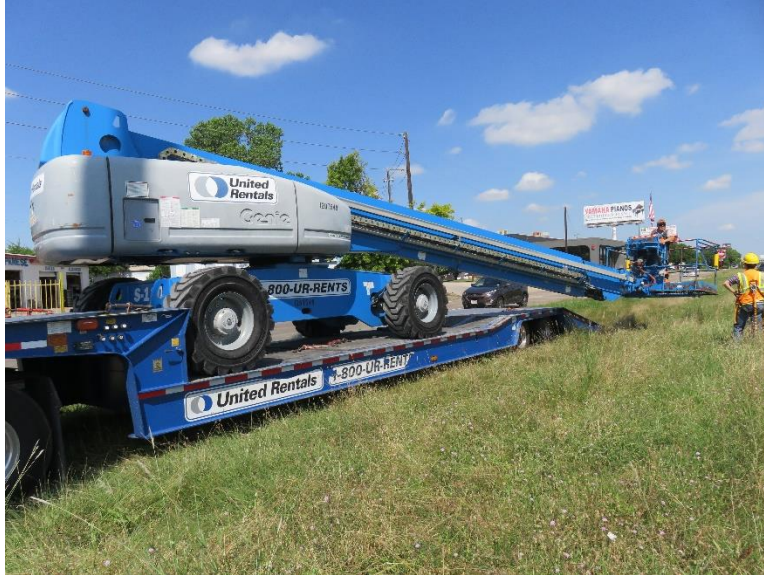
Figure 6.49: Genie Ultra Boom Lift used to Instrument the Selected HMIP in Dallas
