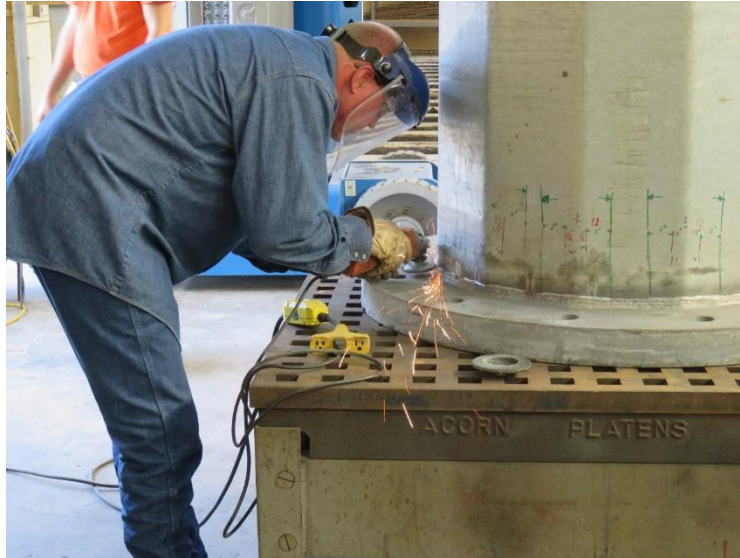
Figure 8.30: Grinding the Shaft Wall Adjacent to the Weld Toe to Remove Cracks – Orientation of the Specimen
