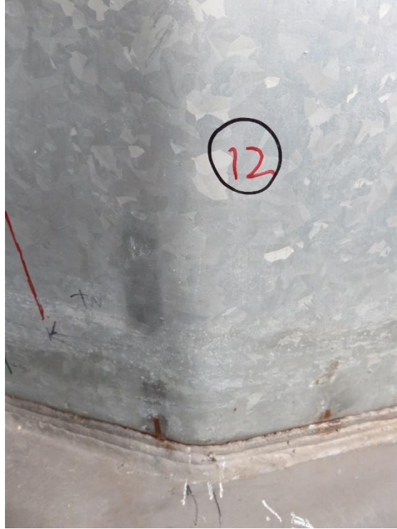
Figure 8.21: State of Cracks: Specimen 33-3-12-TX-A2 – Bend 12
