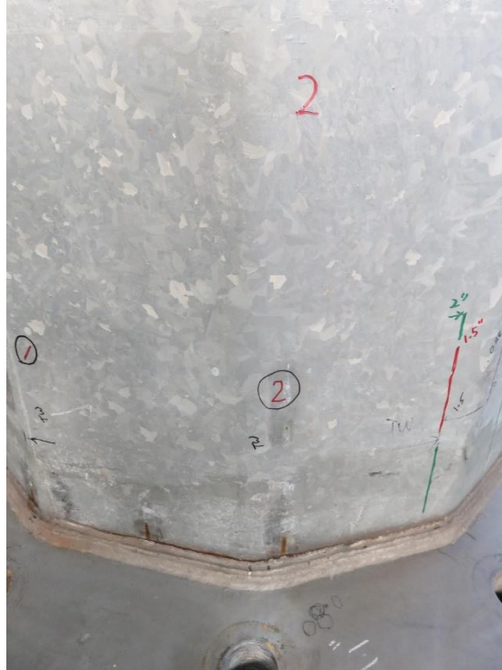
Figure 8.11: State of Cracks: Specimen 33-3-12-TX-A2 – Bend 2
