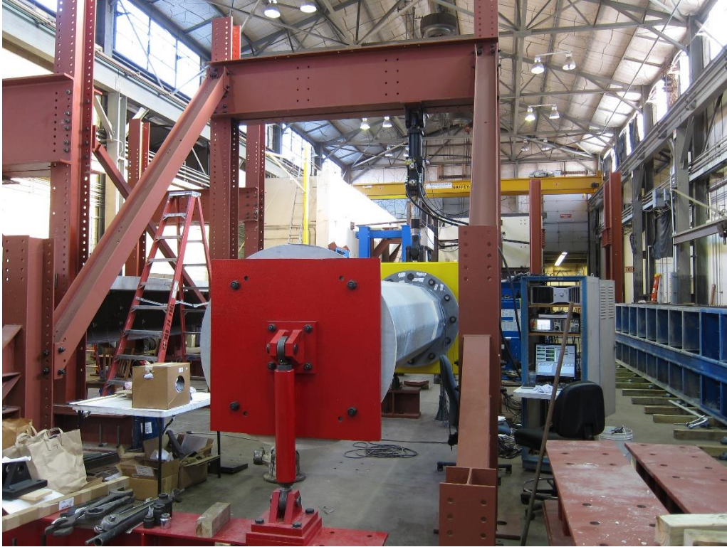
Figure 5.19: Roller Support (2 DOF End) in the Horizontal Fatigue Test Setup
