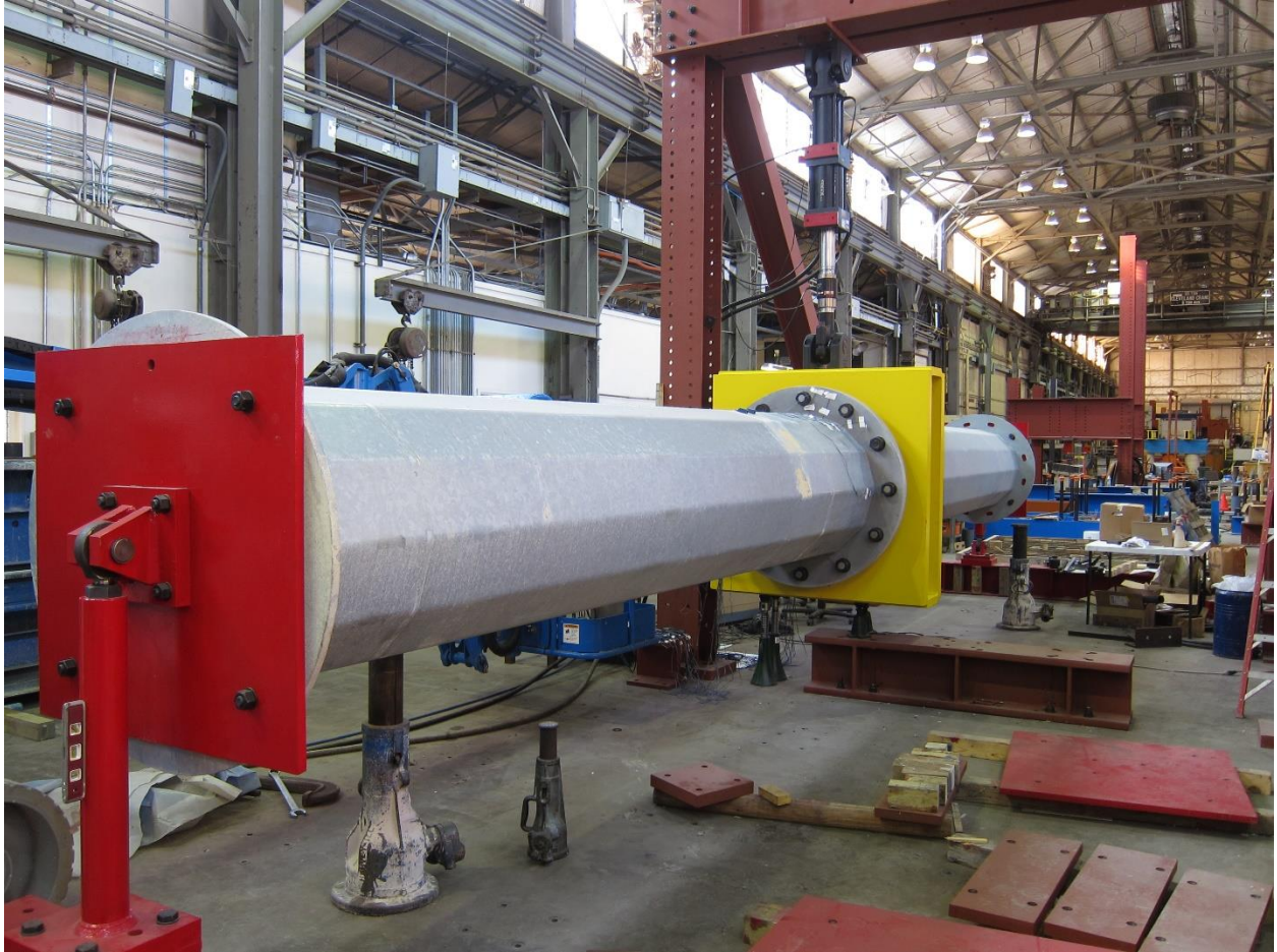
Figure 5.18: Pin Support (1 DOF End) in the Horizontal Fatigue Test Setup
