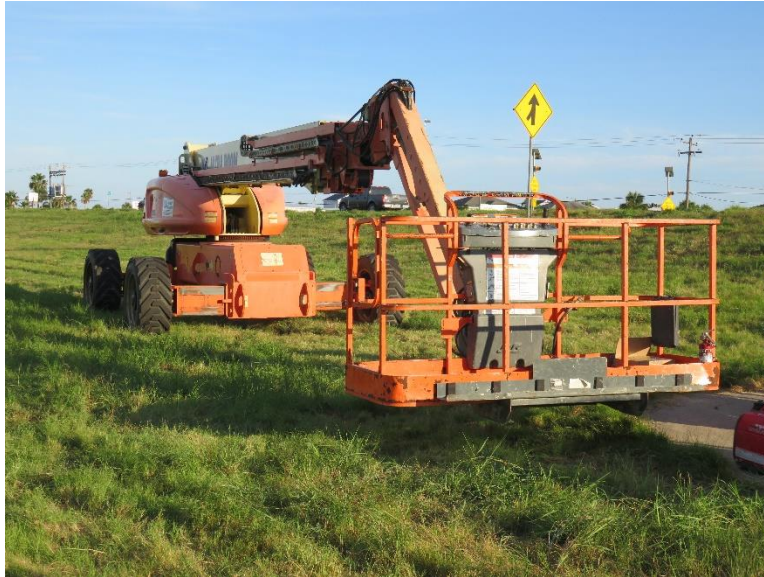
Figure 6.51: JLG Ultra Boom Lift used to Instrument the Selected HMIP in Galveston
