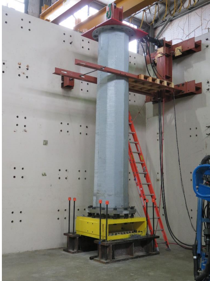
Figure 5.32: Vertical Setup Configured to Perform Fatigue Tests on HMIP Specimens at the Ferguson Structural Engineering Laboratory
