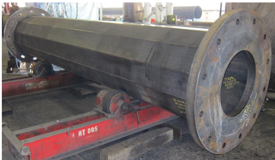
Figure 5.5: HMIP Fatigue Test Specimen of Primary Interest being Fabricated at the Shop
