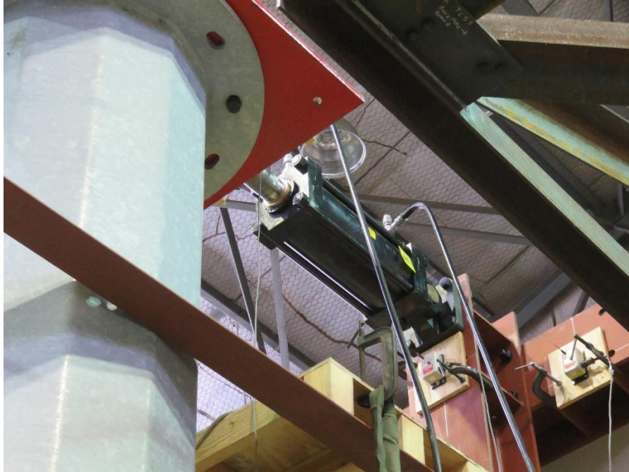
Figure 5.35: An Actuator in the Vertical Setup Used in Ultimate Strength Testing of an HMIP Specimen at the Ferguson Structural Engineering Laboratory
