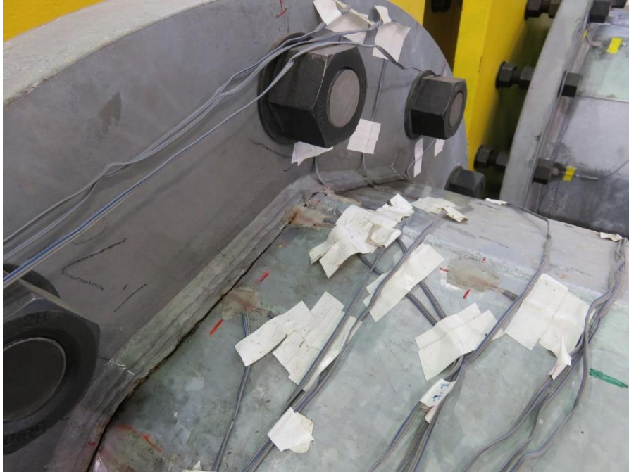
Figure 5.50: Specimen 33-3-12-TX-A1 following the Fatigue Test 1 at the Stress Range of 6 ksi (Fatigue Cracks after 19.4 Million Cycles)
