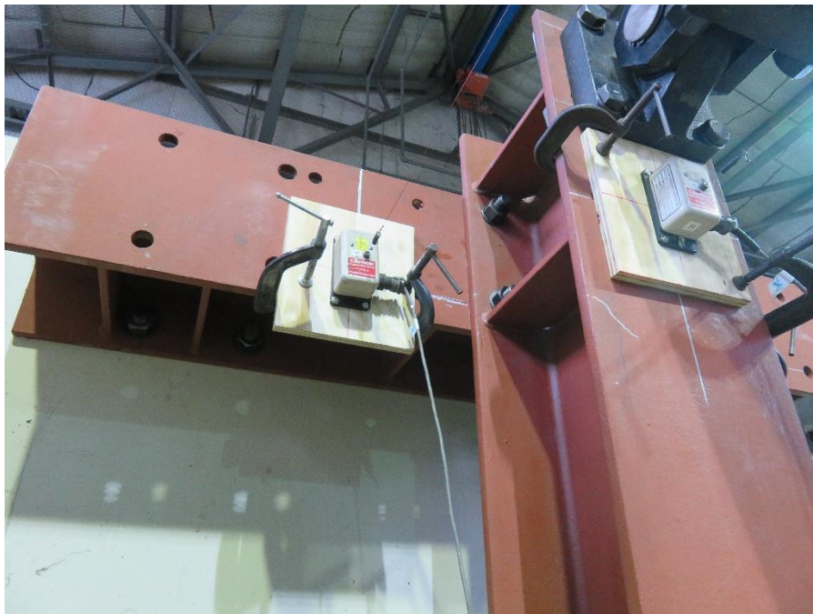
Figure 5.36: String Pods to Measure Lateral Displacements of an HMIP Specimen in the Ultimate Strength Testing at the Ferguson Structural Engineering Laboratory
