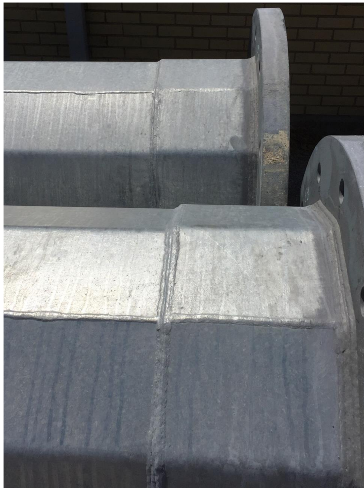
Figure 5.11: A close-up of the Ground Sleeves (External Collars) of the HMIP Specimens of Secondary Interest
