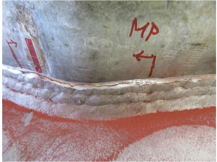
Figure 8.35: Grinding Continued to Remove Magnetic Particle Evidence of the Cracks: Specimen 33-3-12-TX-A3 – Bend 10
