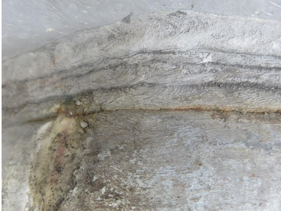
Figure 5.99: Specimen 33-3-12-TXEC-A7 (Bend 4) following the Fatigue Test 8 at the Stress Range of 5 ksi (Fatigue Cracks after 1.8 Million Cycles)
