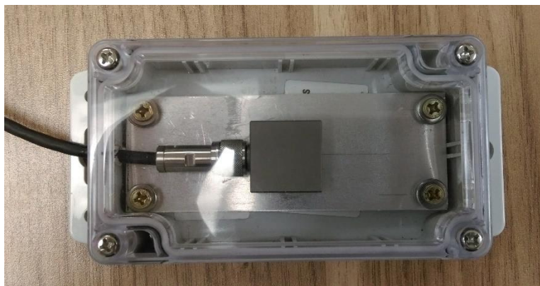
Figure 6.17: Accelerometer shown in a small enclosure
