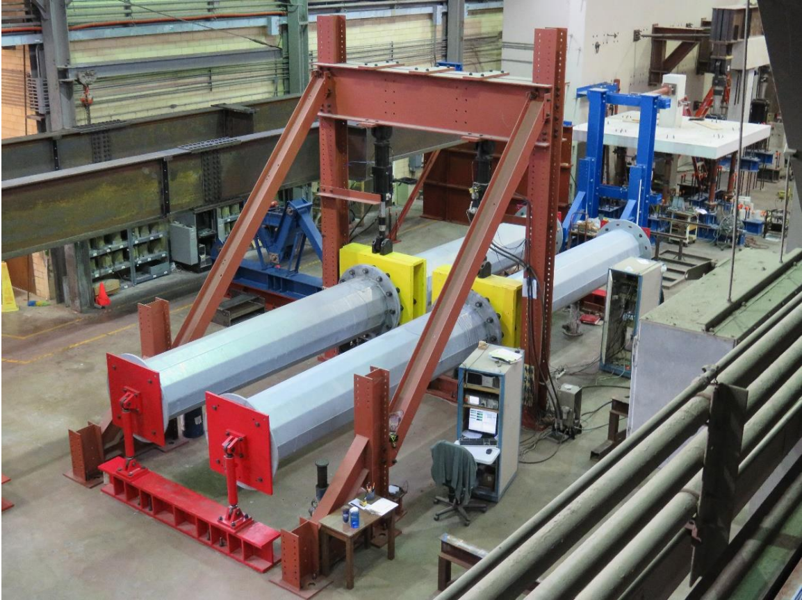
Figure 5.16: Portal Loading Frame Used in Fatigue Testing of HMIP Specimens at the Ferguson Structural Engineering Laboratory
