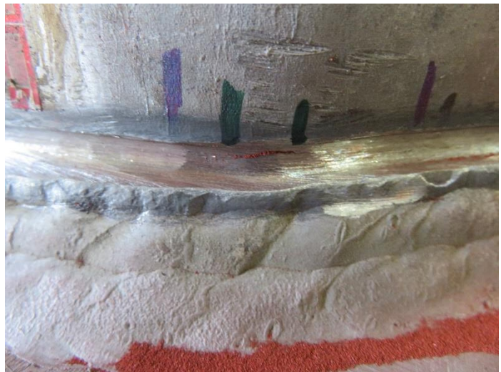
Figure 8.38: Grinding Continued to Remove Magnetic Particle Evidence of the Cracks: Specimen 33-3-12-TX-A3 – Bend 10
