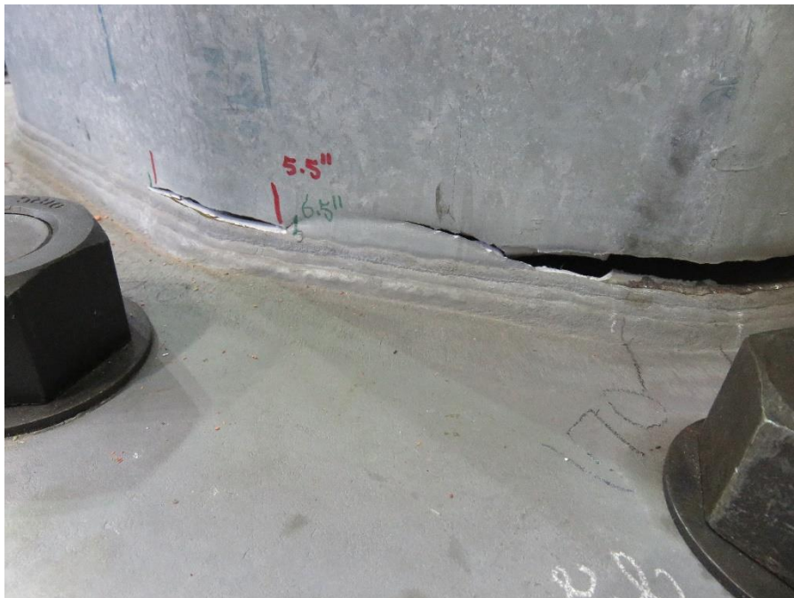
Figure 5.107: Propagation of Cracks from Bends 12 and 11 towards the flat Following the Ultimate Strength Test on the Damaged Specimen 33-3-12-TX-A1
