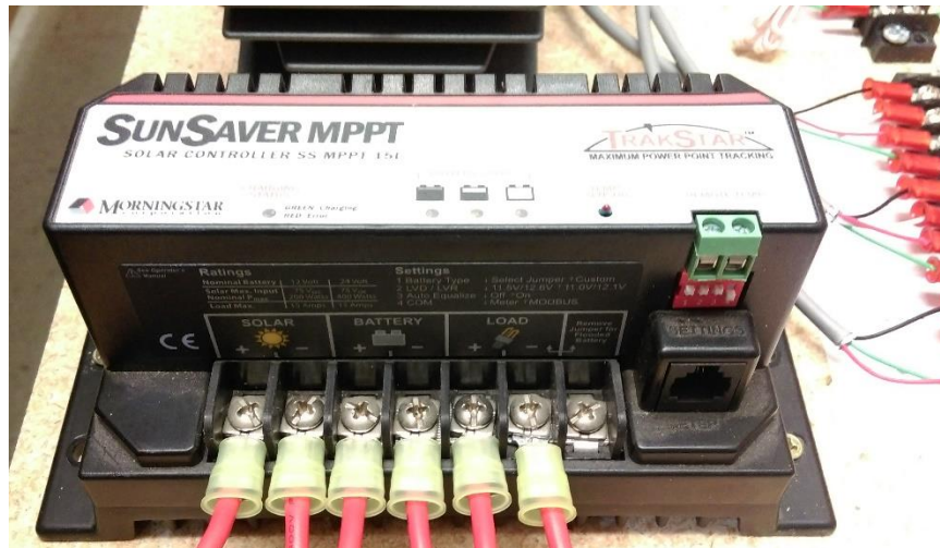
Figure 6.21: MPPT Charge Controller from SunSaver
