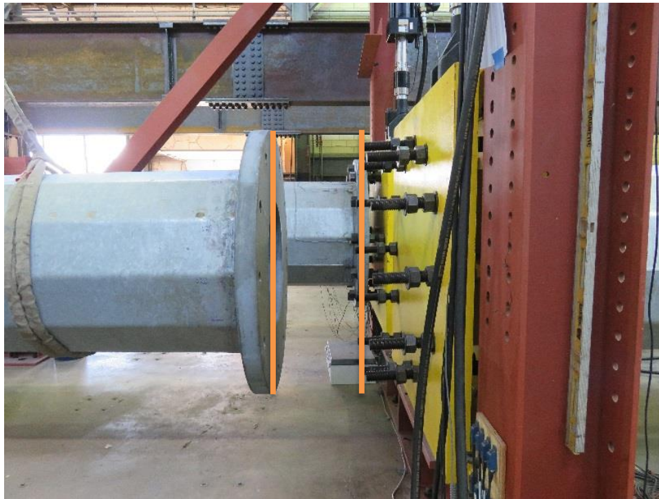
Figure 5.22: Attachment of a "leveled" HMIP specimen to the Load Box.
