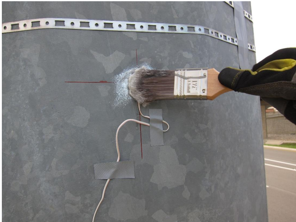
Figure 6.38: Wax to Protect the Strain Gages from Humidity
