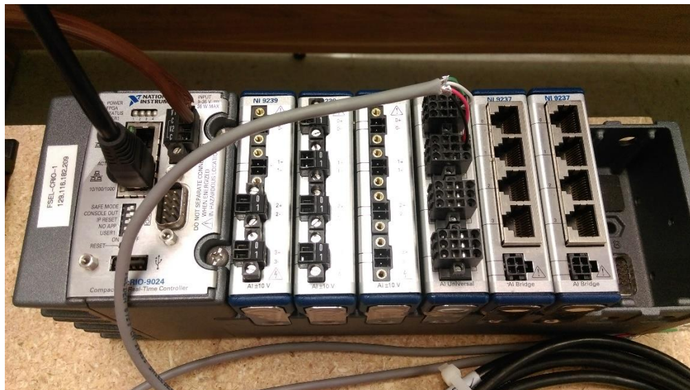
Figure 6.23: NI Compact RIO Data Acquisition System
