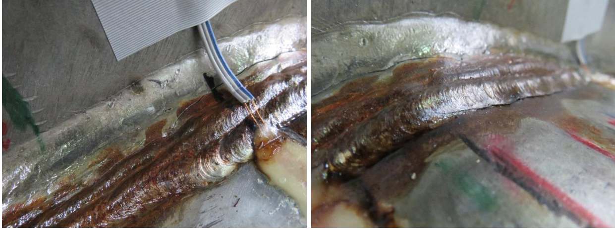
Figure 8.45: Weld-Repaired Specimen 33-3-12-TX-A3 – Bend 10 Following the Fatigue Test: Close-up View
