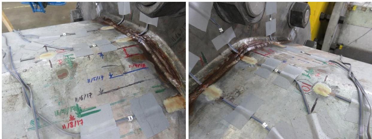
Figure 8.44: Weld-Repaired Specimen 33-3-12-TX-A3 – Bend 10 Following the Fatigue Test: General View
