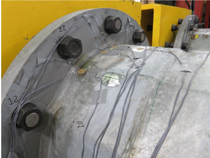
Figure 5.94: Specimen 33-3-12-TXEC-A7 (Bend 10) following the Fatigue Test 7 at the Combined Stress Ranges of 3 ksi and 5 ksi (Fatigue Cracks after 4.2 Million Cycles)
