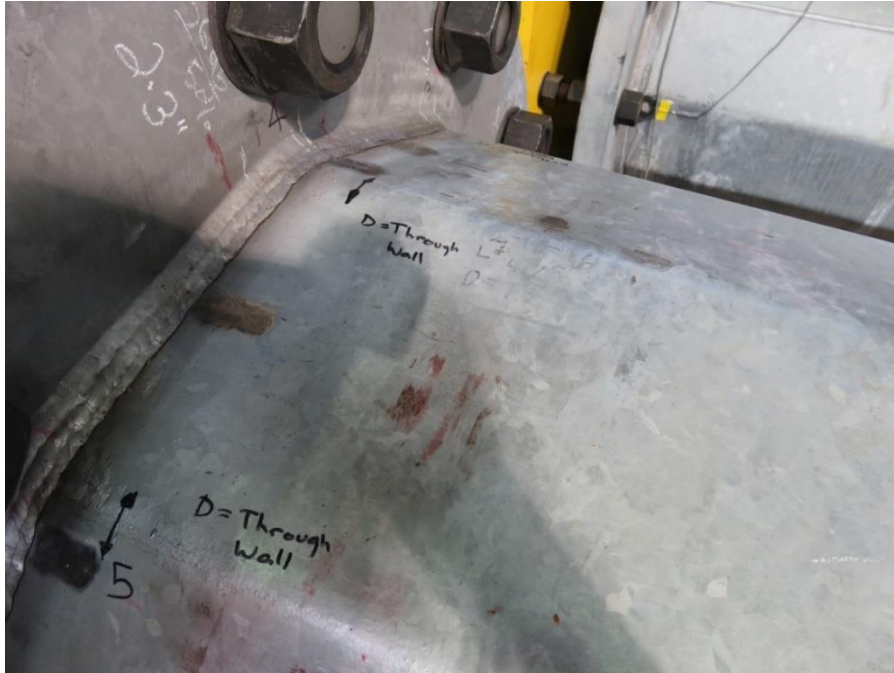
Figure 5.78: Specimen 33-3-12-TX-A3 following the Fatigue Test 4 at the Stress Range of 4 ksi (Fatigue Cracks after 5.5 Million Cycles)
