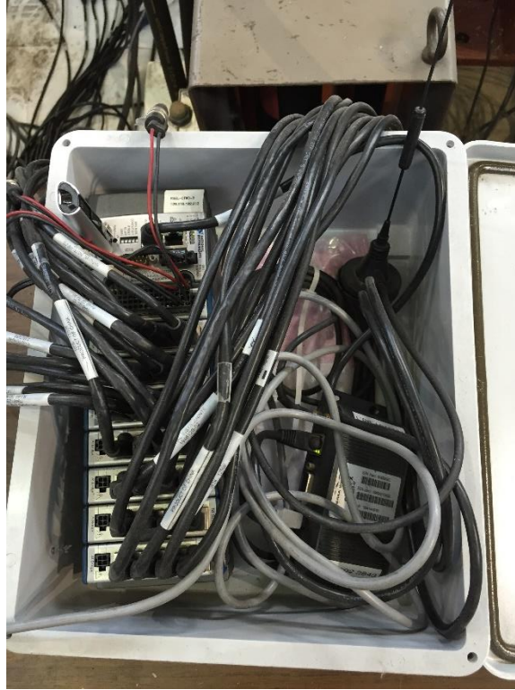
Figure 5.26: NI Compact RIO Data Acquisition System Used to Record Fatigue Test Data
