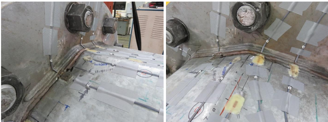
Figure 8.48: Weld-Repaired Specimen 33-3-12-TX-A2 – Bend 8 Following the Fatigue Test: General View
