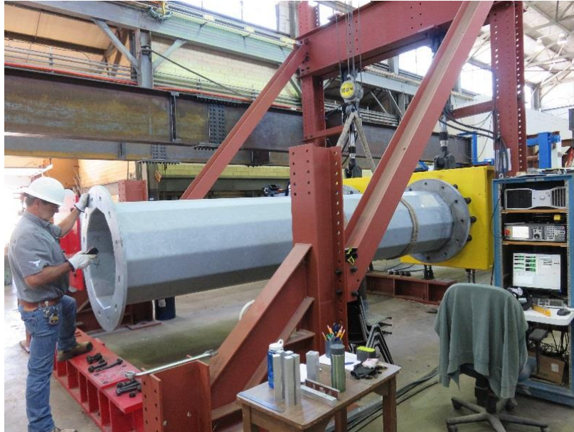
Figure 5.21: Installation of an HMIP Specimen into the Horizontal Fatigue Testing Setup.
