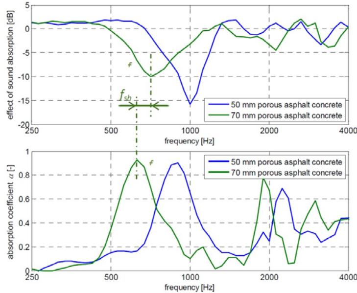
Figure 2.24: Sound absorption effect on noise reduction (Peeters et al., 2010)
