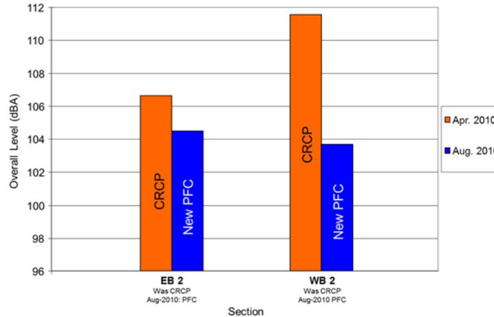
Figure 6.7: Change in noise levels from CRCP to PFC, before (April 2010) and after (August 2010)
