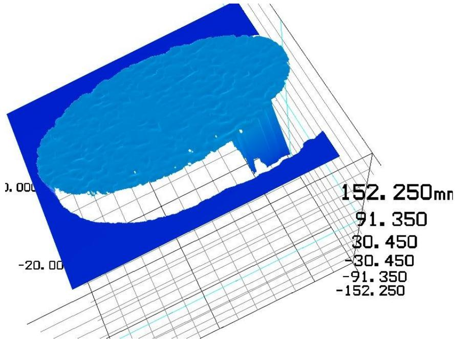
Figure 4.12: LDS scanned TOM surface profile
