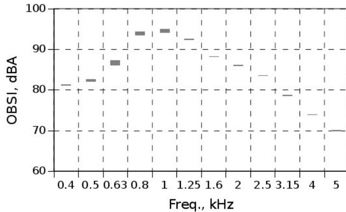
Figure 5.60: OBSI spectra from 1-in. longitudinal tined CRCP at TTI test track
