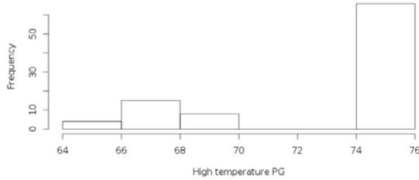
Figure 3.3: Histogram of binder high temperature PG
