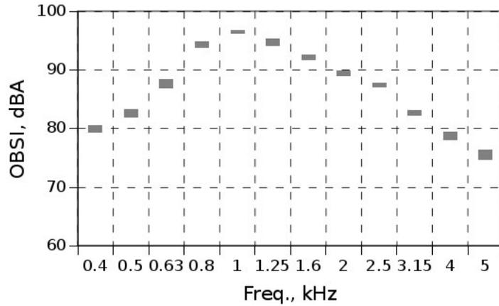
Figure 5.51: OBSI spectra from CRCP on IH 35W (Section 2)
