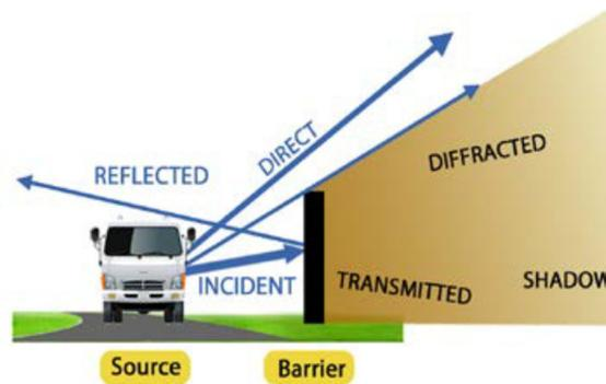
**Figure 5. Acoustic energy and noise barrier (Bowlby 2012)**
