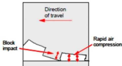
*Figure 2.4: Impacts and shocks noise generating mechanism*
