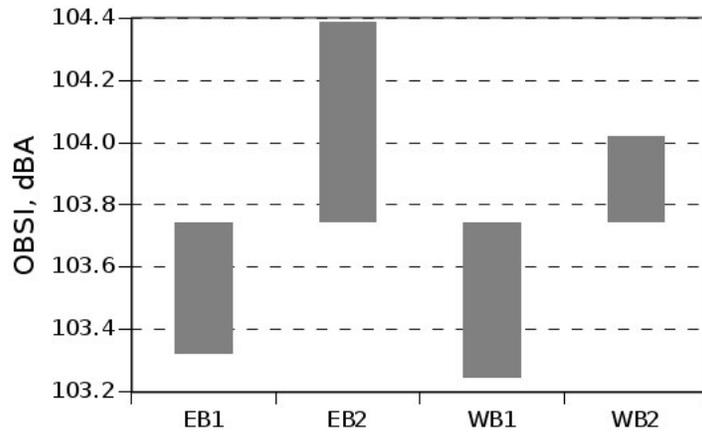
Figure 5.27: OBSI overall levels from PFC2 on IH 30
