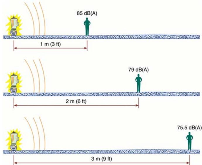
Figure 2.9: Effect of distance on a point noise source (Hanson et al., 2004)
