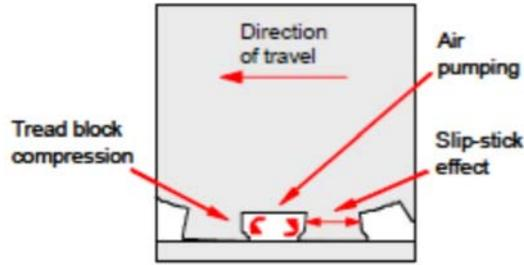
Figure 2.6: Slip-stick effect noise generating mechanism
