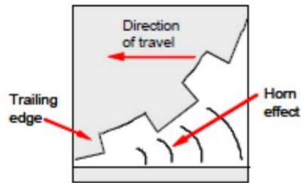
Figure 2.7: Horn-effect amplification mechanism
