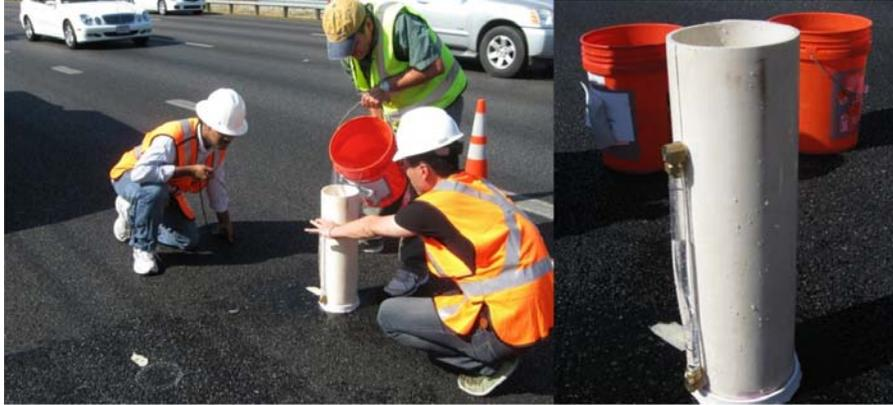
*Figure 5.1: Falling head permeability test*
