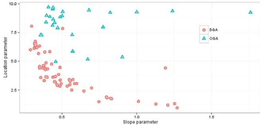
Figure 3.14: Grouping of open- and dense-graded mixtures by parameter
