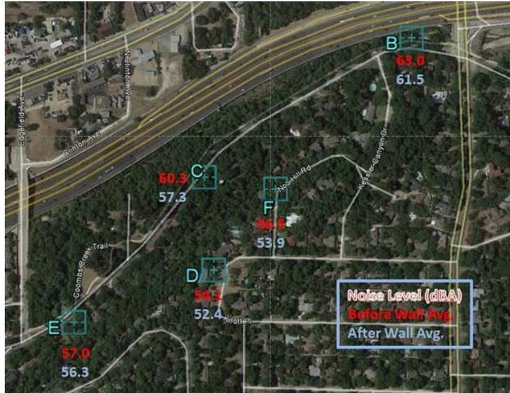
Figure 6.25: Preliminary noise test results
