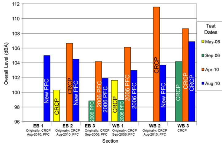
Figure 6.6: OBSI comparison before and after overlay noise levels
