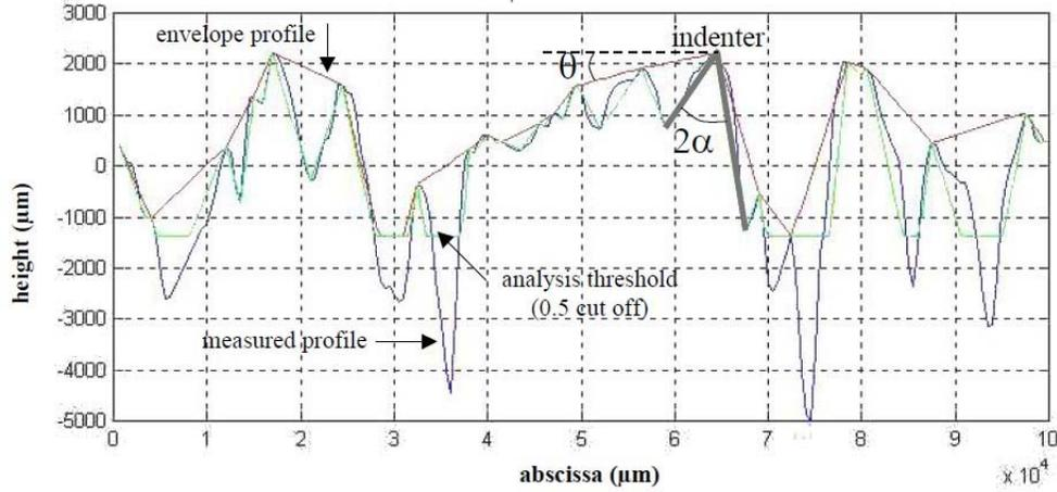
Figure 2.20: Definition of geometric parameters (Anfosso-Lédée and Do, 2002)
