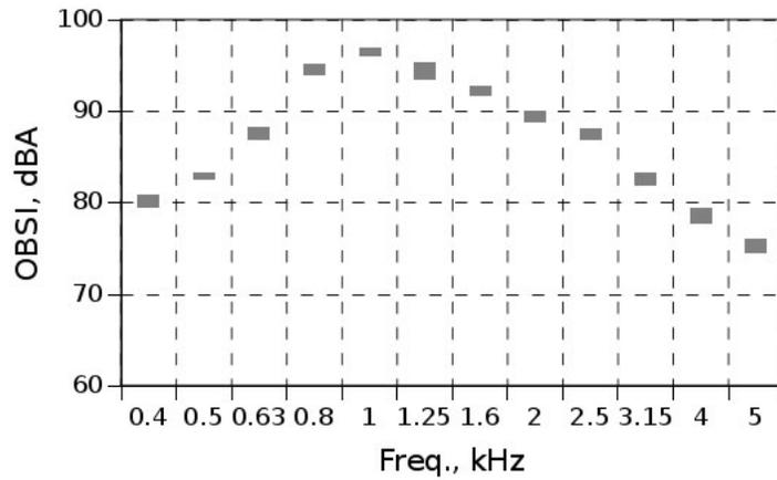
Figure 5.49: OBSI spectra from CRCP on IH 35W (Section 1)
