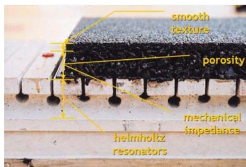
Figure 2.30: Low noise road surface (Kuijpers and van Blokland, 2005)
