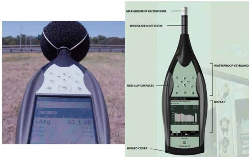
Figure 2.25: Sound pressure level meter
