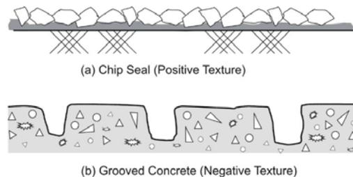
Figure 3.9: Surfaces with positive and negative texture (McGhee and Flintsch, 2003)
