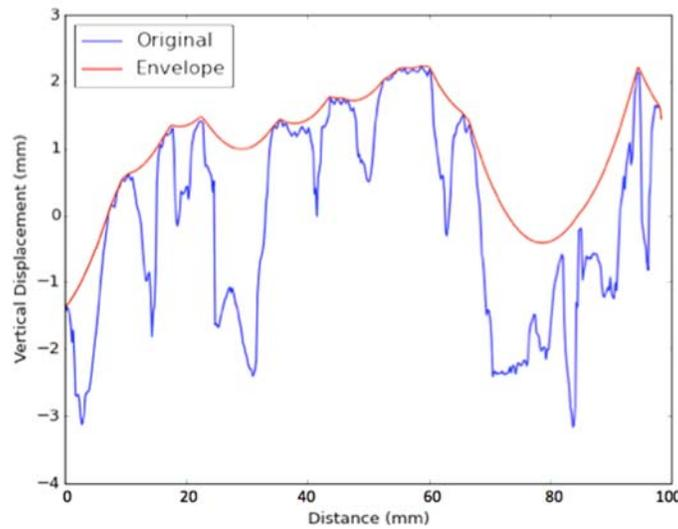
Figure 4.17: Envelope of PFC surface profile
