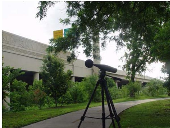
*Figure 6.23: Noise measurement at Coombs Creek Trail Park (Location B) prior to noise barrier installation*
