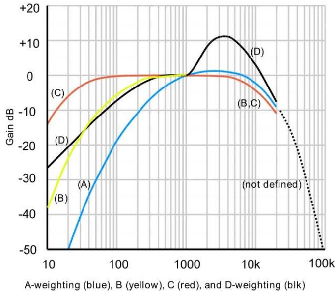
Figure 2.3: A-, B-, C- and D-weightings across the frequency range 10 Hz - 20 kHz
