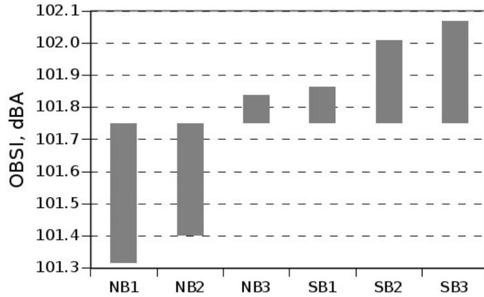
Figure 5.48: OBSI overall levels from CRCP on IH 35W (Section 1)
