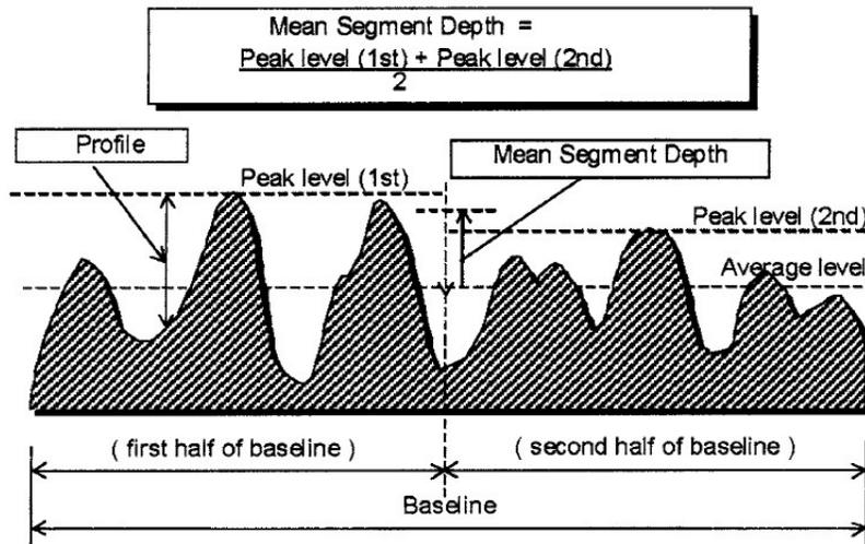
Figure 2.15: Computation of mean segment depth [after ASTM E1845]
