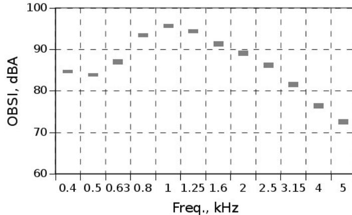
Figure 5.7: OBSI spectra from DGA at TTI test track
