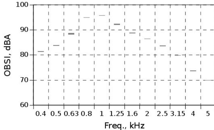
Figure 5.59: OBSI spectra from 1/2-in. transverse tined CRCP at TTI test track
