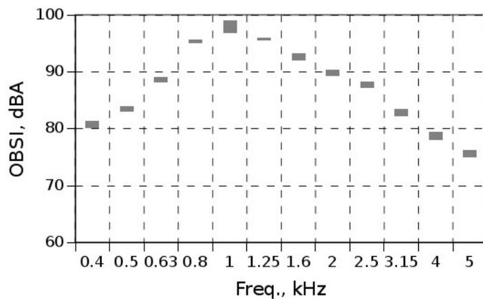
Figure 5.53: OBSI spectra from CRCP on IH 35W (Section 3)
