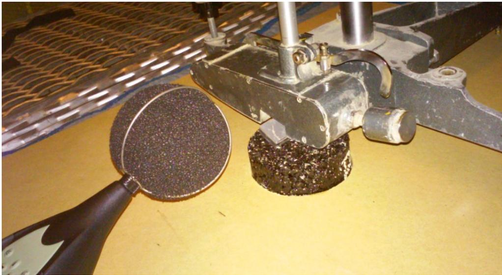
*Figure A.6: BPT testing head in contact with specimen*
