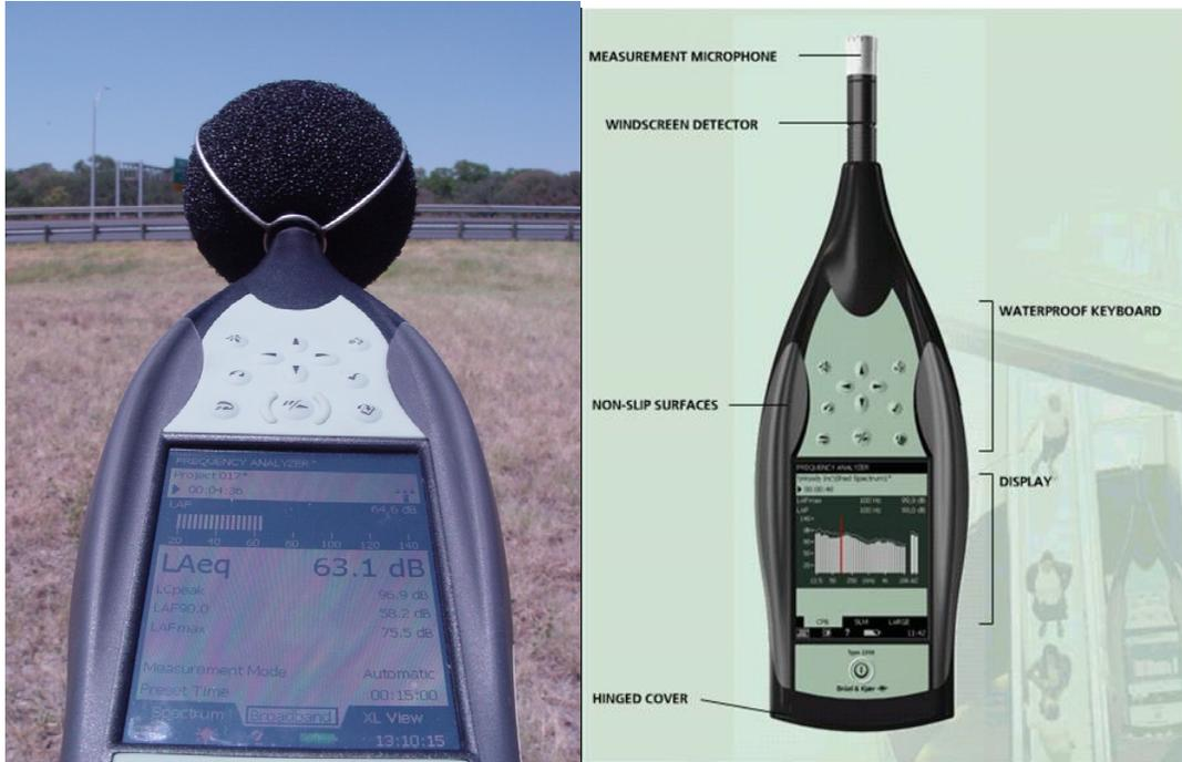
**Figure 1. Sound pressure level meter**
