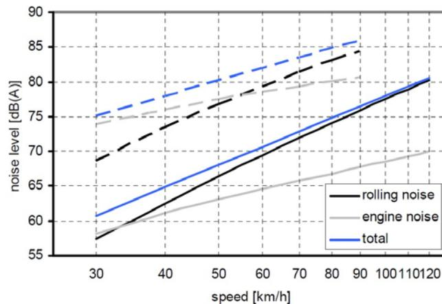
Figure 2.1: Vehicle engine and road noise with speed (van Keulen and Duškov, 2005)
