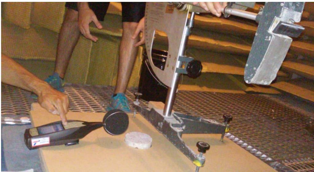
Figure 4.1: BPT noise setup
