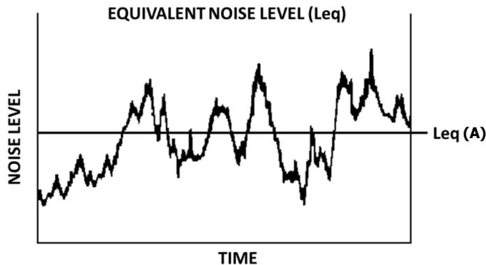
**Figure 2.  $Leq(A)$ : average noise level over a period of time**
