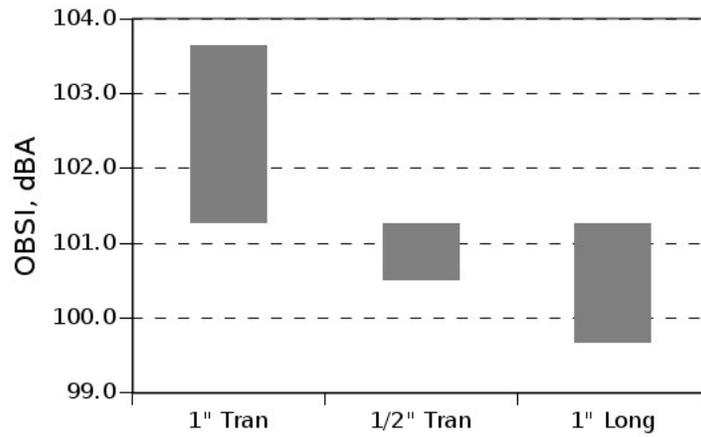
Figure 5.57: OBSI overall levels from CRCP at TTI test track
