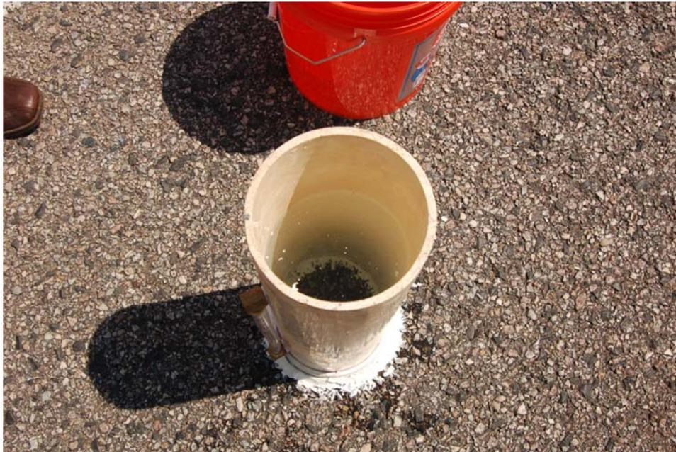
*Figure 5.30: Permeability testing of PFC2 on IH 30*
