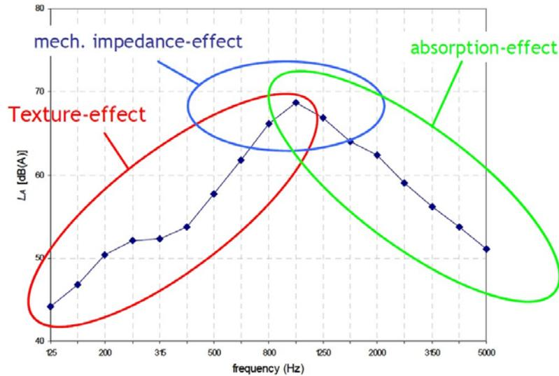
Figure 2.29: Frequency range of road noise influences (Kuijpers and van Blokland, 2005)
