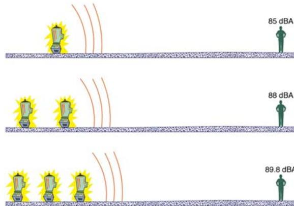
Figure 2.8: Effect of adding noise sources (Hanson et al., 2004)
