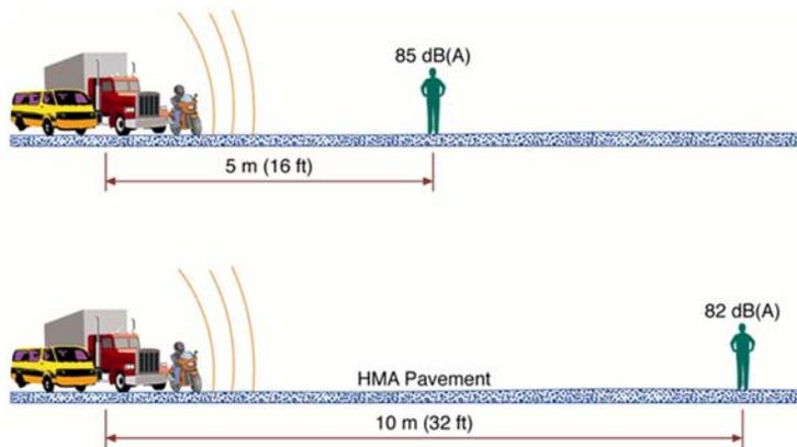
Figure 2.10: Effect of distance on a line noise source over a paved surface (Hanson et al., 2004)
