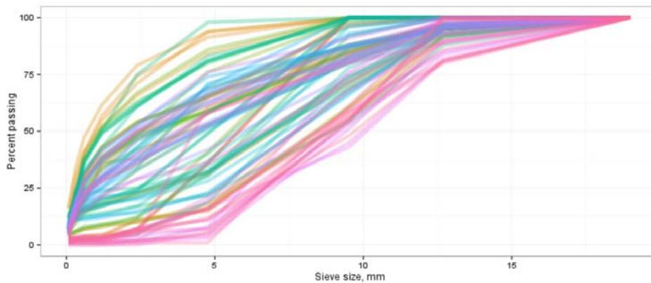
Figure 3.12: Original gradation curves
