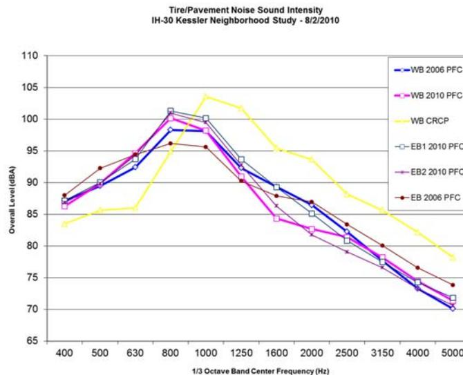
Figure 6.8: Frequency spectra from both PFC overlays and an adjacent CRCP section obtained in 2010
