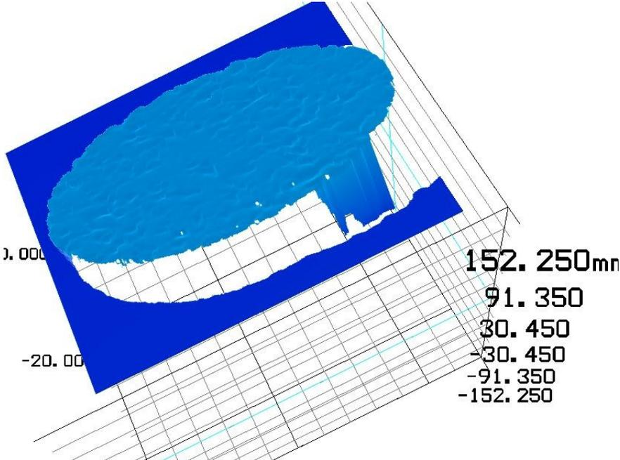
Figure A.3: LDS scanned TOM surface profile
