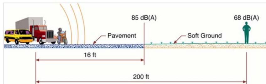
Figure 2.11: Effect of distance on a line noise source over soft ground (Hanson et al., 2004)
