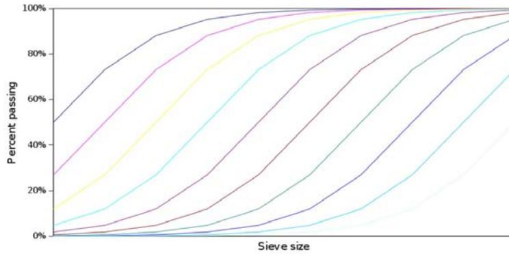
Figure 3.11: Gradations by varying location
