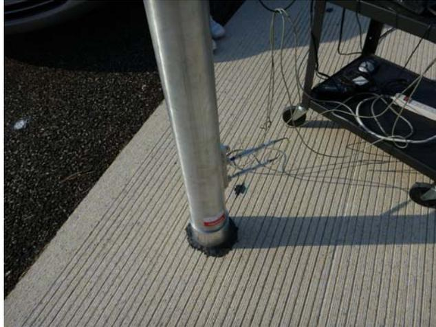
Figure 5.56: 1-in. longitudinal tined surface at TTI test track
