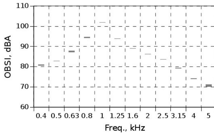
Figure 5.58: OBSI spectra from 1-in. transverse tined CRCP at TTI test track
