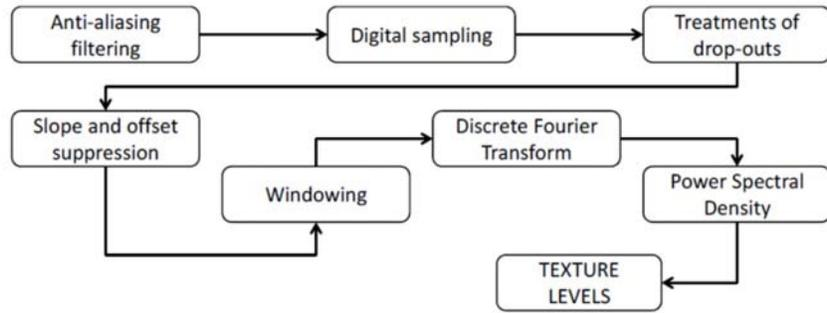
Figure 2.17: Calculation of texture spectrum
