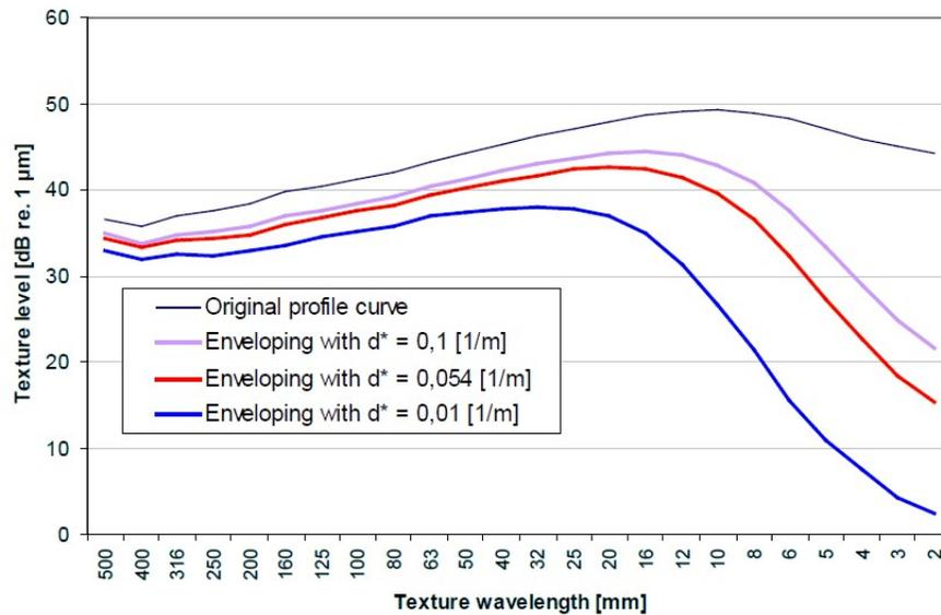
Figure 2.23: Third octave band texture spectra (Sandberg et al., 2011)
