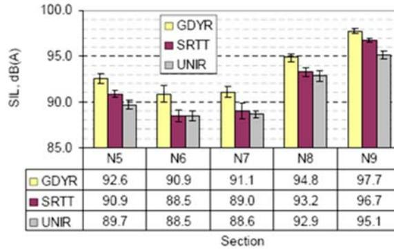
Figure 2.12: Effect of tire type on sound levels (Smit and Waller, 2007a)
