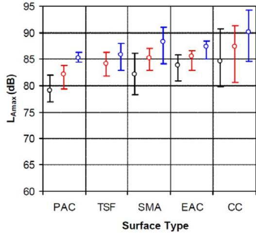
PAC: porous asphalt concrete; TSF: thin surfacings;
