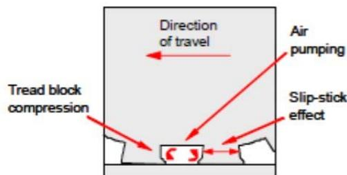
*Figure 2.5: Air pumping noise generating mechanism*
