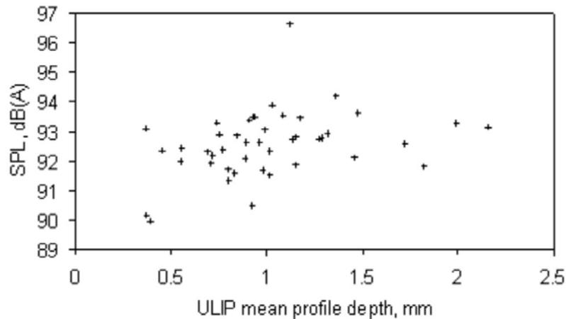
Figure 2.16: Relating road noise level to surface macrotexture
