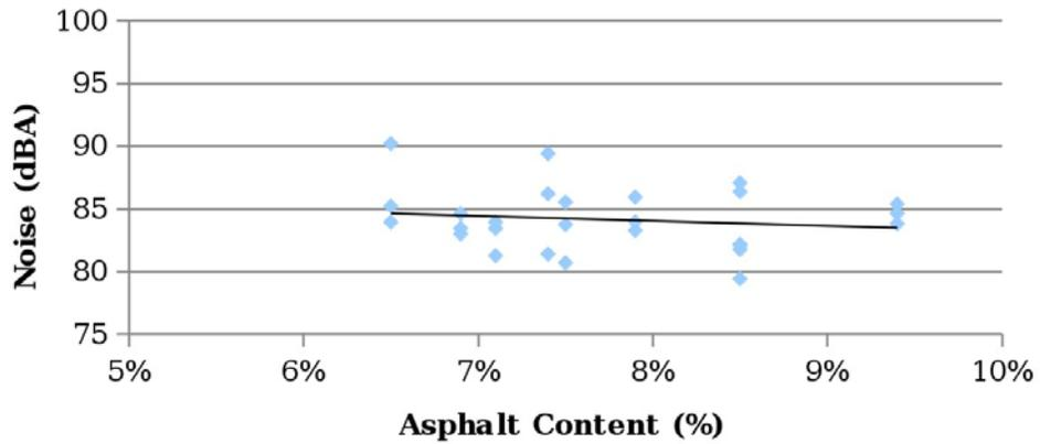
Figure 4.14: Influence of asphalt content on lab noise
