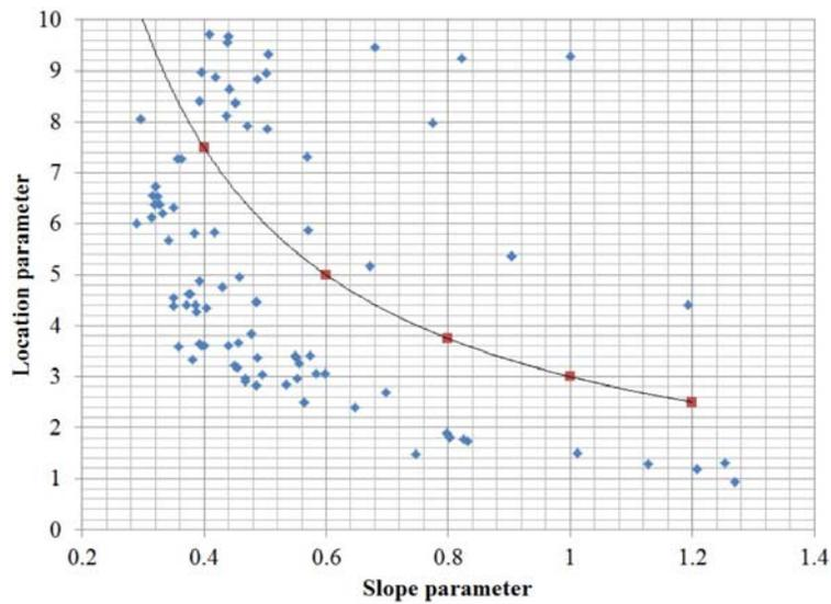
Figure 3.15: Division between open- and dense-graded mixtures
