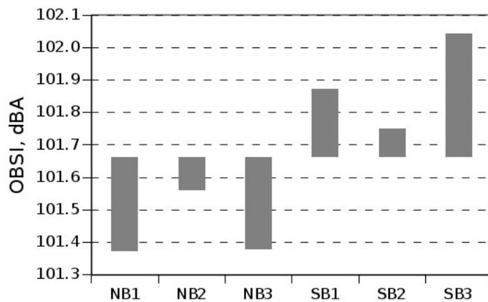
Figure 5.50: OBSI overall levels from CRCP on IH 35W (Section 2)
