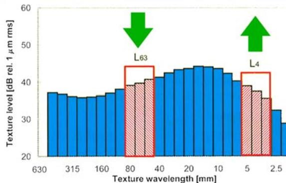
Figure 2.18: Texture spectra parameters
