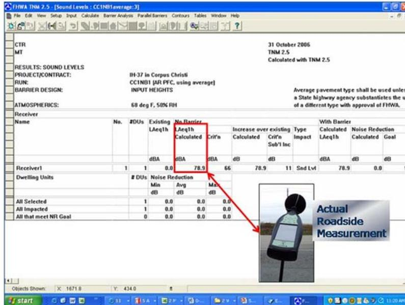
Figure 2.28: Comparison of actual roadside versus predicted noise levels using TNM
