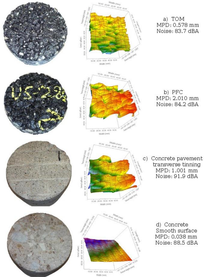
Figure A.9: Preliminary tests results
