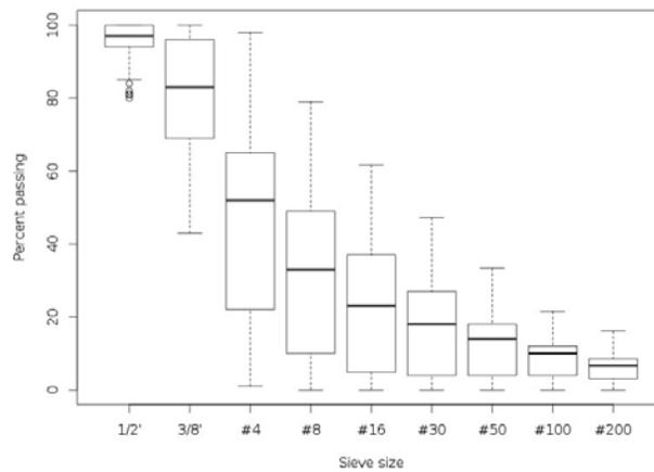
Figure 3.1: Box plot of database gradations
