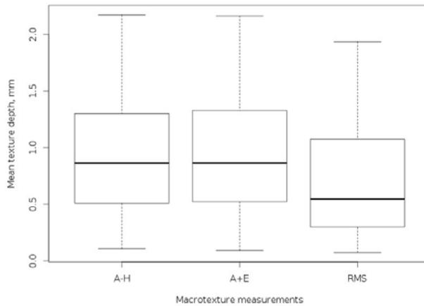
Figure 3.5: Box plot of surface macrotexture
