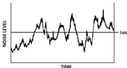
Figure 2.27:  $L_{eq}$ : average noise level over a period of time
