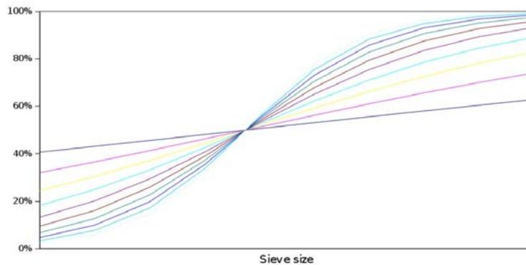
Figure 3.10: Gradations by varying slope
