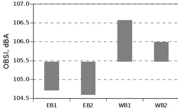
Figure 5.26: OBSI overall levels from PFC1 on IH 30
