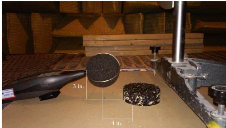
*Figure 4.4: Sound meter position*
