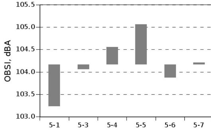
Figure 5.9: OBSI overall levels from PFC on SH6
