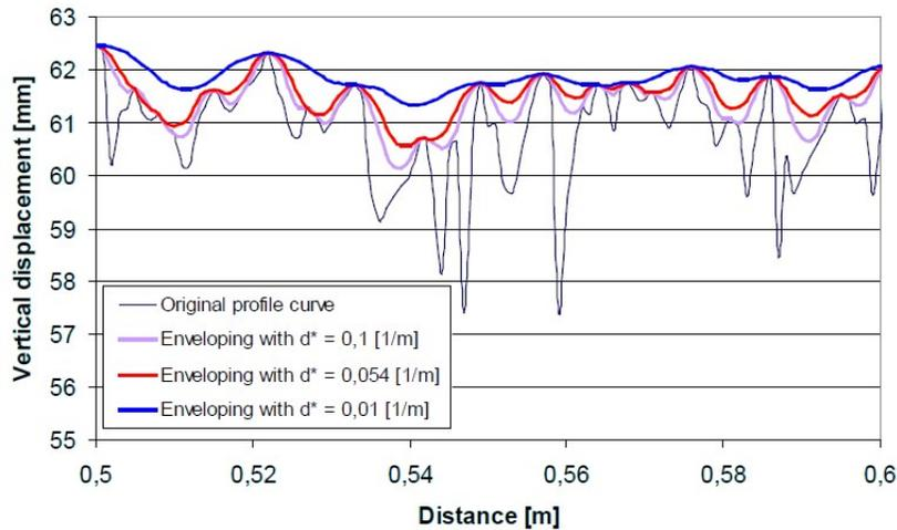
Figure 2.22: Profile envelopes with varying stiffness (Sandberg et al., 2011)
