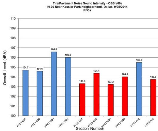
Figure 6.9: Recent OBSI tests on both PFC overlays on IH30 in Dallas (September 2014)
