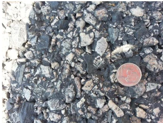
*Figure 5.31: Close-up of PFC1 surface texture*
