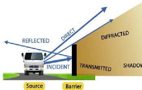
Figure 6.17: Acoustic energy and noise barrier (Bowlby and Knauer, 2012)
