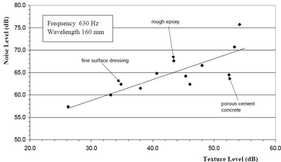
Figure 2.19: Correlation between noise and texture third band octave bands (Anfosso-Lédée and Do, 2002)
