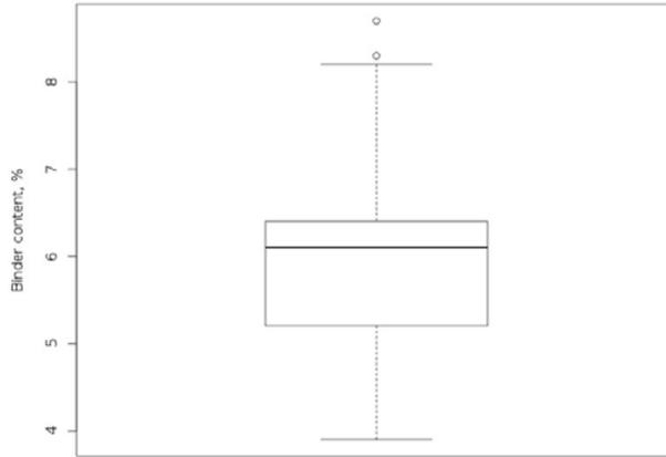
Figure 3.4: Box plot of asphalt binder contents
