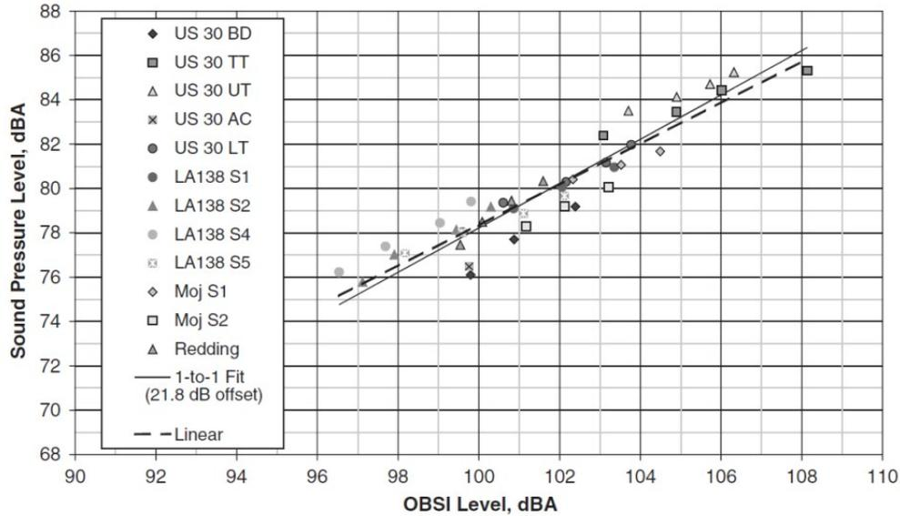
Figure 2.21: Light vehicle pass-by levels at 25 ft versus OBSI for SRTT (Donavan and Lodico, 2009)
