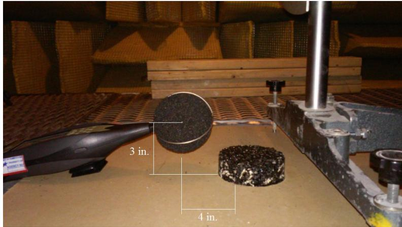
Figure A.8: Sound meter position
