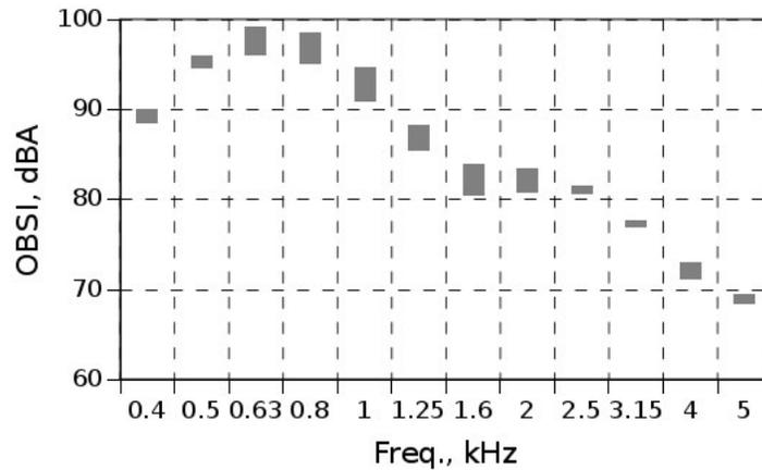
Figure 5.13: OBSI spectra from PFC on SH195
