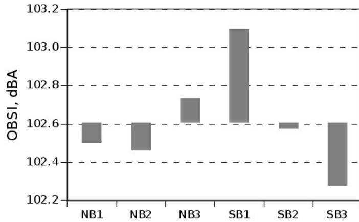
Figure 5.52: OBSI overall levels from CRCP on IH 35W (Section 3)
