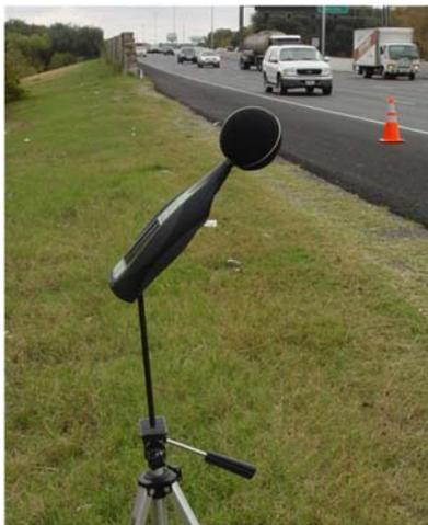
Figure 2.26: SPL meter on a tripod during wayside test
