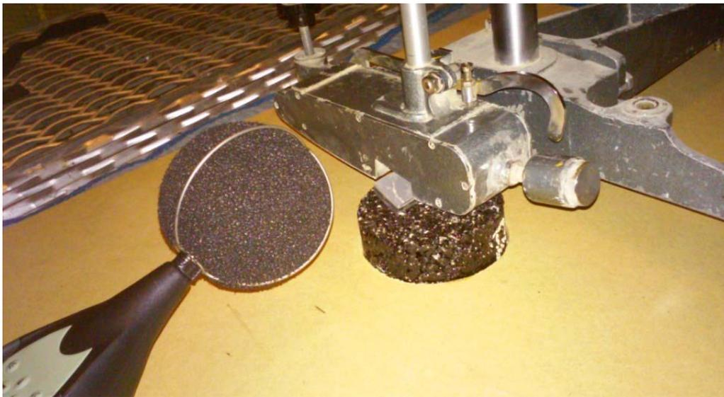
*Figure 4.2: BPT testing head in contact with specimen*
