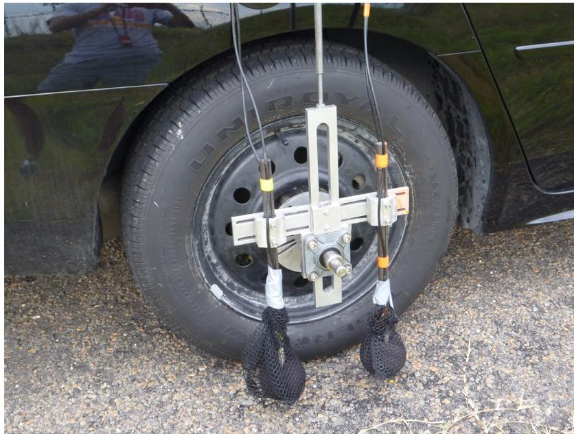
**Figure 4. OBSI test probe**
