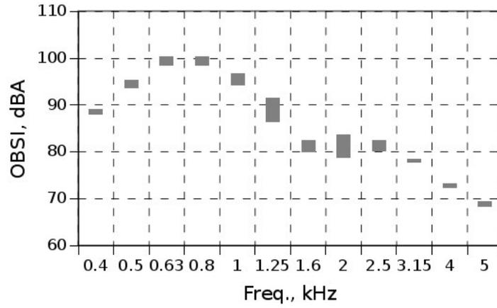
Figure 5.10: OBSI spectra from PFC on SH6
