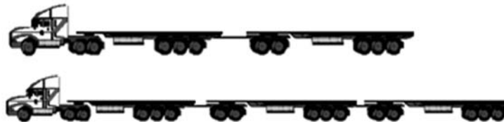
Figure 2.11 Australian double road train at 36.5m long (79.0t) and triple road train at 53.5m long (115.5t)
