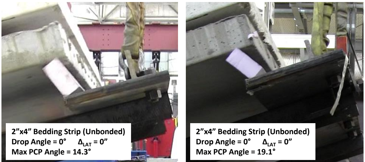
Figure 3.12: Inclined PCP Experimental Tests with 2"x4" Bedding Strips
