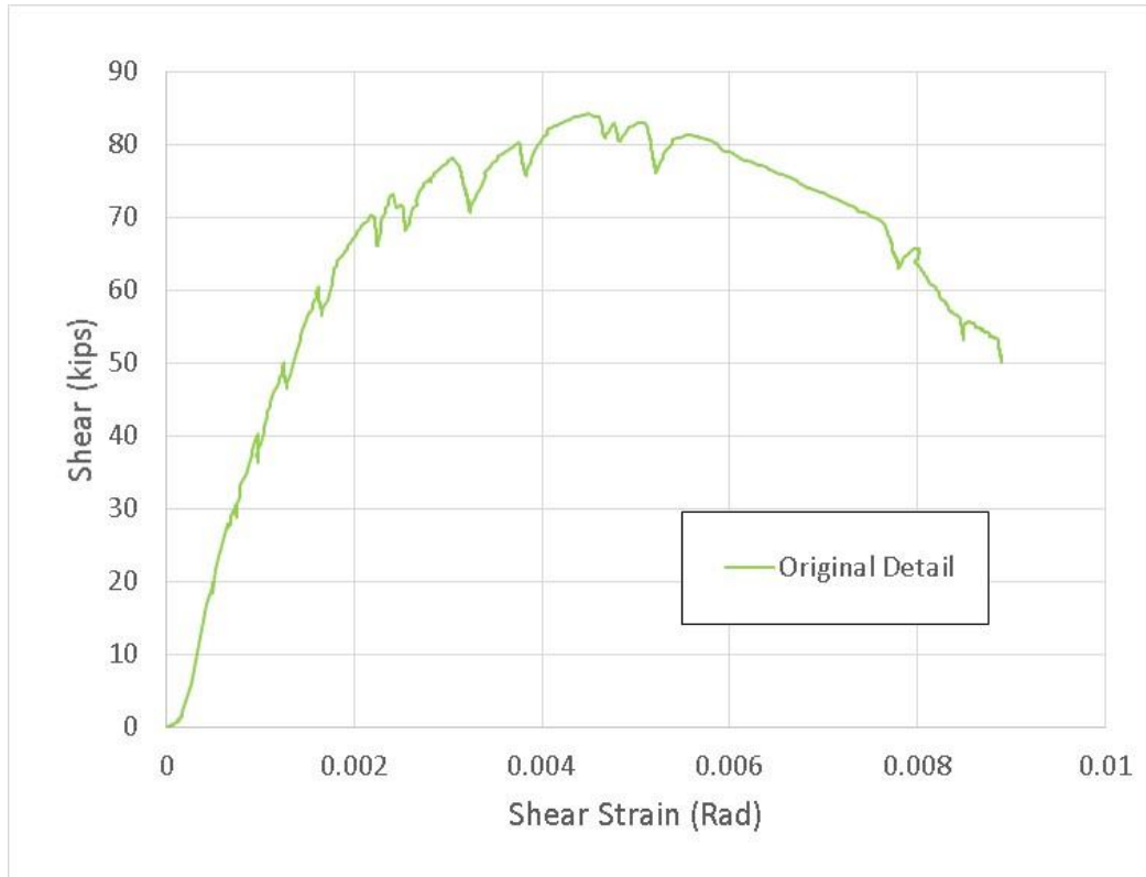
Figure 7.33 Shear Force vs Shear Strain for Original Detail Specimen
