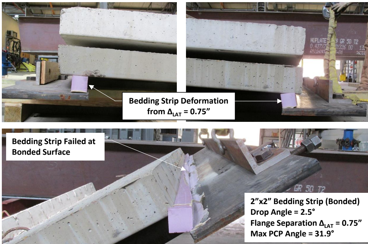
Figure 3.10: Inclined PCP Experimental Tests with 2"x2" Bedding Strips (Bonded)
