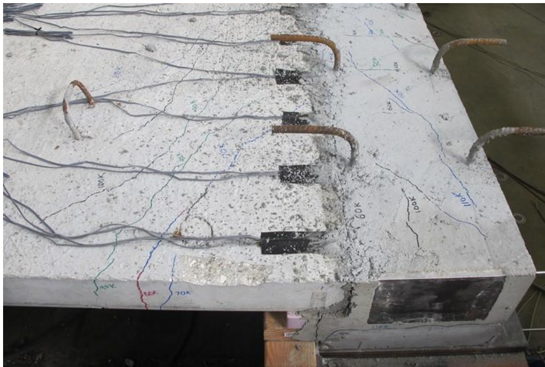
Figure 7.46 Even Distribution of Cracking in Precast Panel of 6" Reinforcement Spacing Detail at 110 kips
