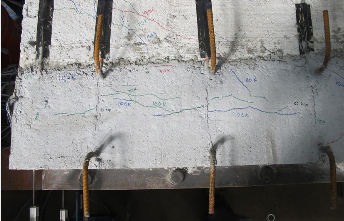
Figure 7.39 Reduced Splitting in Closure Pour at 113 Kips of Shear
