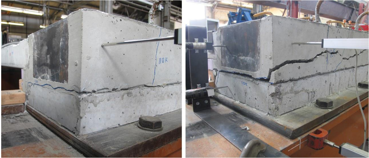
Figure 7.47 Initiation of Closure Pour to Girder Interface Crack at 110 kips and Failure at 114 kips (6" Reinforcement Spacing Specimen)
