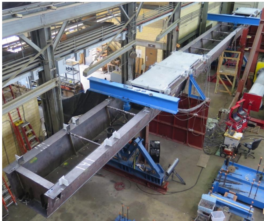
Figure 6.34 Tub Girder Experimental Test Setup – Overhang – 3 PCPs
