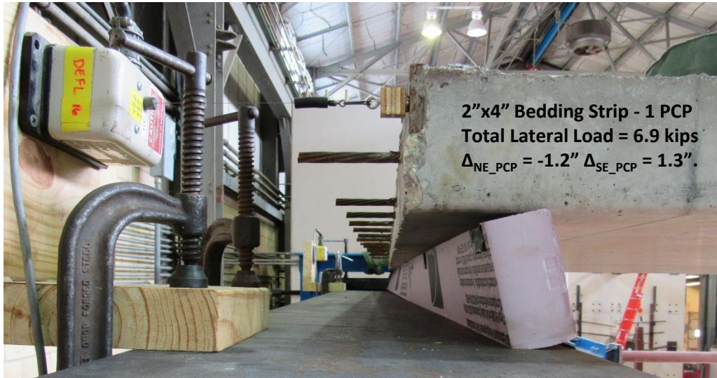
Figure 3.22: Bedding Strip Deformation using Twin I-Girder Test
