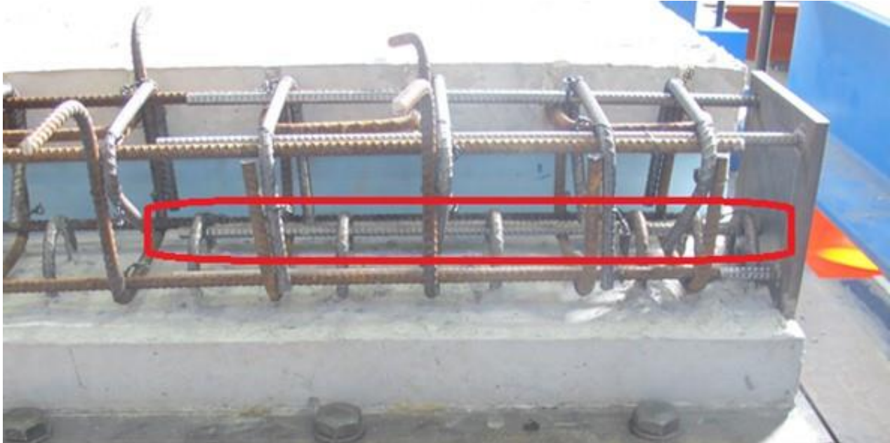
Figure 7.25 Additional Reinforcement to Improve Engagement of R-Bars (Photo)
