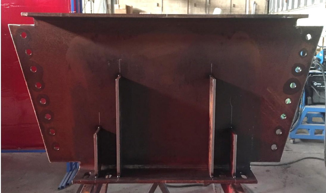
Figure 6.7 Diaphragm at North Support for Overhang Tests
