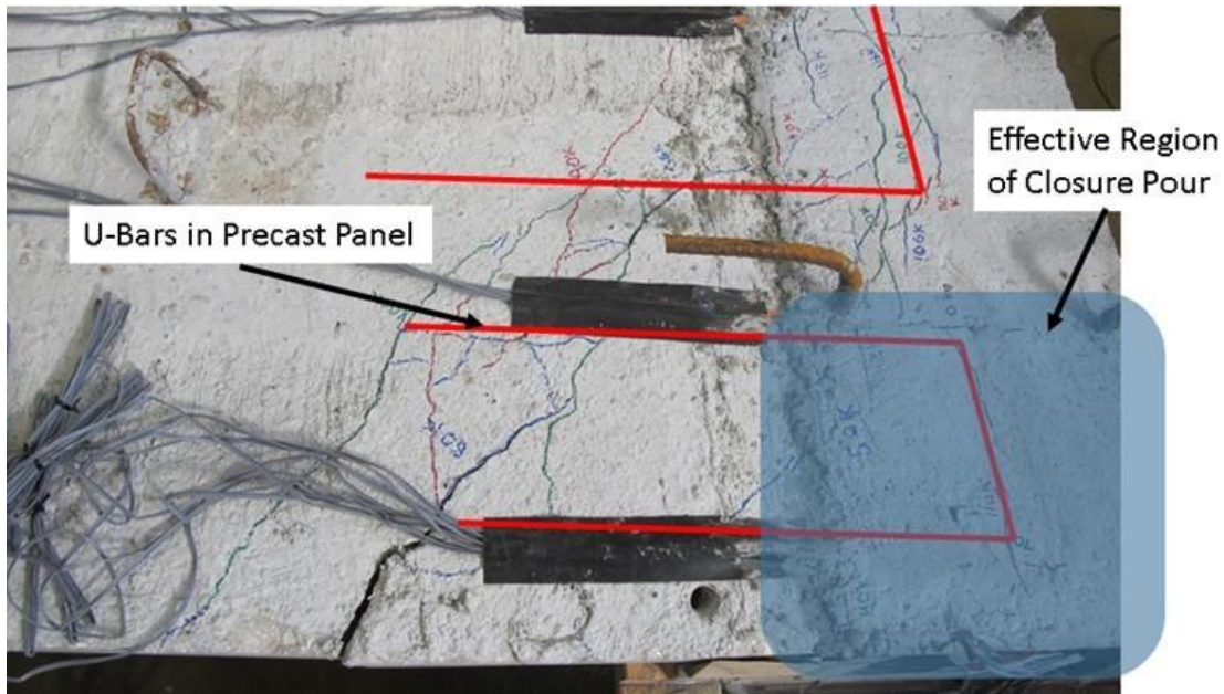
Figure 7.44 Concentration of Strength in Closure Pour Leading to Overload of U-bar and Premature Failure of Precast Panel
