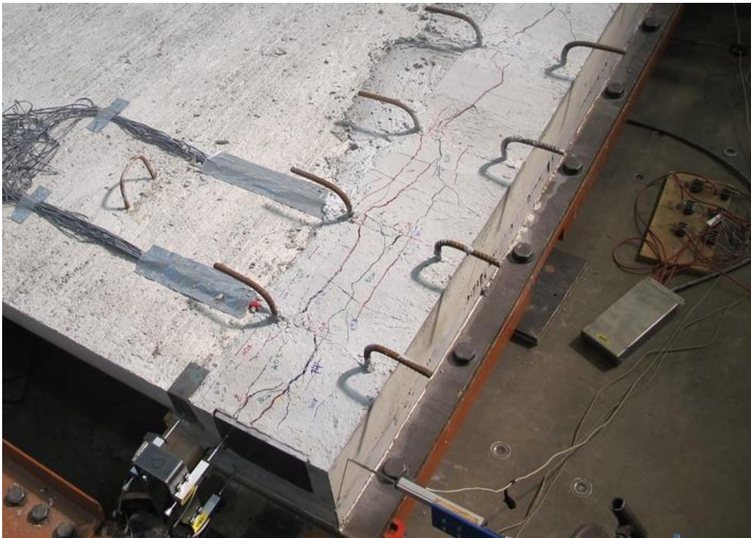
Figure 7.35 Cracking of Cap Plate Specimen at Failure
