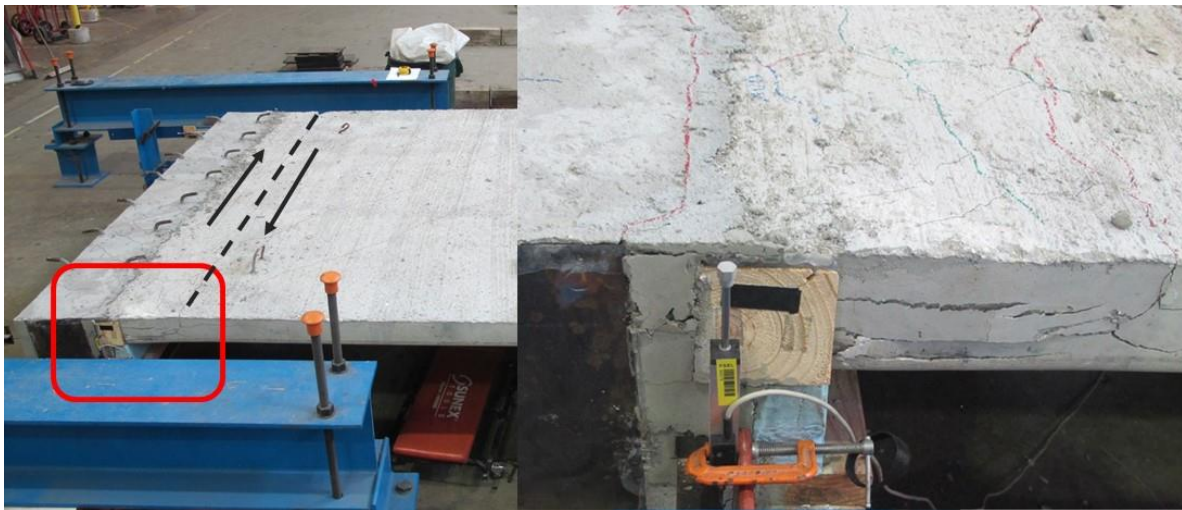
Figure 7.55 Beginnings of Side Face Blowout at South-most Tendon due to Shear Slip of Precast Panel
