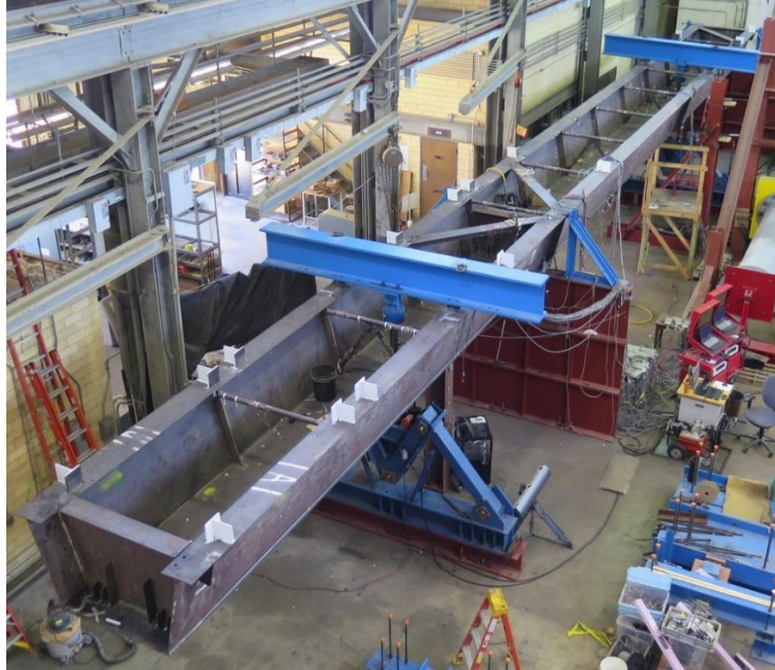
Figure 6.33 Tub Girder Experimental Test Setup – Overhang – 3 DIAGs
