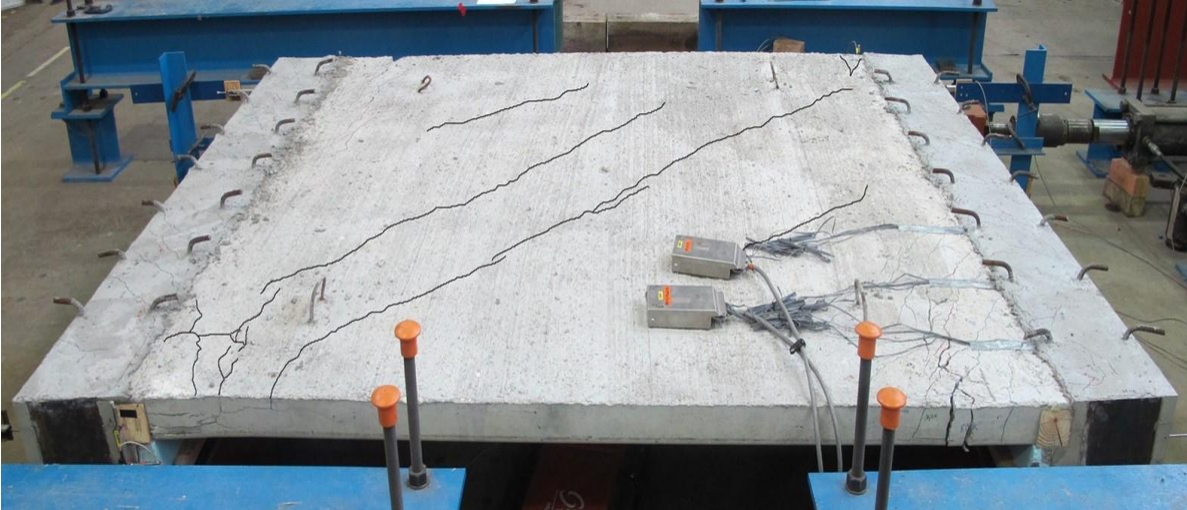
Figure 7.53 Full-Length Diagonal PCP Cracks
