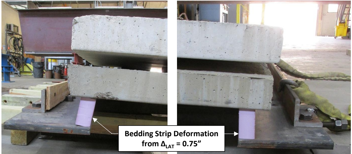
Figure 3.11: Flange Separation with 2"x4" Unbonded Bedding Strips
