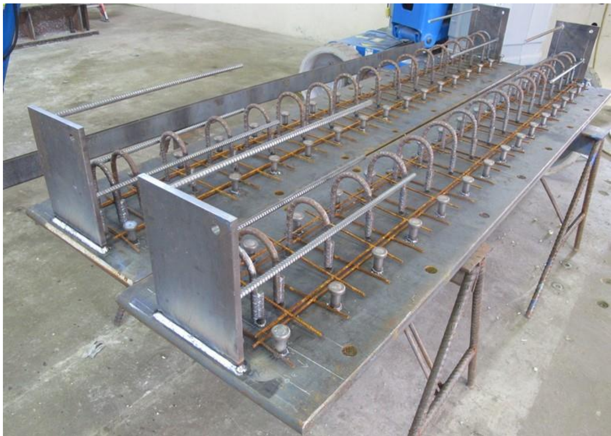
Figure 7.21 Cap Plate Welded to Steel Base Plate
