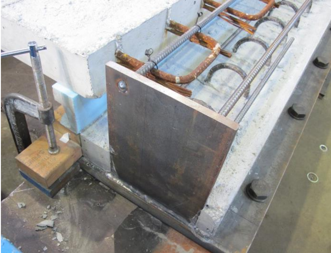
Figure 7.22 Top Inside Rebar Plug Welded to Cap Plate
