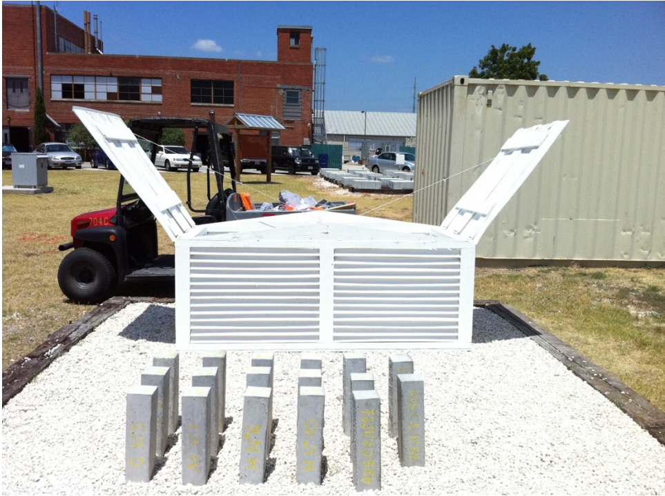
Figure 6-160: Carbonation exposure site at UT Austin with shelter (Stevenson Screen)
