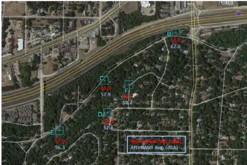
Figure 6.1: Site 1 average noise measurements, before and after noise wall installation
