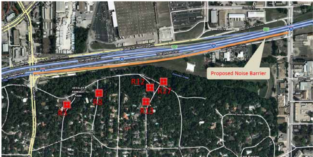
Figure 5.21: Site 2 noise measurement locations
