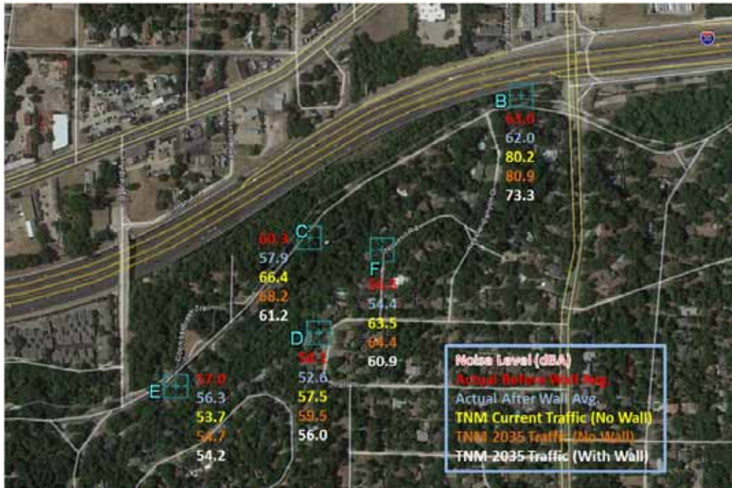
Figure 6.2: Site 1 average noise measurements, before and after noise wall installation, compared with TNM predictions
