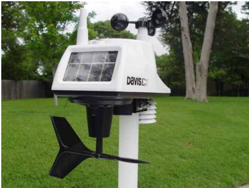
Figure 5.3: Davis Instruments portable weather station, showing the ISS
