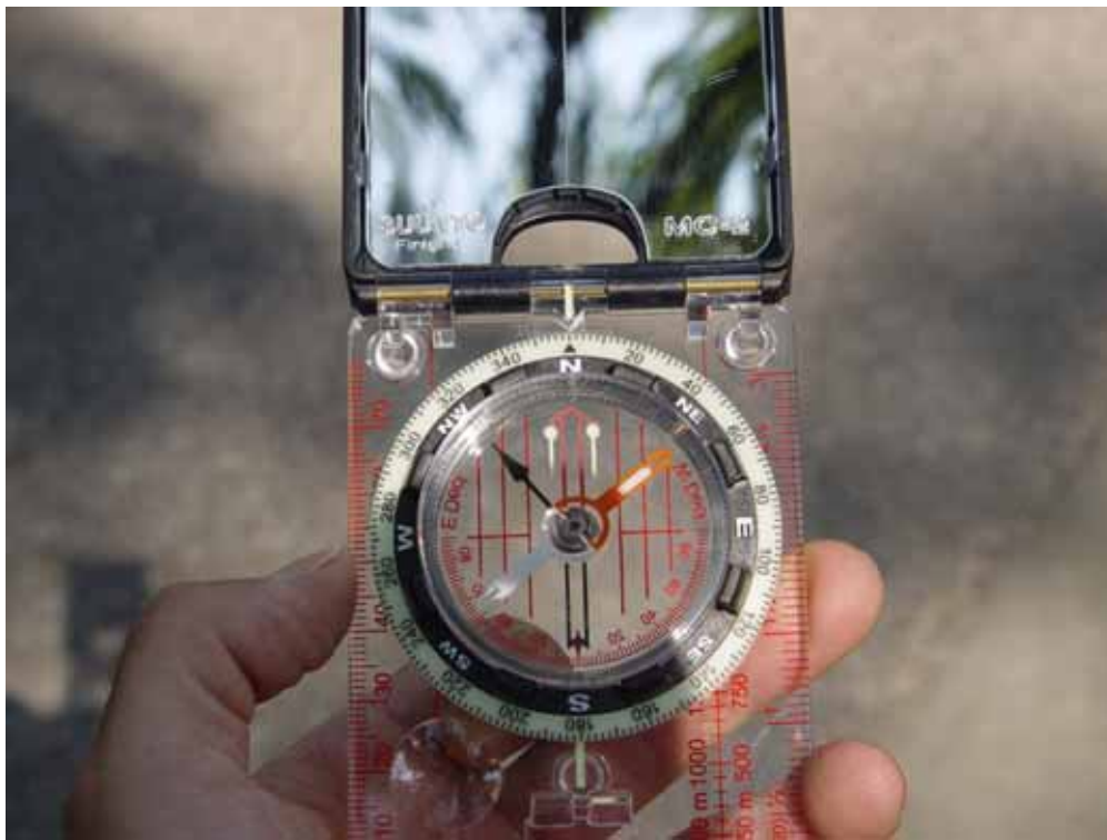
Figure 5.6: Mirror compass utilized for orientation of the weather station
