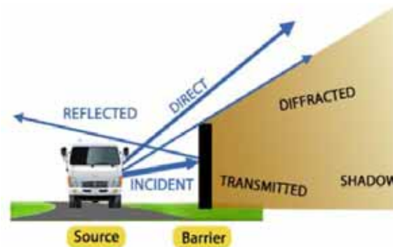
Figure 2.1: Acoustic energy and noise barrier (Bowlby 2012)
