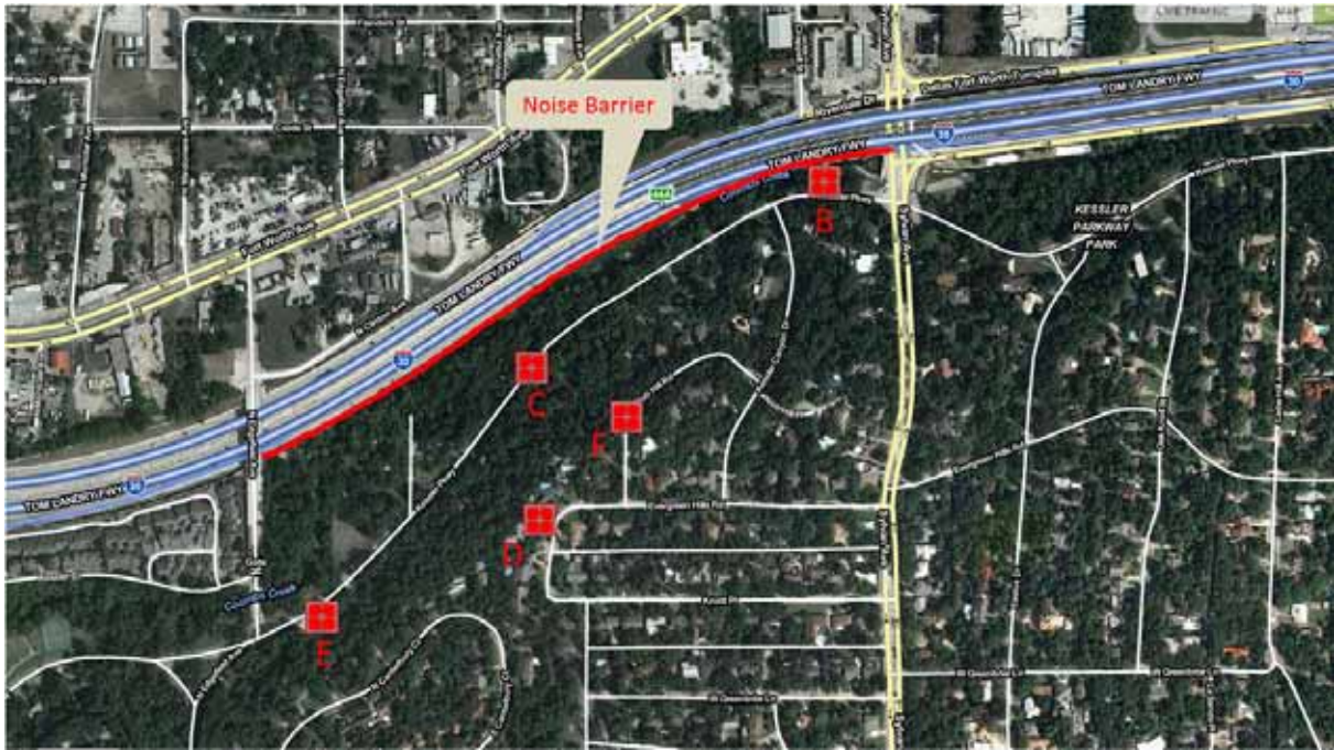
Figure 5.10: Site 1 noise measurement locations
