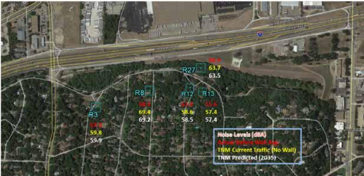
Figure 6.4: Site 2 average noise measurements, before noise wall installation, compared with TNM predictions
