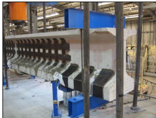
Figure 4-9: Strengthening of the cut end
