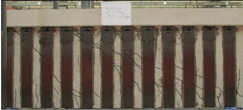
Figure 3-48: Cracking pattern of 48-3-14-3
