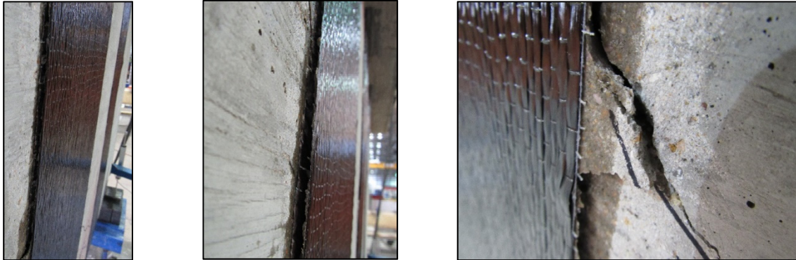
Figure 3-60: Failure of test 48-3-14-8
