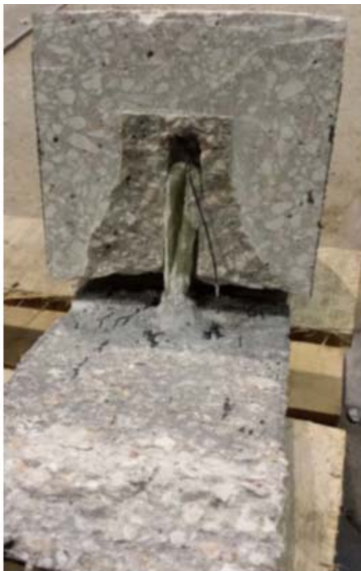
Figure 6-54: GFRP pullout, sectional view
