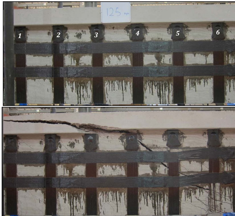
Figure 3-50: Test 48-3-14-4 before (top) and after (bottom) failure
