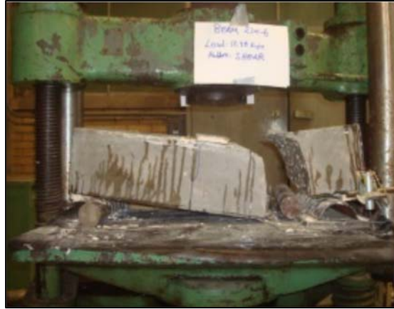
Figure 6-17: Concrete beam shear failure (Huaco, 2009)
