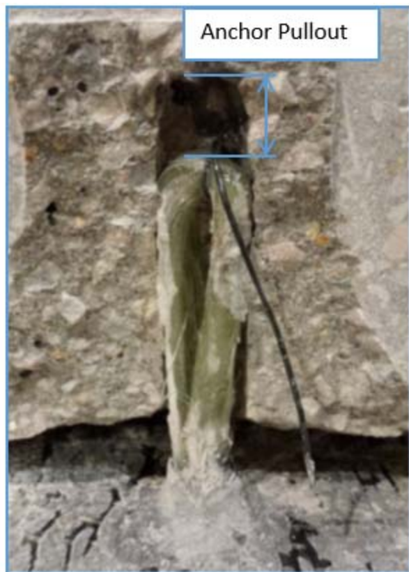
Figure 6-54: GFRP pullout, sectional view
