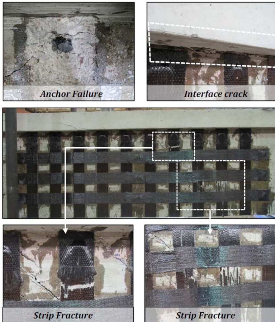
Figure 3-65: Failure of test 48-3-14-10
