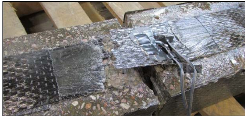
Figure 6-53: CFRP strip fracture
