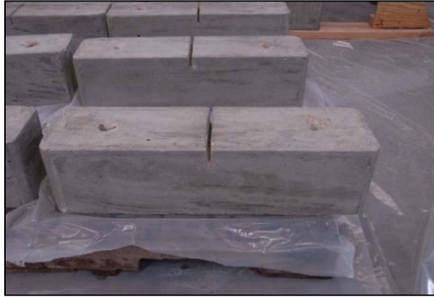
Figure 6-2: Beam specimen before CFRP installation (Series 1 to 3)
