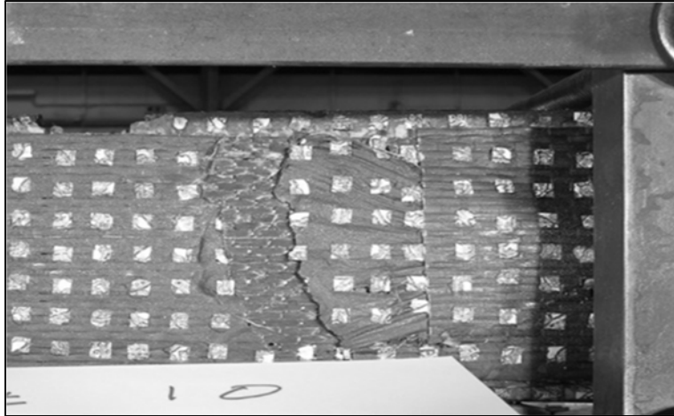
Figure 6-42: Delamination between CFRP strip and anchor
