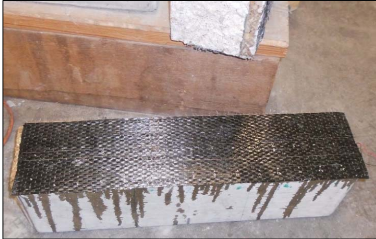
Figure 7-2: Specimen with artificial defects after CFRP installation
