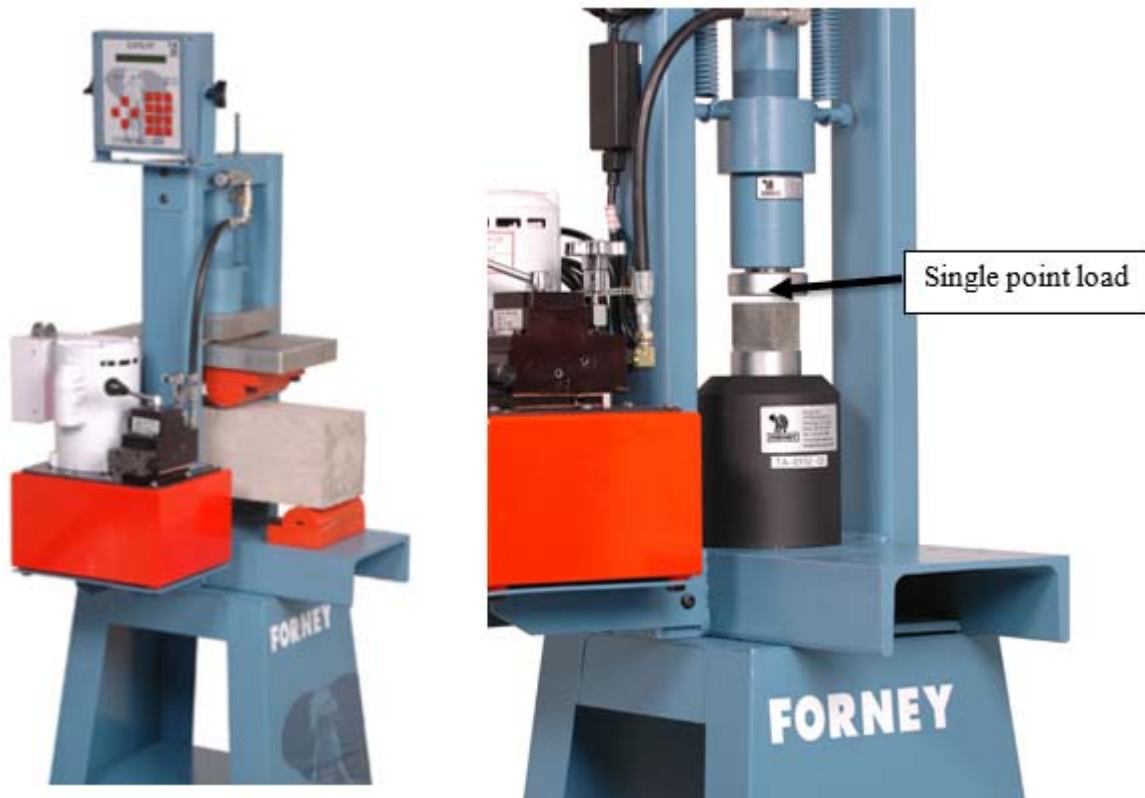
Figure 10-8: Commercial modulus of rupture test setup
