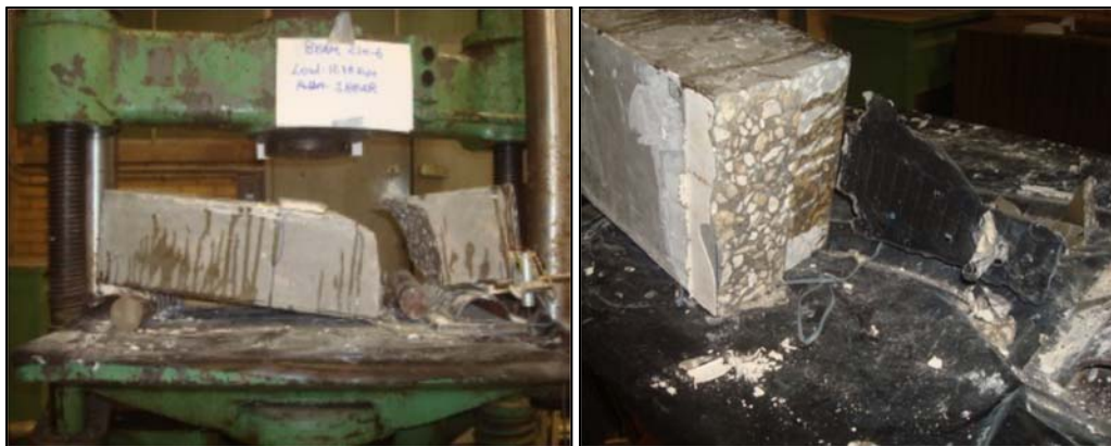
Figure 6-41: Concrete beam shear failure (Huaco, 2010)
