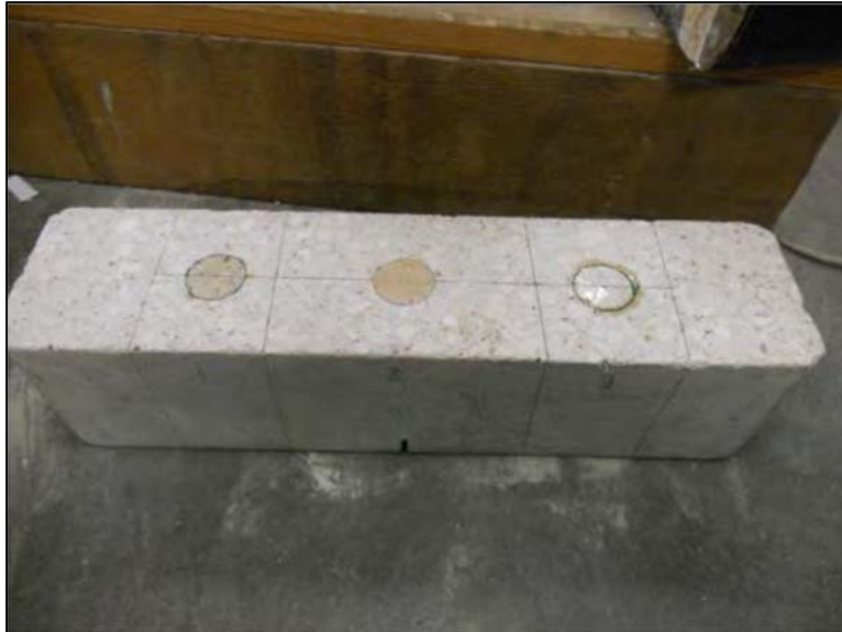
Figure 7-1: Artificial defect fabrication
