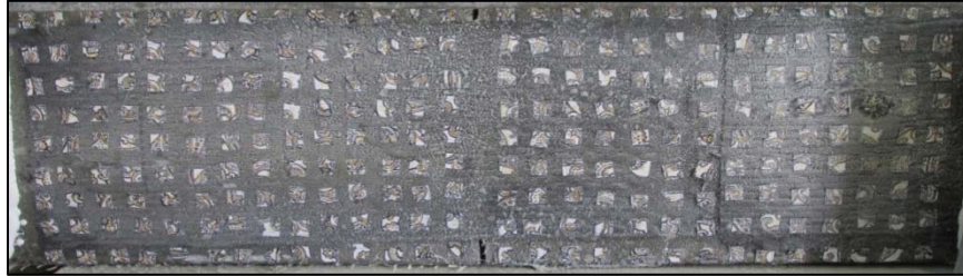
(c) Paper target grid on specimen
