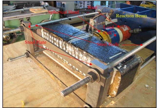
Figure 6-38: Loading and test setup for series 1-3
