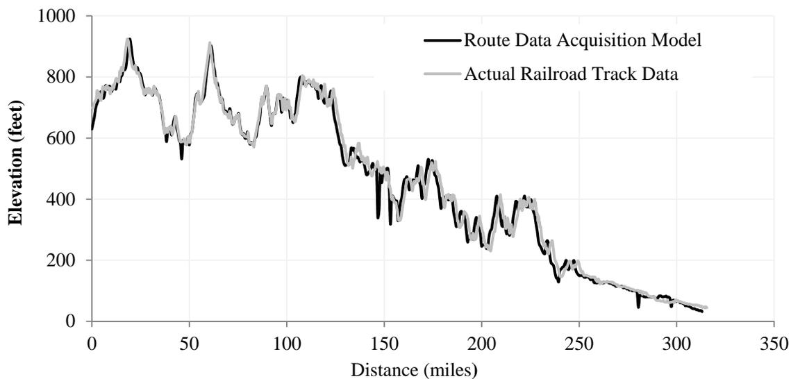
Figure 6.1: Elevation Profiles Comparing the Two Datasets – Model (darker color) and Actual Railroad Track Data (gray color)
