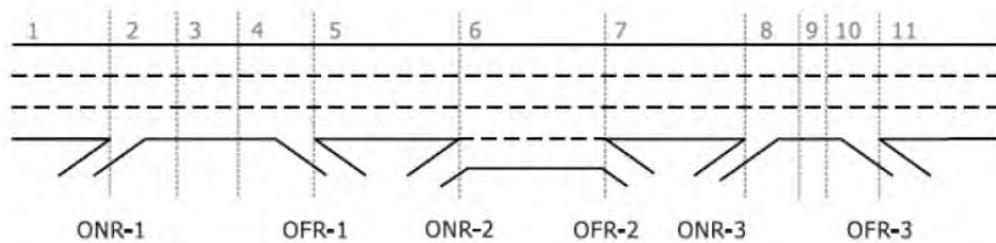
Figure 3.2: Sample Input Data Showing Roadway Geometry (HCM, 2010)
