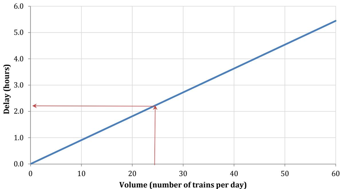
*Figure 7.1: Sample TRIT Output for Relationship between Delay and Volume*
