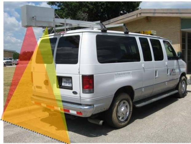
*Figure 1.1: TxDOT’s 3D Automated Measurement System*
