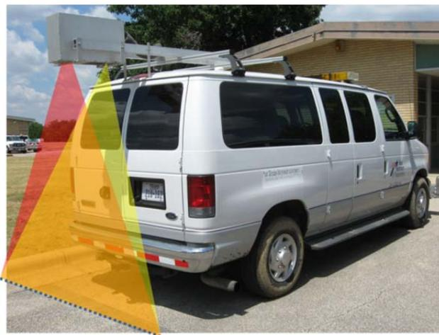
*Figure 1.1: TxDOT’s 3D Automated Measurement System*
