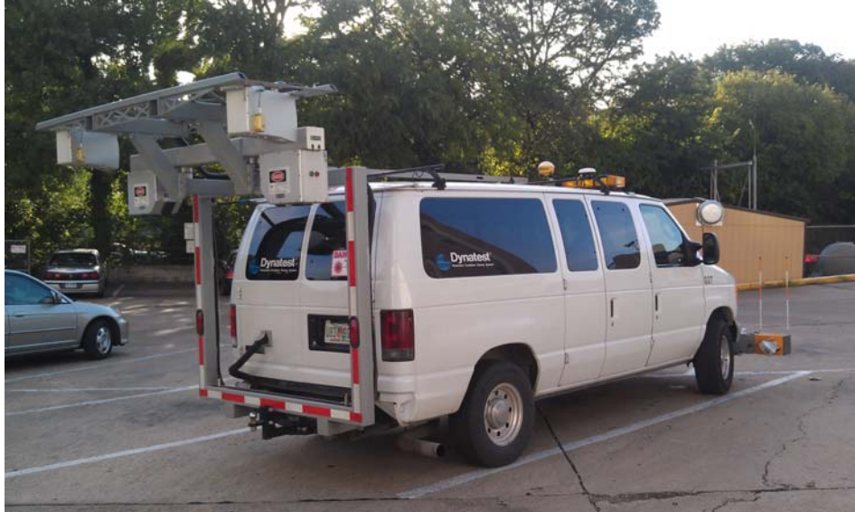
Figure 2.32: Dynatest's Pavement Condition Survey System
