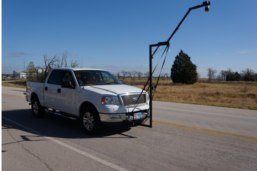
Figure 2.39: Digital Crack Map Data Collection Underway
