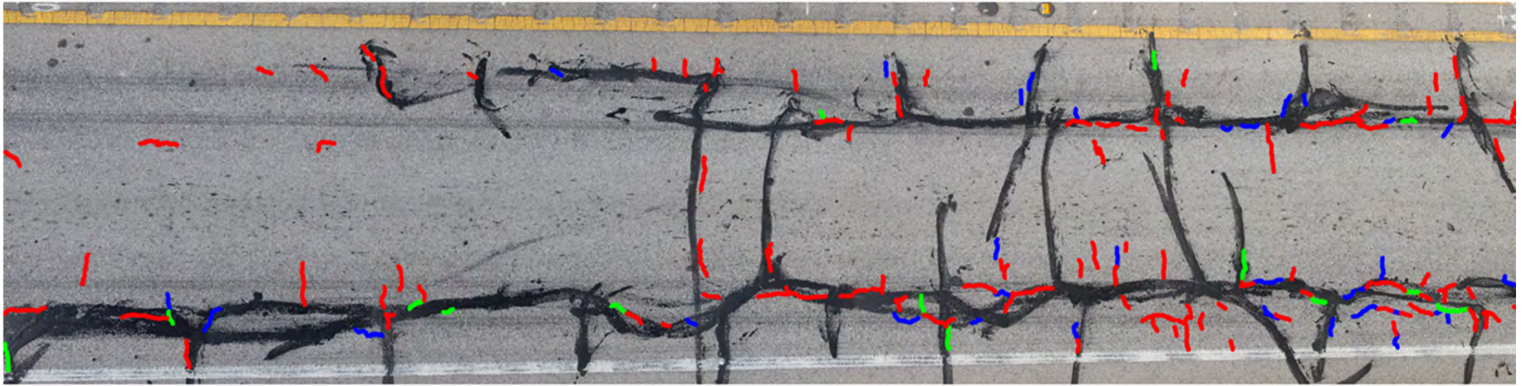
Manual Crack Map
