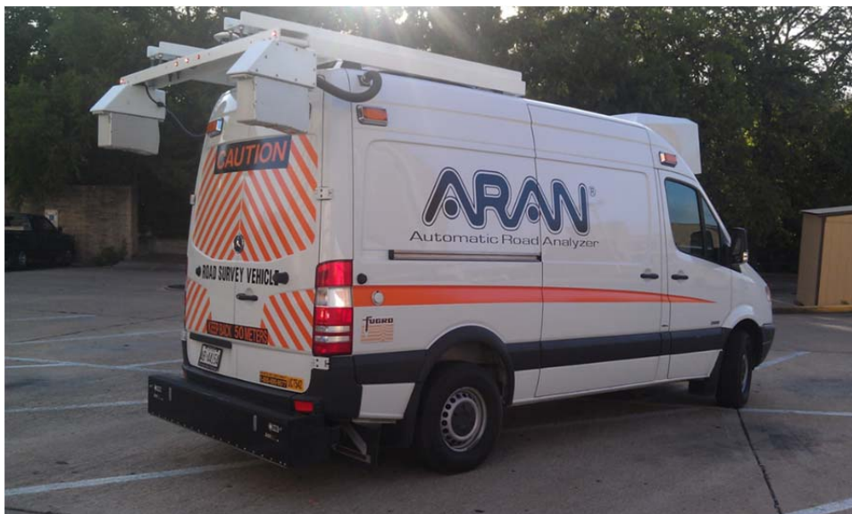
Figure 2.31: Fugro's ARAN 48 with Pave3D System
