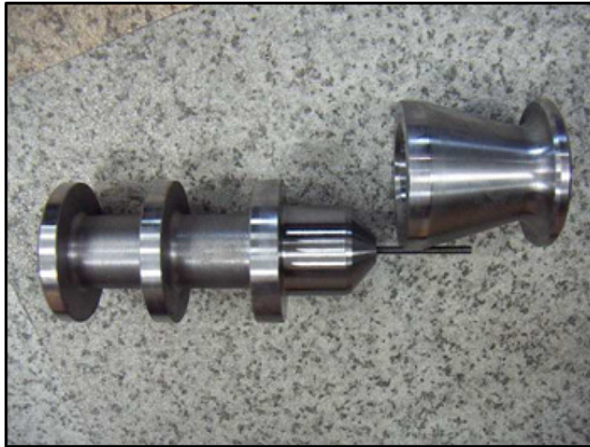
Figure 2.5: Mechanical shear connector used at match-cast joints (from Kim, Chung, and Kim, 2008)
