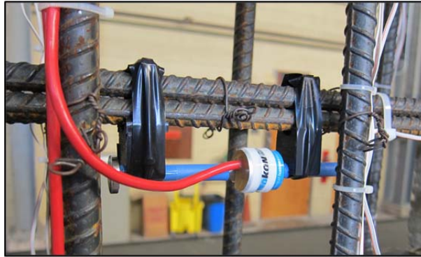
Figure 4.24: Vibrating wire gauge within splice region
