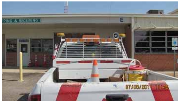
Figure 42: Small Light Bar, Two Rotary Amber Lights, and Arrow Lights
