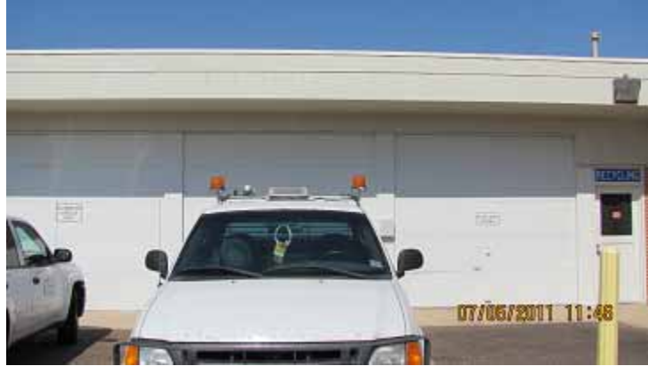
Figure 40: Small Light Bar and Two Rotary Amber Lights
