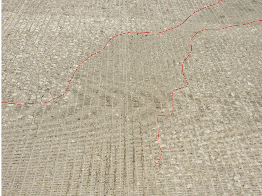
Figure 10.6: Surface Texture Highlighting Exposed Aggregate Regions and Mortar Rich Region
