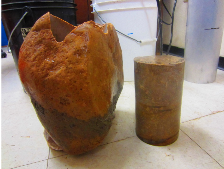
Figure 9.13: Left, Aggregate “Shell” Right, Pure Siliceous Aggregate Core
