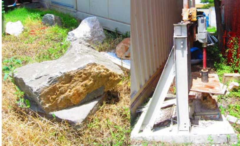
Figure 6.11: Left: Large Aggregate Cast into Support Block for Drilling; Right: Modified Core Drill Rig
