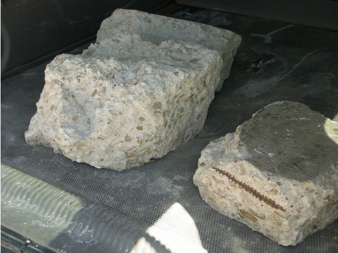
Figure 10.11: Concrete Samples Collected for Determining Mechanical Properties
