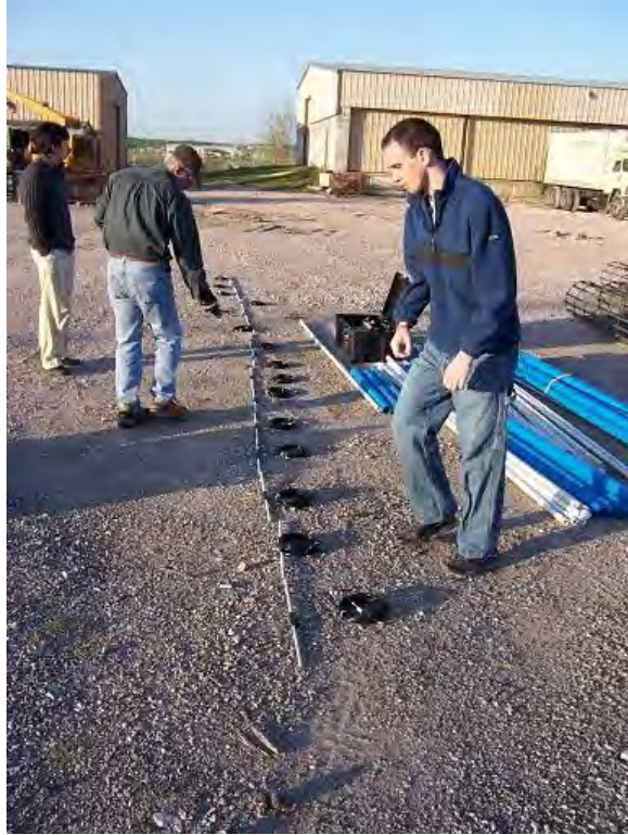
Figure E.12: Laying out the sensors in the correct orientation.
