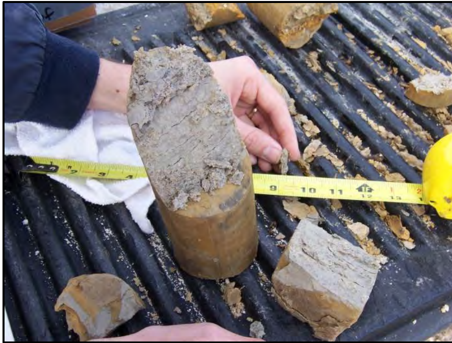
Figure 24. Large Selenite Seam Intersected by B-2 at a Depth of 38 ft
