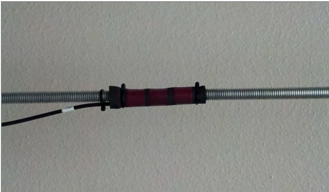
Figure 3.14: Fiber optic strain gauge before installation within the instrumented shaft
