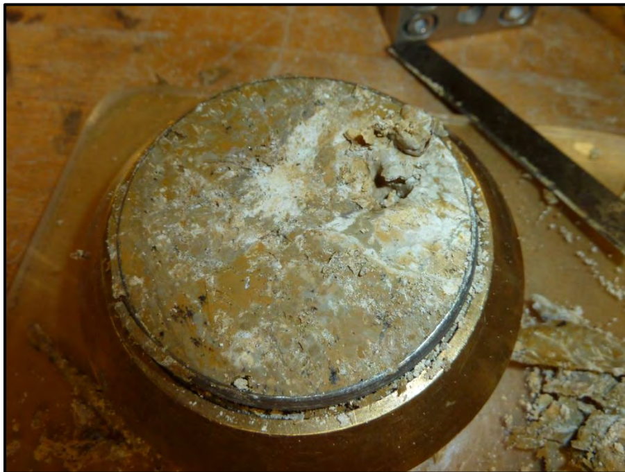
Figure 44. Rock Particle Requiring Removal and Replacement
