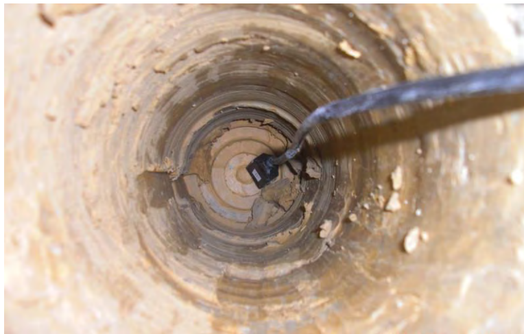
Figure E.30: A sample installation of a probe installed through the facing of the wall.
