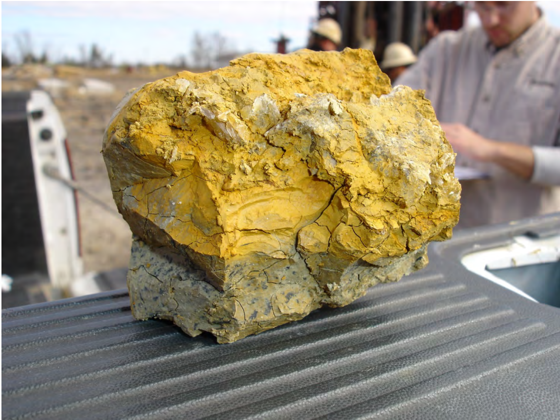
Figure 3.2: A sample of the Taylor Clay at the project site
