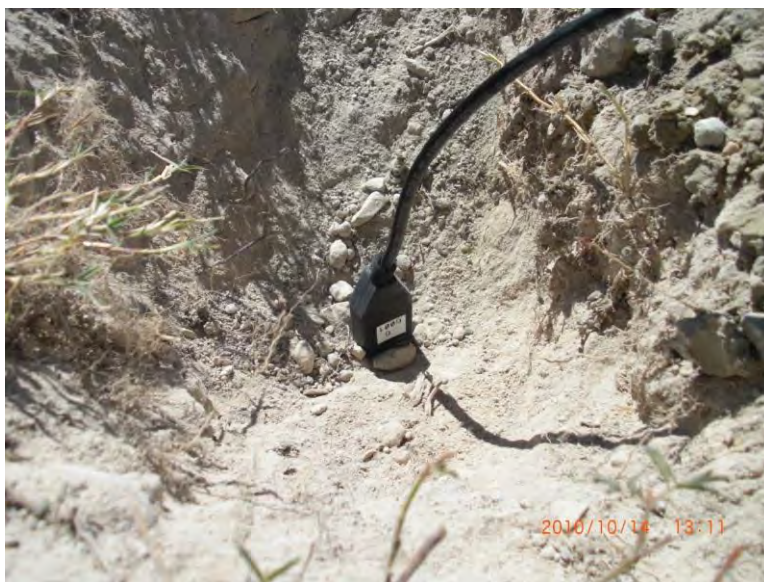
Figure E.32: A sample probe installation from the ground surface.
