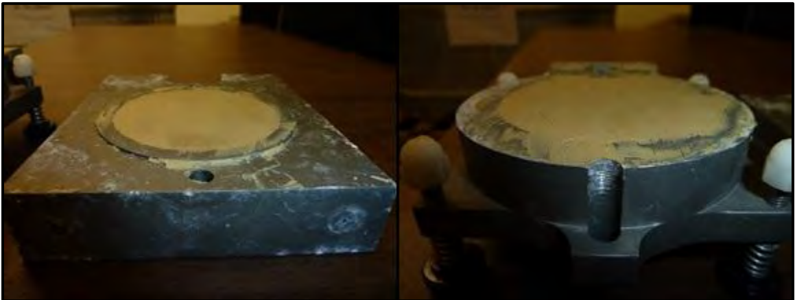
Figure 79. Flattened Shear Surface Smoothed for Residual Shear
